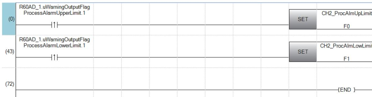
(0) At the time when a process alarm upper limit alert is issued in CH2, the processing is to be performed.
