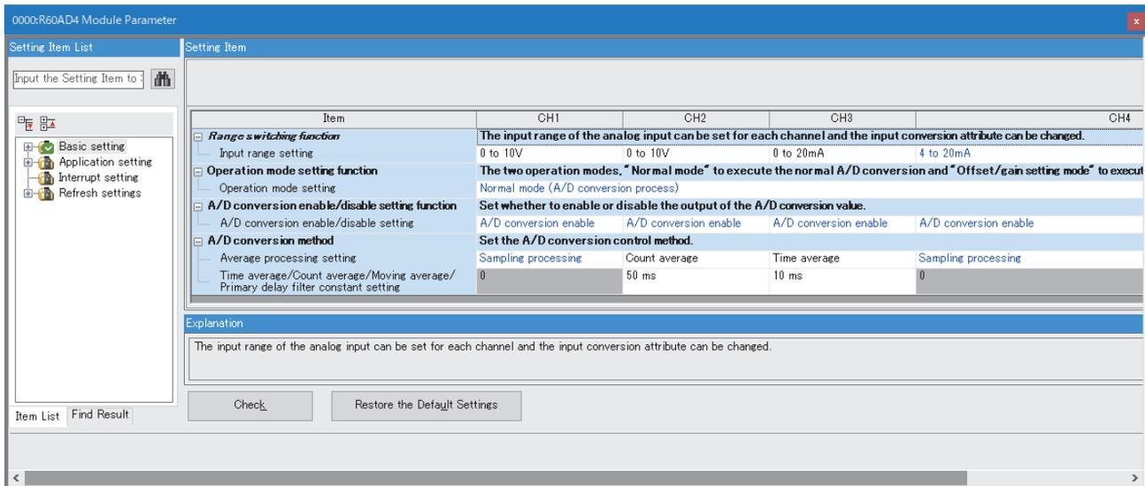
7. Set "Application setting" of "Module Parameter" of the A/D converter module as shown below.
