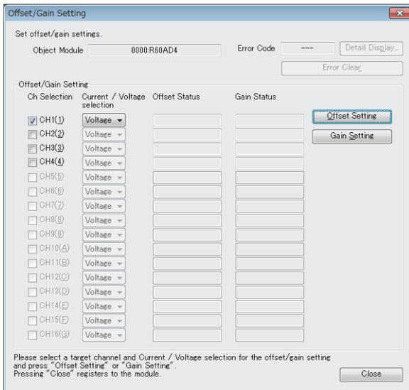
4. Mark the checkbox of the channel where offset and gain values are to be set.
