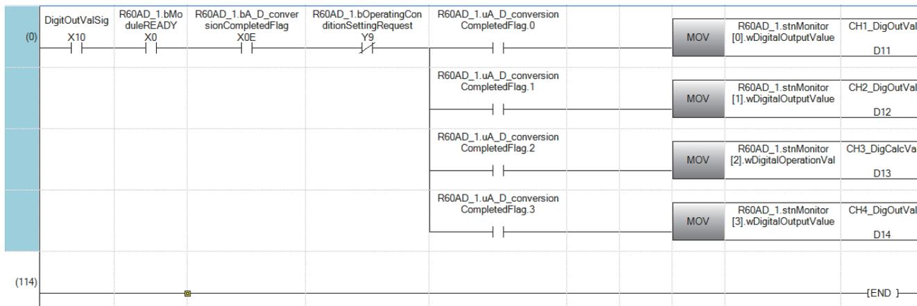
(0) CH1 Digital output value, CH2 Digital output value, CH3 Digital operation value, and CH4 Digital output value are to be read.
