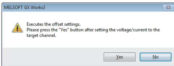
6. Apply the offset voltage or current to the terminal of the corresponding channel, and click [Yes] button.
