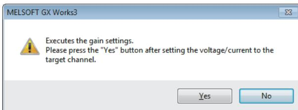
8. Apply the gain voltage or current to the terminal of the corresponding channel, and click [Yes] button.
