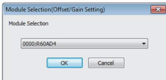
2. Select the target module for the offset/gain setting, and click [OK] button.
