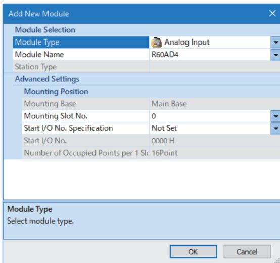
5. Set the window as follows to add the module label of the A/D converter module.
