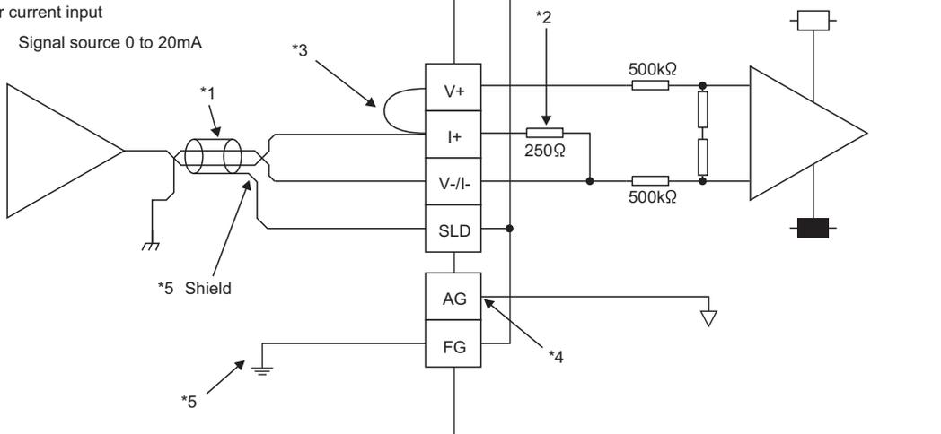
\*1 For the wire, use the 2-core twisted cable.
