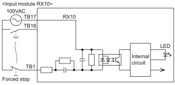
\*: The forced stop input can be set with parameters.
