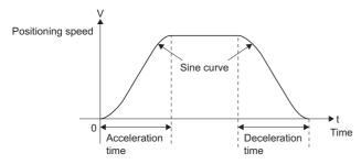
As shown below, the S-curve ratio setting serves to select the part of the sine curve to be used as the acceleration/deceleration curve.
