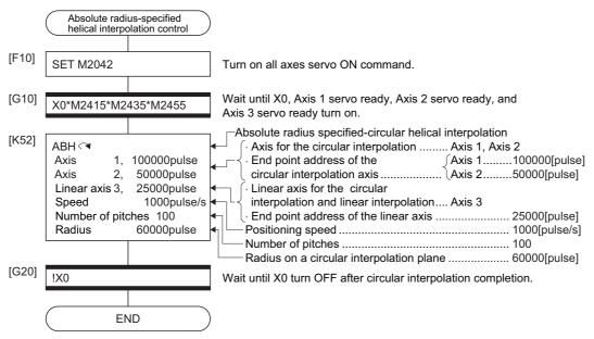
\*1 Example of the above Motion SFC program is started using the automatic start or sequence program.
