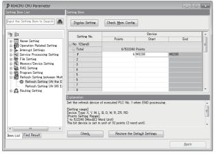
• Set the device received from CPU No.2 (M2400 to M2495)
