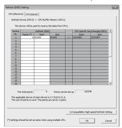
• Set the device transmitted to CPU No.1 (M2400 to M2495, D40 to D59)
