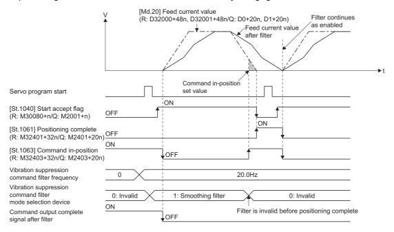
M-code output for continuous trajectory control (CPSTART instruction) is output at the time when the feed current value before filter reaches the specified point. Consequently, due to the delay by the filter, M-code may be updated before the feed current value after filter reaches the specified point.
