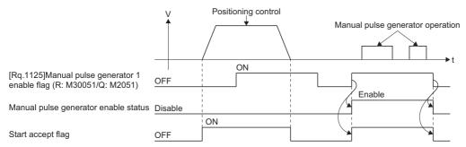
If another axis is set and the same manual pulse generator enable flag turns on again during smoothing deceleration after manual pulse generator enable flag turns off, a minor error (error code: 198EH) occurs, and the manual pulse generator input is not enabled. At this time, include the start accept flag OFF for specified axis as an interlock condition for turning ON the manual pulse generator enable flag.
