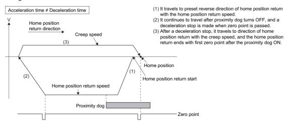
• If the zero point is passed during deceleration, the nearest zero point from deceleration stop position to home position return direction is set as the home position.
