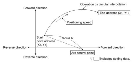
· Positioning control of a complete round is possible in the central point-specified circular interpolation control.
