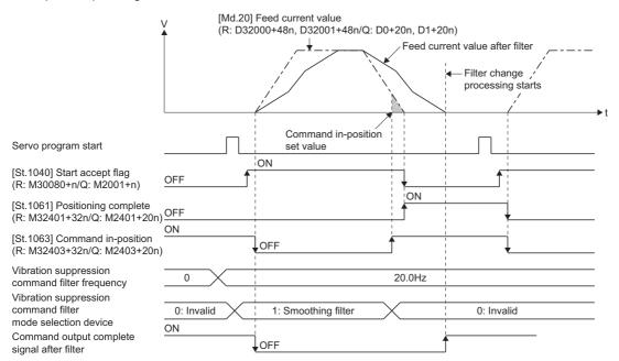
• When a servo program is started up consecutively before the command output complete signal after filter turns ON, filter processing continues and does not become invalid even by changing the mode selection device to "0: Invalid".
