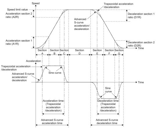
Processing for advanced S-curve acceleration/deceleration is shown below.
