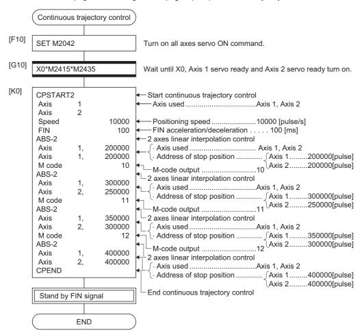
• The Motion SFC program which outputs M-code of each point for continuous trajectory control to Y20 to Y2F by BCD code is shown below.
