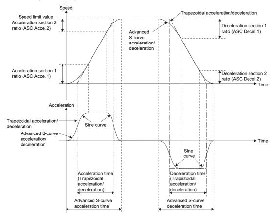
Advanced S-curve acceleration/deceleration can be set by the servo program with the following two methods.
