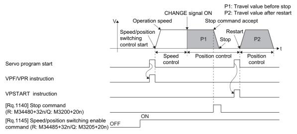
• It controls at the speed stored at the VPF/VPR instruction execution in the re-starting. Therefore, even if the speed change before stop during control, it becomes the speed at the VPF/VPR instruction execution.
