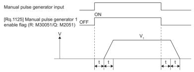
Output speed (V<sub>1</sub>) [pulse/s] = (Number of input pulses/s)  $\times$  (Manual pulse generator 1-pulse input magnification setting) Travel value (L) = (Travel value per pulse)  $\times$  (Number of input pulses)  $\times$  (Manual pulse generator 1-pulse input magnification setting)
