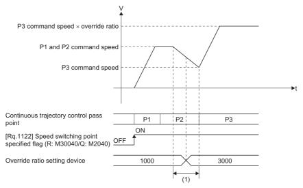
When the override ratio is changed during deceleration of the speed change to P3 (section (1)), the speed is not changed. Speed is changed to the speed of "P3 command speed × override ratio" from the beginning of P3.
