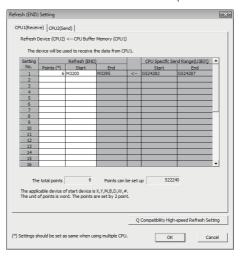
• Set the device transmitted to CPU No.1 (M2400 to M2495)
