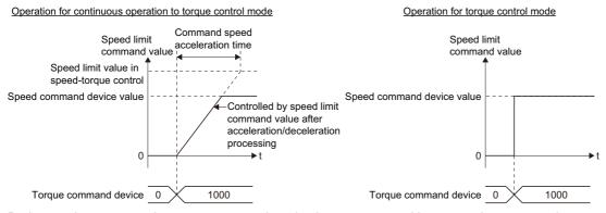
During continuous operation to torque control mode, the torque control is executed at command torque set in "Torque command device". Command torque can be changed any time during continuous operation to torque control mode. Speed change request (CHGV, M(P).CHGV/D(P).CHGV) is invalid (no operation).
