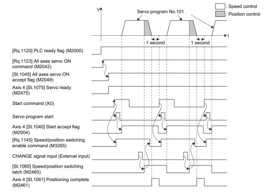
The Motion SFC program for executing the servo program (No. 101) for speed-position switching control is shown below.
