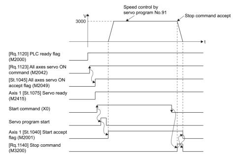
The Motion SFC program for executing the servo program (No. 91) for speed control (I) is shown below.
