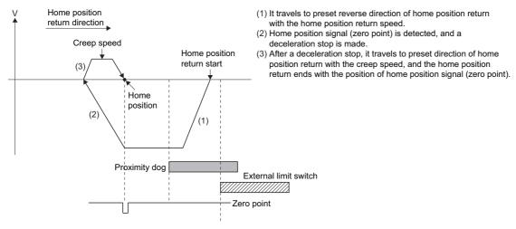
• If the zero point is passed during deceleration, the nearest position of home position signal (zero point) of home position return direction from deceleration stop position is set as the home position.
