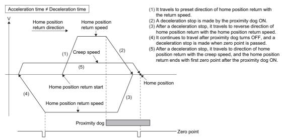
When it starts in the proximity dog, the zero point is not passed ("[St.1066] Zero pass (R: M32406+32n/Q: M2406+20n)"
