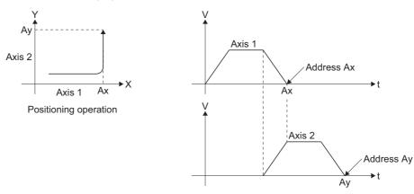
Continuous-trajectory control processing of each axis
