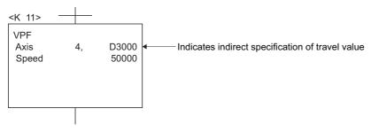
• The travel value is stored in the data register for travel value change during speed control in the Motion SFC program.
