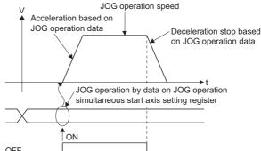
[Cd.1096] JOG operation simultaneous start axis setting register (forward JOG) (R: D35286 to D35289/Q: D710, D711)/
