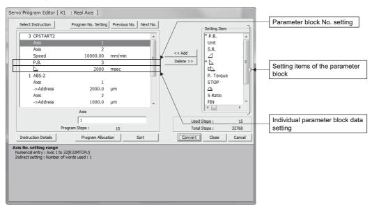
Unit : Interpolation control unit S.R. : Speed limit value  $\triangle$ : Acceleration time : Deceleration time P. Torque EΔ : Acceleration time : Torque limit value STOP : Deceleration processing on STOP input : Allowable error range for circular S Ratio : S-curve ratio when S-pattern processing interpolation is executed
