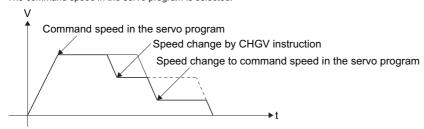
(2) Change speed by CHGV instruction < command speed in the servo program The change speed by CHGV instructions is effective.
