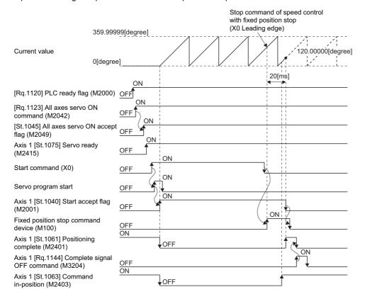
The Motion SFC program for executing the servo program (No. 55) for speed control with fixed position stop is shown below.
