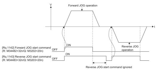
• If the JOG start command ("[Rq.1142] Forward JOG start command (R: M34482+32n/Q: M3202+20n)" / "[Rq.1143] Reverse JOG start command (R: M34483+32n/Q: M3203+20n)") turns on during deceleration by the JOG start command OFF, after deceleration stop, JOG operation is not executed. After that, the JOG operation is executed by the JOG start command OFF to ON.
