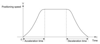
S-curve ratio set the part of the sine curve used to produce the acceleration and deceleration curve as shown in the diagram below.
