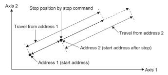
When the address 2 is moved to the same address (address which calculates with start address + specified travel value) using the INC $\square$ , the following processing using the servo program and Motion SFC program is required.
