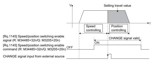
• If the stop occurred during position control, re-start with position, and the positioning control of setting travel value. The travel value after the re-start is calculated as follows:
