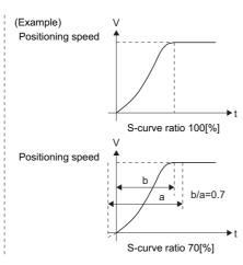
S-curve ratio can be set by the servo program with the following two methods.
