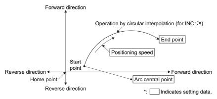
· Positioning control of a complete round is possible in the central point-specified circular interpolation control.
