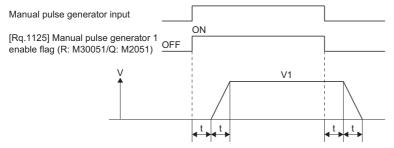
Output speed (V1) = [Number of input pulses/ms] × [Manual pulse generator 1-pulse input magnification setting]
