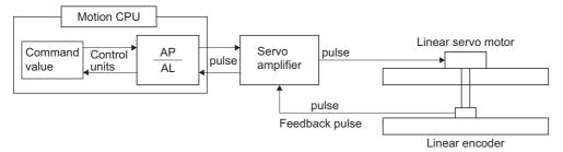
Calculate the number of pulses (AP) and travel value (AL) for the linear encoder in the following conditions.
