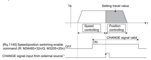
\*1 The CHANGE input signal from external source uses the input set for the DOG signal in the external signal parameter. When "normally open contact input" is set, CHANGE input occurs at the CHANGE signal on, and when "normally closed contact input" is set, CHANGE input occurs at the CHANGE signal off. (Fig. Page 193 External Signal Parameter)
