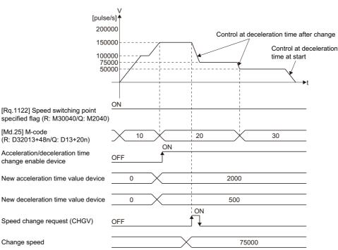
• For control with changed acceleration/deceleration time, even if acceleration/deceleration time change enable device is turned OFF (invalid), control at acceleration/deceleration time after change continues until the operation ends.
