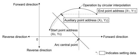
• The setting range of the end point address and auxiliary point address is  $(-2^{31})$  to  $(2^{31}-1)$ .
