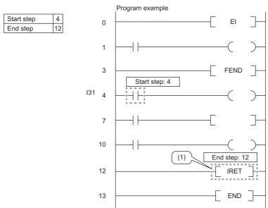
(1) When the scan time in an interrupt program is measured, do not specify the IRET instruction for the end step.
