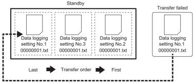
The retry ends when the network is recovered and retry of the file transfer succeeds.
