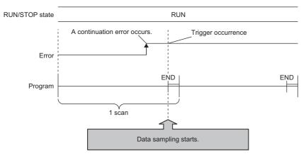
In the following situations, the occurrence of a continuation error that is specified as a trigger condition is not recognized as a trigger, with no data collection:
