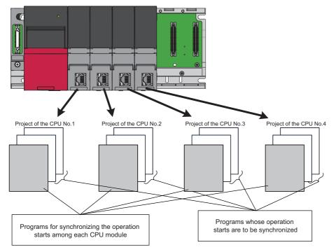
The following is an example of the configuration of a program which synchronizes the start of operation processing across CPU modules and programs which should start operation processing synchronously.
