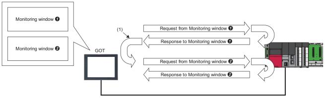
(1) From the time the CPU module sends a response until the GOT sends the next request, the CPU module will not receive requests from the GOT.
