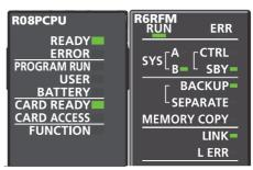
When an error has occurred, the following LEDs are on. Check details of the error with the engineering tool and eliminate the error cause.
