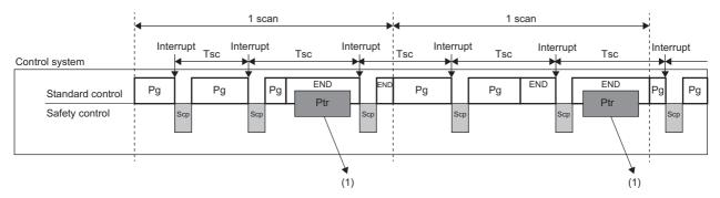
Tsc: Safety cycle time Pg: Standard program Scp: Safety cycle processing Ptr: Tracking
