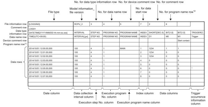
\*2 These items are displayed when a local device/local label is specified. The items are not output when a global device/global label is specified. (The corresponding columns and rows become blank.)
