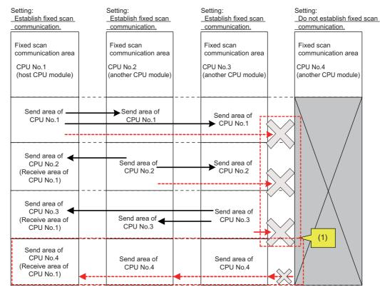
(1) Since the setting does not allow fixed scan communication, this CPU module does not send data to the other CPU modules although send areas have been reserved. This CPU module does not receive data from the other CPU modules.
