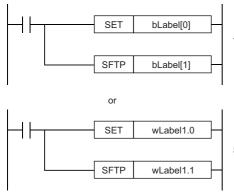
To shift the bits correctly, specify the array of the bit type label.
