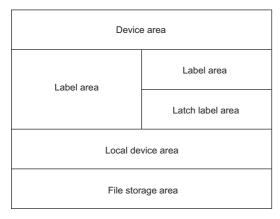
The capacity of each area can be changed with the setting of the CPU parameter. ( Page 103 Device/label memory area setting)
