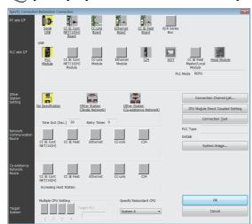
Connection Destination Connection" window. 2. Click the [Connection Test] button to check whether the CPU
