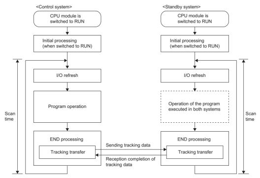
Both systems perform different processing depending on the set operation mode.
