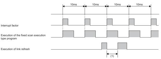
(1) The link refresh is suspended and the fixed scan execution type program is executed.
