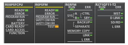
\*1 In a redundant master station system, the MST LED of the master/local module in the standby system flashes.
