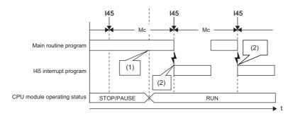
Mc: Multiple CPU synchronization cycle
