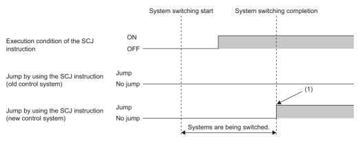
(1) After system switching, the processing jumps in the first and later scans
