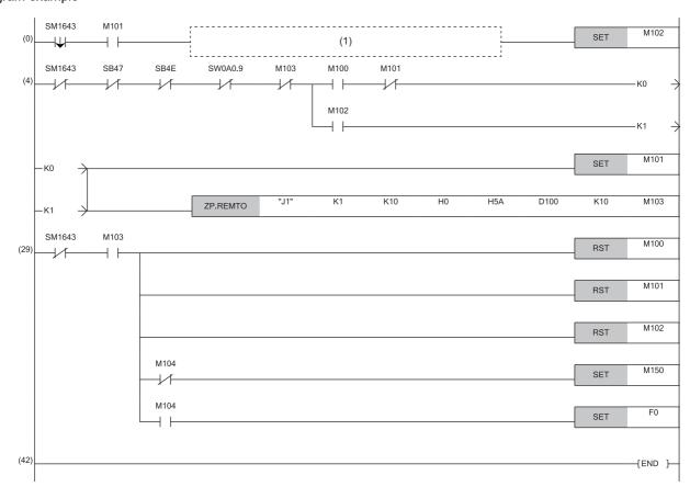
(1) Add an interlock circuit for determining whether or not to execute the instruction again (according to the X signals and buffer memory status of the target module) as required.
