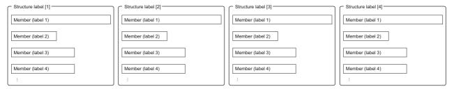
When a structure is declared as an array, add an index enclosed by '[]' after the structure label name.
