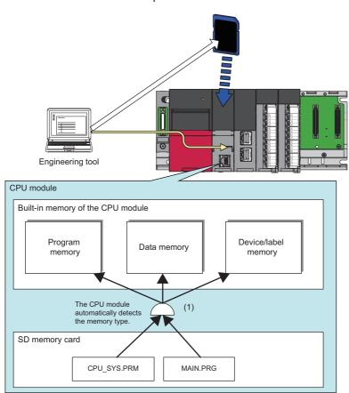
(1) The boot operation is executed according to the boot file setting when the CPU module is powered on or is reset.
