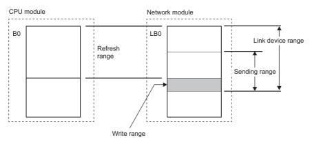
\*1 There is only one network module to which the link direct device can write data for each network number. When more than one network module with the same network number is mounted, the network module with the lowest slot number is the target for writing by the link direct device
