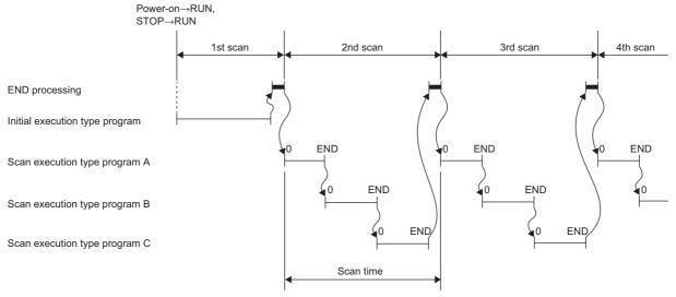
When multiple scan execution type programs are executed, the execution time of the scan execution type program will be the total time until all the scan execution type programs finish execution. Note that if interrupt program, fixed scan execution type program, and/or event execution type program are executed before the scan execution type program finishes execution, the execution time for these programs is also included.
