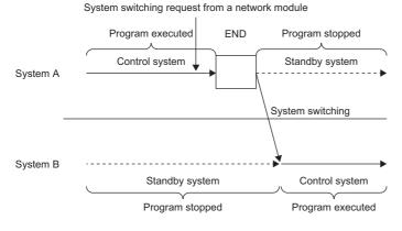
The following network modules send a system switching request.
