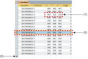
**5.** When the value is changed or the record is deleted, the database of the CPU module is changed according to the operation.
