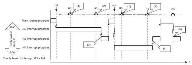
Mc: Multiple CPU synchronization cycle
