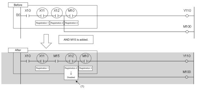
(1) The registration of the device test with execution conditions of the instruction immediately after the instruction to be added is disabled.
