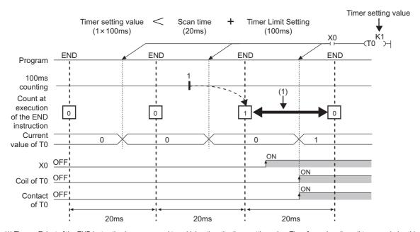
(1) The coefficient of the END instruction becomes equal to or higher than the timer setting value. Therefore, when the coil turns on during this period, the contact also turns on at the same time.
