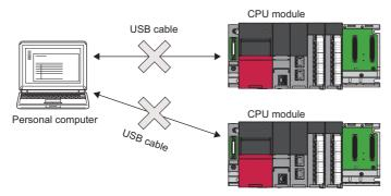
• Connecting to more than one CPU module via a USB hub
