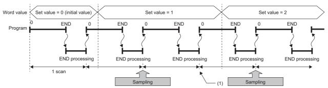
(1) The data logging function does not collect data because there has been no change in state since the last scan.
