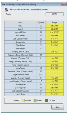
1. On the "Valid Range Confirmation of Latch Interval Setting" window, check the effective range for the latch timing setting. Specify the latch interval operation within the effective range.
