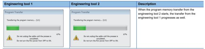
If the later program memory transfer (from the engineering tool 2) has completed with an error, the former program memory transfer (from the engineering tool 1) does not complete. In such a case, write the data again instead of powering off and on or resetting the CPU module.
