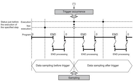
The state changes from non-running to running immediately before the execution of the specified step.
