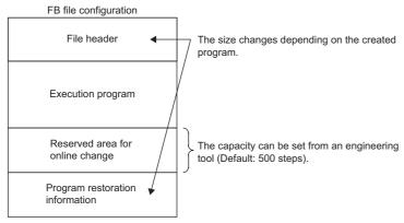
When an FB file is stored in the CPU module, the file header, execution program, and reserved area for online change are allocated to the program memory. Program restoration information is allocated to the data memory. The destination memory to which each area is allocated when an FB file is stored in the CPU module is the same as that for programs.
