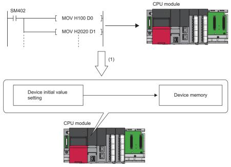
(1) If initial device values are used, a program to set data to the devices becomes unnecessary.
