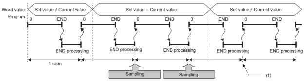
(1) During the END processing, the data logging function does not collect data because the conditions are not met.
