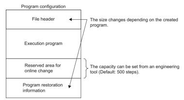
When the program is stored in the CPU module, file header, execution program, and reserved area for online change are allocated to the program memory. Program restoration information is allocated to the data memory. The following table shows the destination memory to which each area is allocated when a program is stored in the CPU module.
