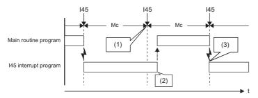
Mc: Multiple CPU synchronization cycle
