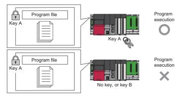
If the security key of only one program does not match the security key of the CPU module, all the other programs in the CPU module are not executed as well.
