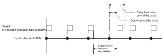
The delay limit value behind a cycle differs as follows.
