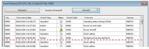
Since the time goes back one hour at No.00005 where the daylight saving time ends, the dates and times on which events occurred are reversed at the upper and lower side of the broken line ((time of new event history) < (time of old event history)).
