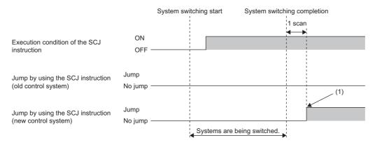
(1) After system switching, the processing jumps in the second and later scans.
