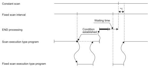
\*1 If processing does not finish during the waiting time, the scan time is extended.
