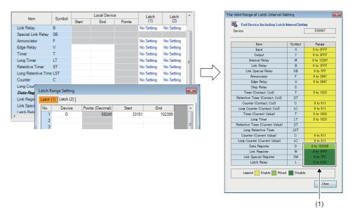
(1) D30848 or later areas of the data register (D) and areas of the devices (W, SW, and L) in disabled ranges can be latched in real time.
