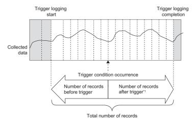
\*1 This number includes the record exactly at the time when the trigger condition is met.
