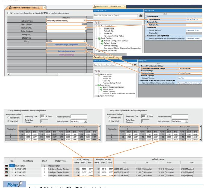
Assign B (bit device) to RWw/RWr (word device).
