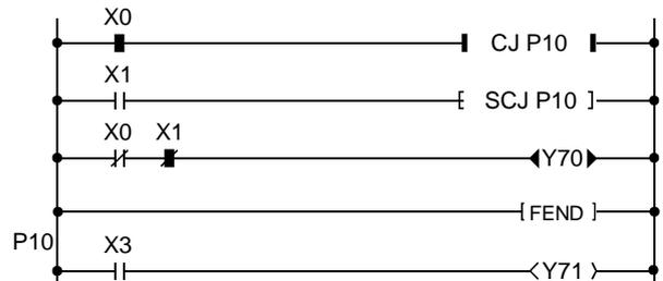
(3) Turning off X0 and on X1 executes the SCJ instruction and jumps the program to P10 from the second scan. Therefore, Y70 turns off.
