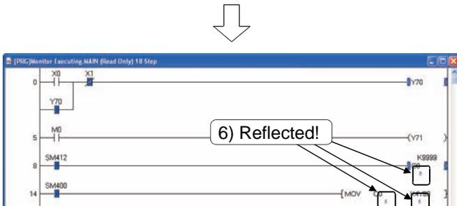
6) The change of the value of "C0" to "5" is reflected on the ladder monitor screen.
