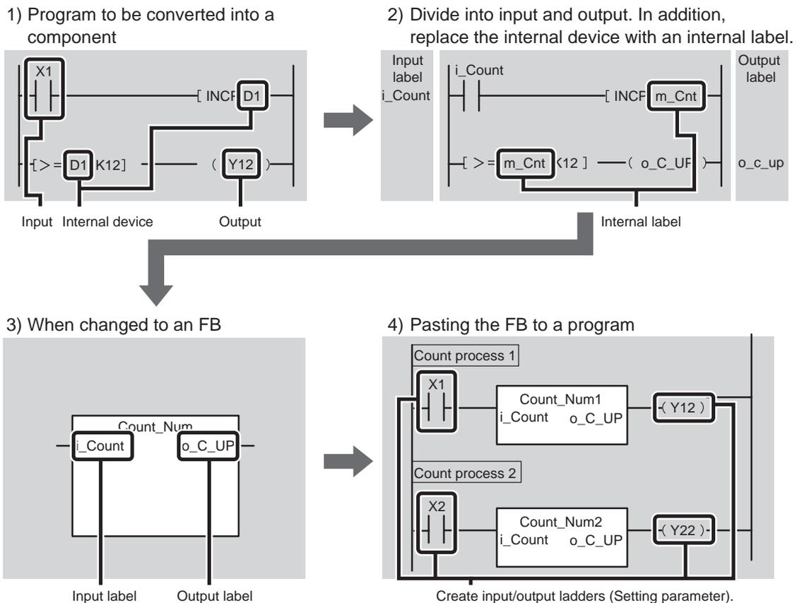
Figure App. 9.2 Flow of conversion into components
