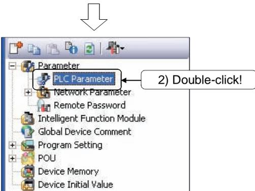
2) "PLC Parameter", the "Network Parameter" folder, and "Remote Password" are displayed. Double-click the "PLC Parameter".
