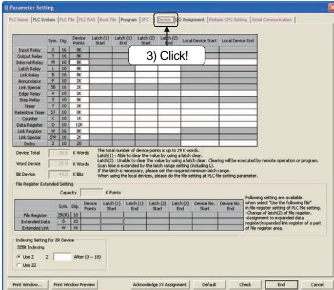
3) The Q Parameter Setting dialog box is displayed. Click the "Device" tab.
