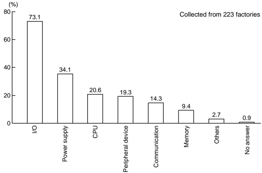
Figure 9.2 Causes of programmable controller faults (multiple answers allowed)
