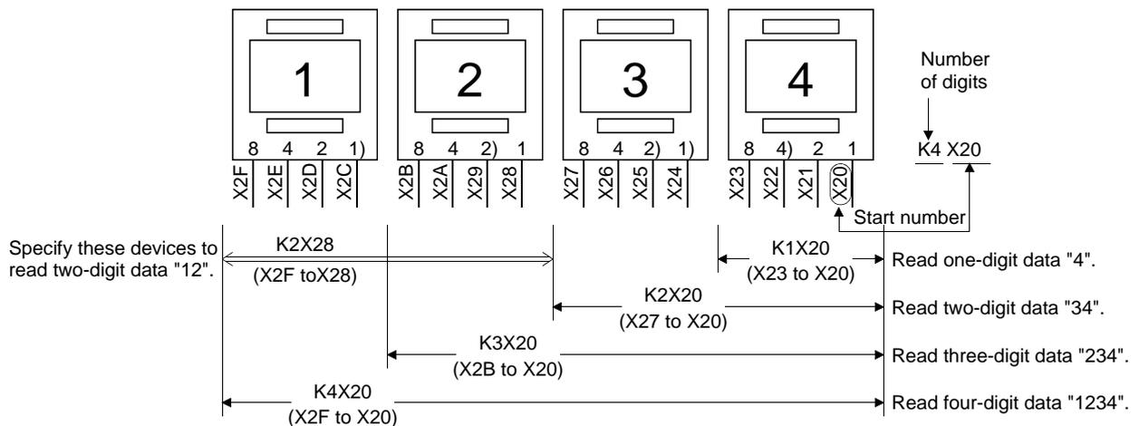
As long as four bit devices are in consecutive order, any bit device can be specified as the first.
