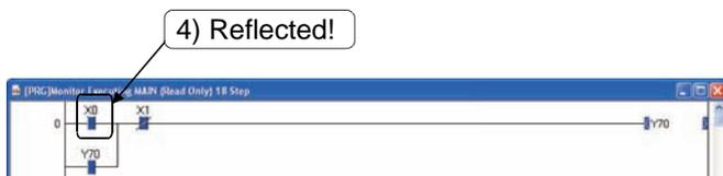
4) The result of the device being turned on is reflected on the ladder monitor screen.
