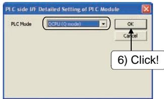
6) The PLC side I/F Detailed Setting of PLC Module dialog box is displayed. Select "QCPU (Q mode)" and click the **OK** button.
