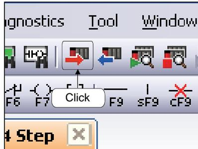
(b) Click the **Parameter + Program** button. Checkboxes for the target program and the target parameter displayed in the window are automatically marked (✓).
