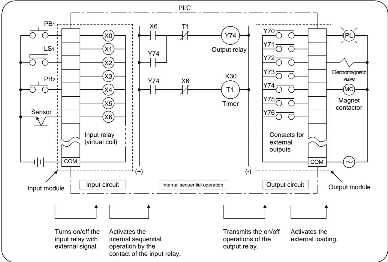
Figure 1.1 Programmable controller configuration
