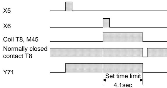
(Note) The above ladder operates as an off delay ladder by momentarily turning on inputs X5 and X6.
