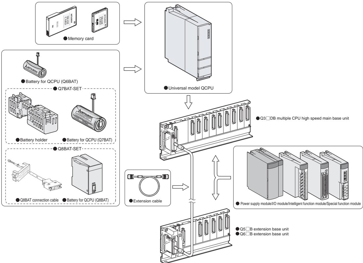
Figure 1.3 MELSEC-QnUD module configuration (when Q3□DB is used)
