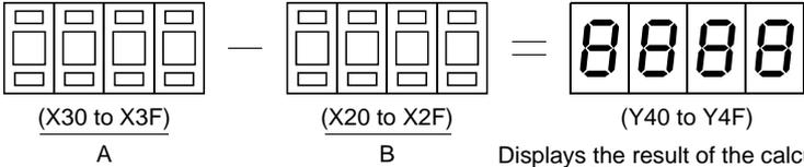
Displays the result of the calculation of A - B on the BCD display of Y40 to Y4F. When the result is a negative number, make sure that the display displays 0 and the LED of Y70 turns on.
