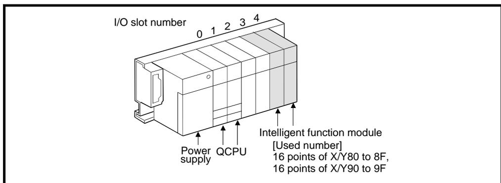
Figure 7.1 Installation of intelligent function module
