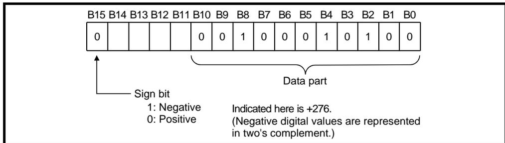
Figure 7.6 Example image of buffer memory content (D/A converter module)
