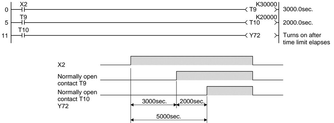
(2) Necessary time is obtained by using timers and counters.
