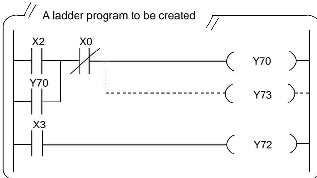
This section explains how to add a line to the ladder program shown on the left.
