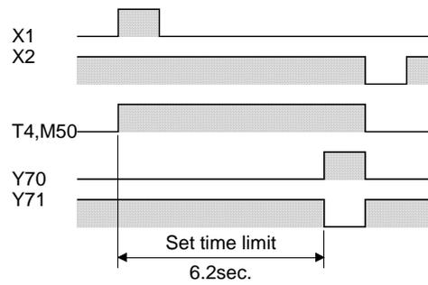
(Note) The above ladder operates as an on delay ladder by momentarily turning on inputs X1 and X2.
