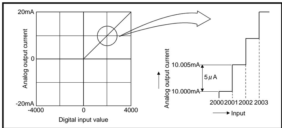
Figure 7.15 D/A conversion characteristics (current output)
