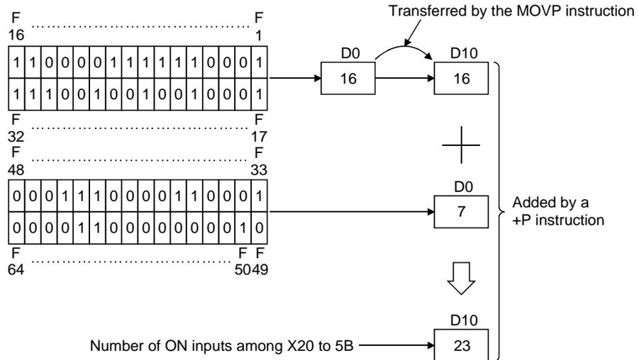
(2) Searching for ON devices shifting 32-bit data to right
