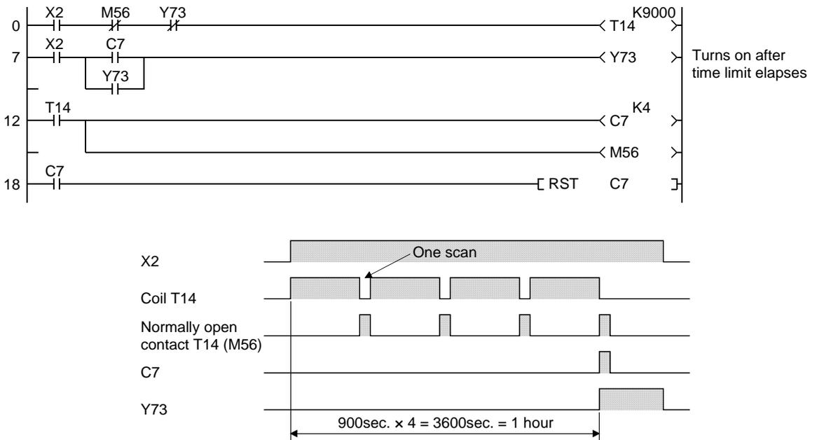
(Note) Sufficient time is obtained with the counter C7 which counts the number of time-outs of the timer T14.
