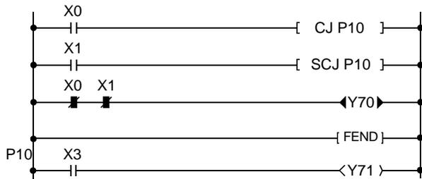
(2) When X0 is turned on, the CJ instruction is executed and the program jumps to P10. Therefore, Y70 remains on.
