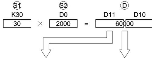
To store the result of 16-bit data × 16-bit data, 16 bits (1 word) is not enough. Therefore, D10 which is specified in the program and the next number D11 work as the holder of the result.
