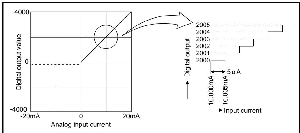
Figure 7.13 A/D conversion characteristics (current input)
