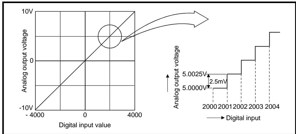
Figure 7.14 D/A conversion characteristics (current output)
