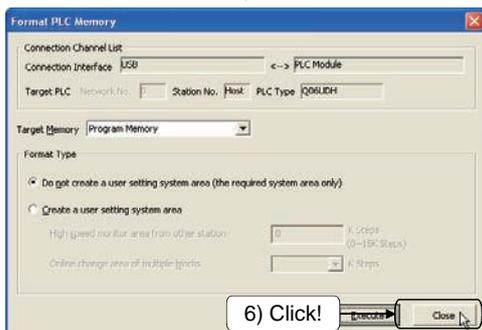
(6) Clearing all the device memory from the CPU
