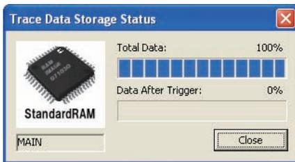
3) The Trace Data Storage Status screen is displayed when the sampling trace is started.
