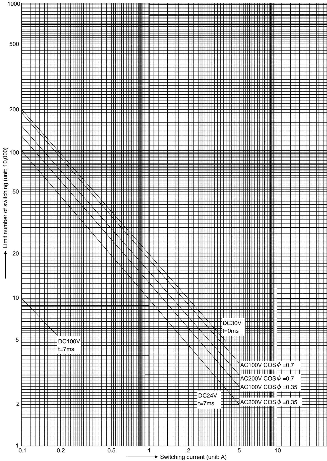
Figure 9.3 Life characteristics of output relay's contact (QY10, QY18A)
