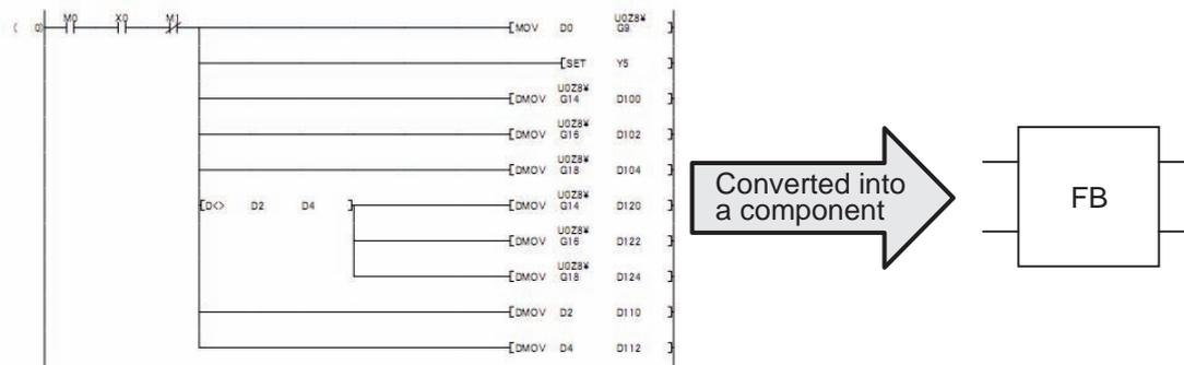
Figure App. 9.1 Converting a sequence program into a component
