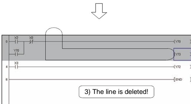
3) The line is deleted when the left button of the mouse is released.
