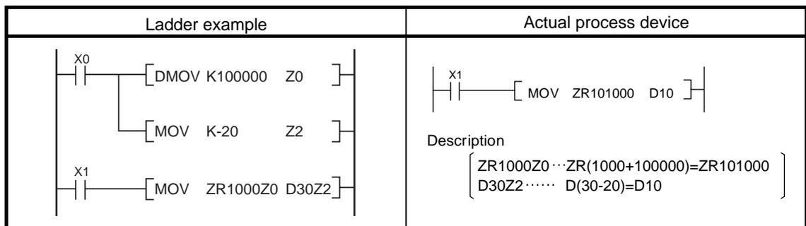
(2) When specifying the 32-bit indexing using "ZZ" specification
