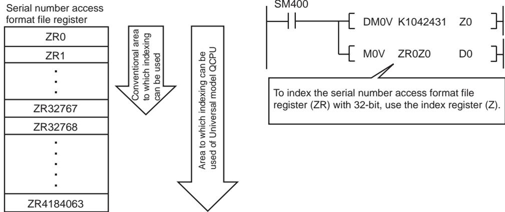
A method for specifying index registers for 32-bit indexing can be selected from following two methods.
