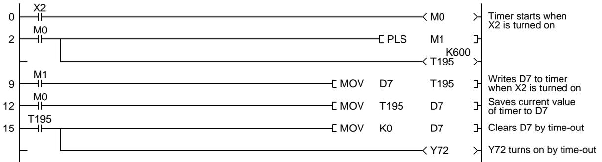
(2) When retentive timers are assigned in the device setting of the PLC parameter Retentive timer (ST): 224 points (ST0 to ST223)
