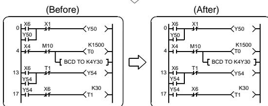
4) Confirm that the normally open contact is changed to the normally closed contact and vice versa.
