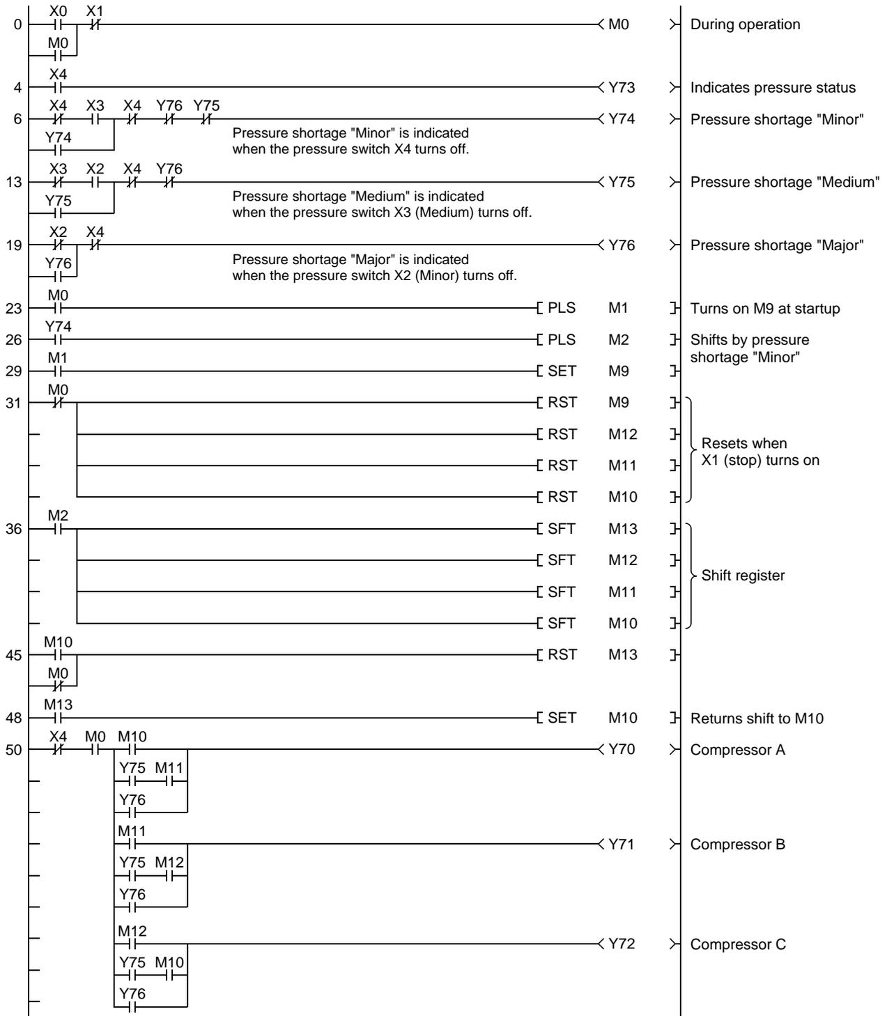
After the basic operation, one compressor is activated in reaction to pressure shortage detected. To use the three compressors equally, they are activated according to the set order. This control is enabled by the 3-stage ring counter (ring-shaped shift registers) M10 to M12.
