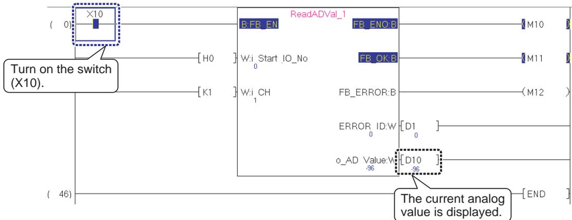
Double-clicking the FB in the sequence program on the screen enables monitoring of the sequence program status in the FB.
