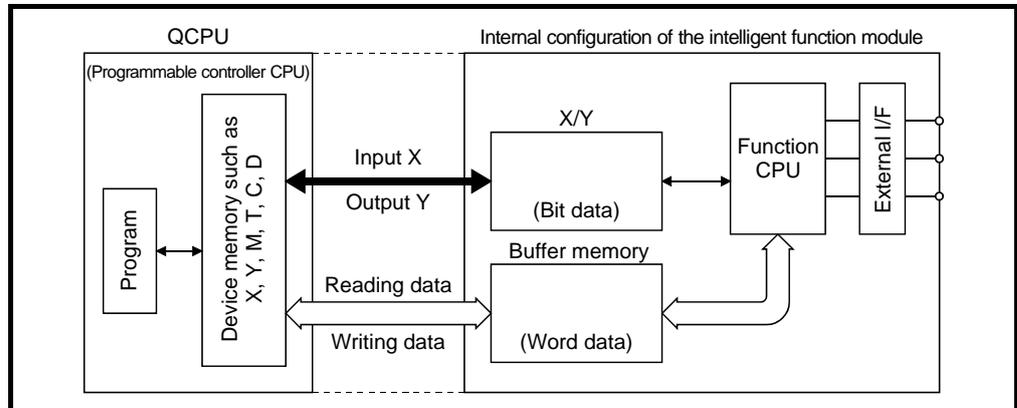
Figure 7.2 Internal configuration of the intelligent function module
