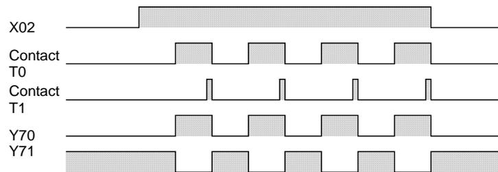
(3) The flip-flop operation starts when X2 is turned on. In this operation, Y70 turns on if the timer T0 is on, and Y71 turns on if the timer T1 is on. (Cycle: 10sec.)
