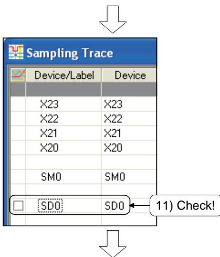
10) Set devices to be traced on the Sampling Trace screen as shown on the left.
