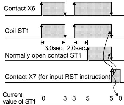
When using the program as a retentive timer, specify the points in parameters in advance.
