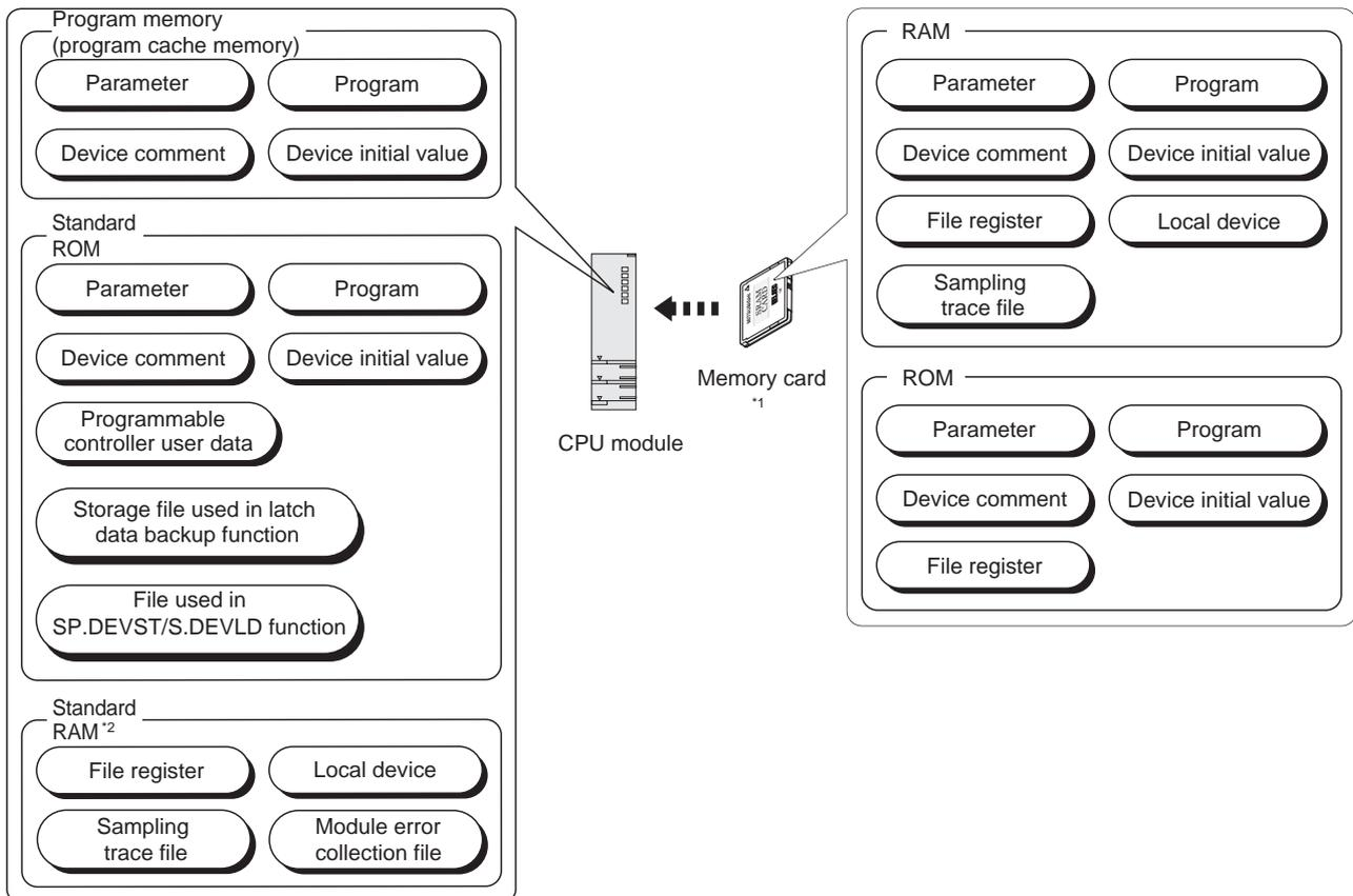
\*1: A memory card cannot be used for Q00UJCPU, Q00UCPU, Q01UCPU.
