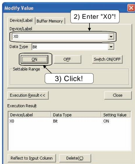
2) The Modify Value dialog box is displayed. Input "X0" to the "Device/Label" list box.
