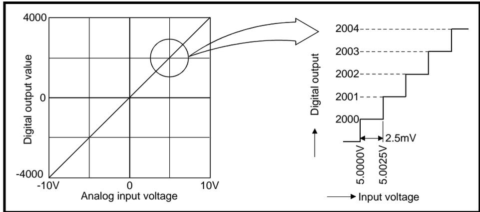
Figure 7.12 A/D conversion characteristics (voltage input)
