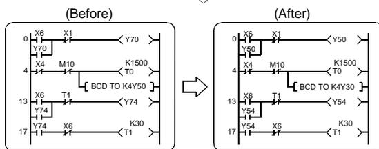
6) Confirm that the target device numbers are replaced.
