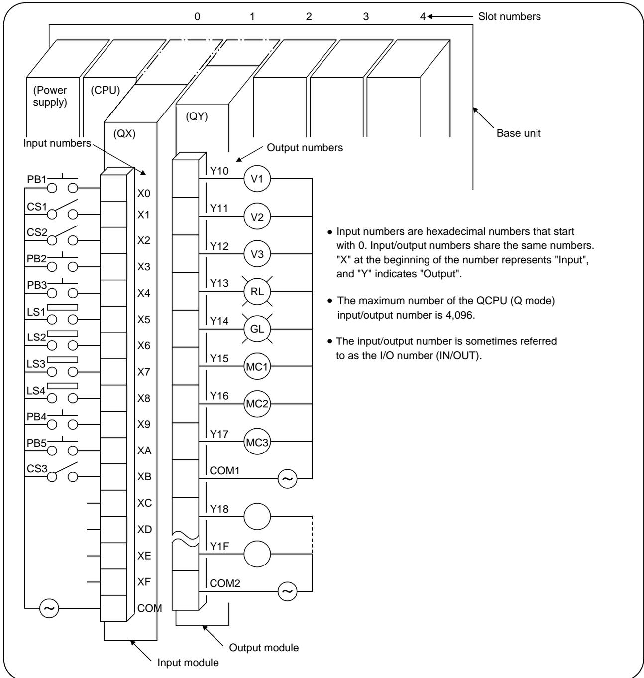
Figure 1.4 Wiring of I/O devices
