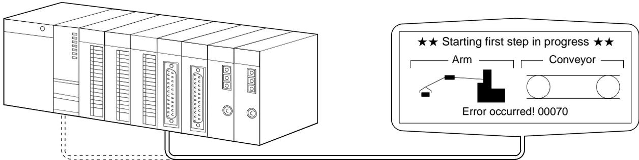
MELSEC-Q supports a wide variety of GOTs (Graphic Operation Terminals). In addition to the error display function, GOTs have a lot of useful functions such as the graphic monitoring, ladder monitoring, device monitoring, touch-panel switch, and printing function.
