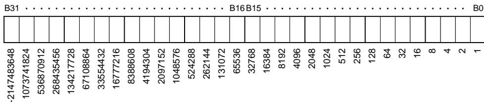
As the case of 16-bit data processing, the programmable controller processes a 32-bit negative value in two's complement. Therefore, the most significant bit B31 (B15 for 16-bit data), is a sign bit.
