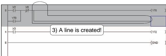
3) A line is created when the left button of the mouse is released.
