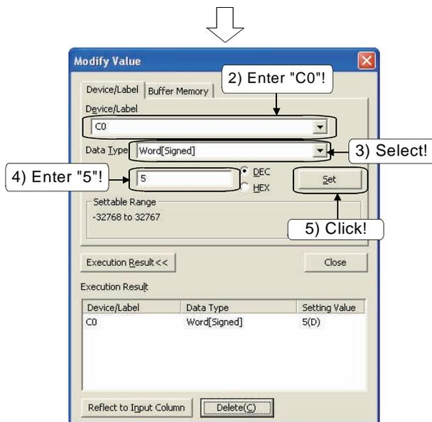
2) The Modify Value dialog box is displayed. Input "C0" to the "Device/Label" list box.
