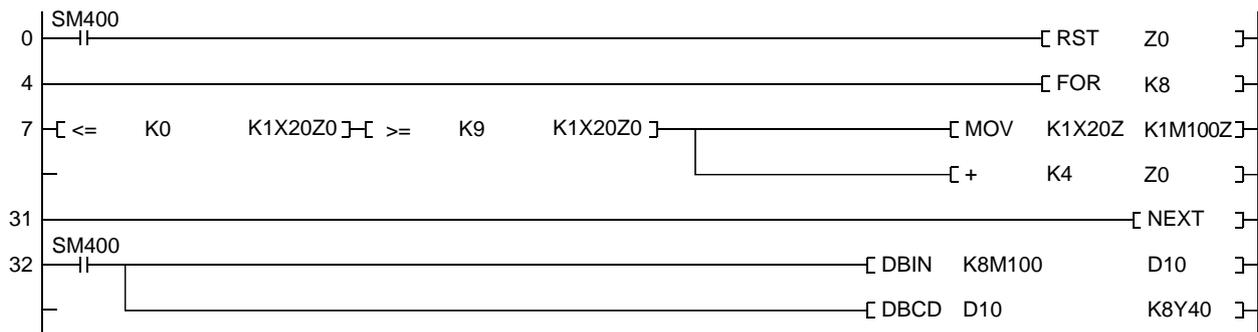
Appendix 4.29 Displaying number of faults and fault numbers using fault detection program
