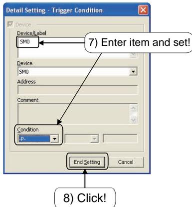
7) The Detail Setting - Trigger Condition dialog box is displayed. Set the following items. In this example, set error occurrence as trigger condition.
