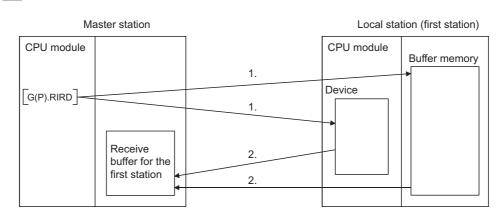
1. The buffer memory in the local station or the device in the CPU module is accessed.
