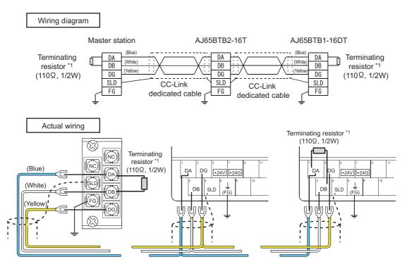
\*1 When a Ver.1.10-compatible CC-Link dedicated cable or CC-Link dedicated cable (Ver.1.00-compatible) is used, connect 110Ω 1/2W (Brown-Brown) terminating resistors.
