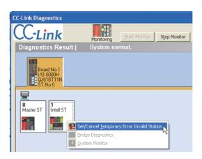
**3.** When the step 2. is performed while the selected station has been set as a temporary error invalid station, the temporary error invalid station setting is canceled.
