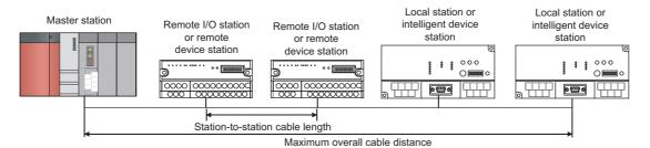
• Ver.1.10-compatible CC-Link dedicated cable (a terminating resistor of  $110\Omega$  used)
