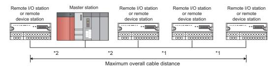
• CC-Link dedicated cable (Ver.1.00-compatible) (a terminating resistor of 110Ω used)
