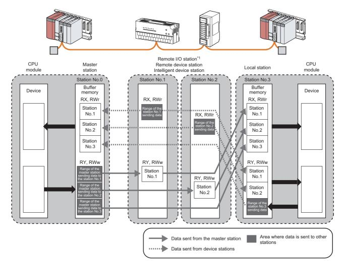
\*1 RWr and RWw are not used for a remote I/O station. Note, however, that buffer memory areas are occupied depending on the mode of the master/local module. () Page 46, Section 3.6.3 to Page 55, Section 3.6.6)
