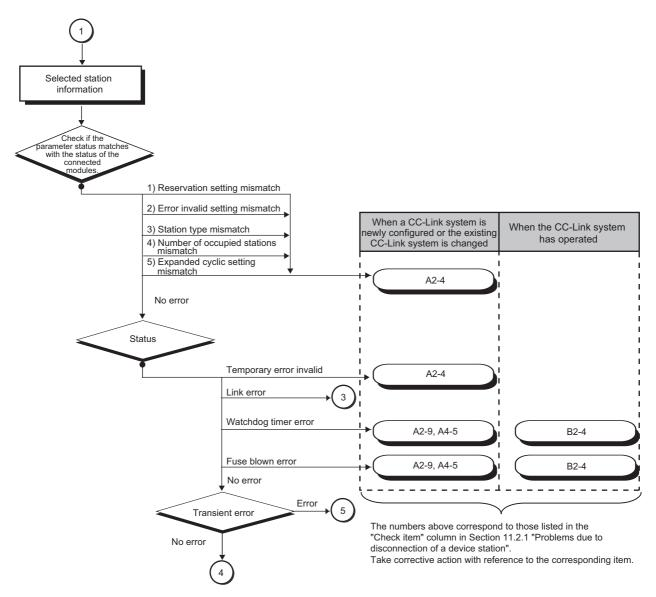
\*1 To check error details, a programming tool is required.
