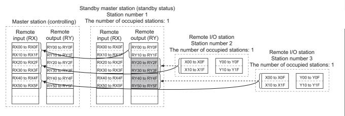
Inputs (RX/RWr) from device stations to the master station are stored in outputs (RY/RWw) of the standby master station (shaded areas in the figure above).
