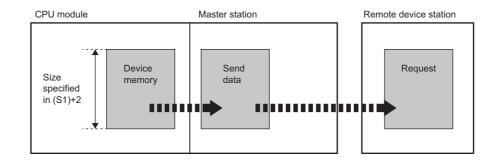
When the send data size ((S1)+2) is an odd number of bytes, the low byte of the last data is sent as the last byte.
