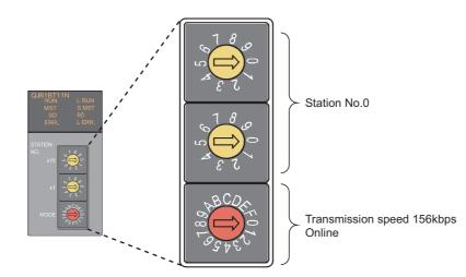
**6.** Set the station number and transmission speed using the switches on the AJ65BTB2-16T and AJ65BTB1-16DT.
