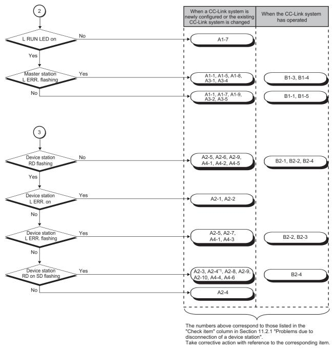
\*1 To check error details, a programming tool is required.
