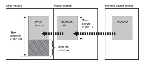
If the receivable data size ((S1)+3) is smaller than the receive data size ((S1)+4), data sent from a remote device station cannot be received.
