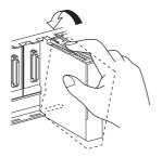
**4.** Connect a CC-Link dedicated cable to each module. Connect terminating resistors to the modules at both ends. (
