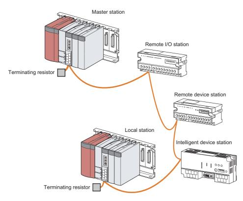
The CC-Link version and the number of device stations that can be connected vary depending on the mode of the master/local module. (Figure 27, Section 3.2.1, Page 43, Section 3.6.2) Master/local modules of other series can be also used in a CC-Link system.
