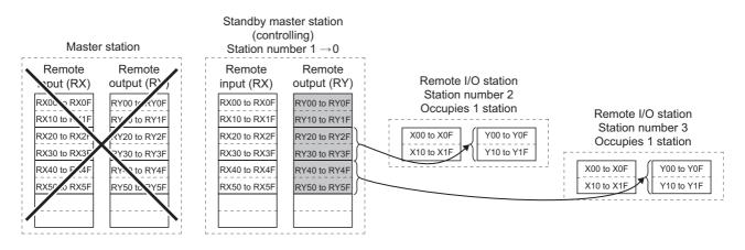
Outputs (RY/RWw) of the master station are stored in inputs (RX/RWr) of the standby master station. By transferring the inputs (RX/RWr) of the standby master station to the outputs (RY/RWw), outputs to the device stations are continued (shaded areas in the figure above). ([] Page 147, Section 8.2.5 (7))
