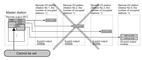
The parameter cannot be set using dedicated instructions. Therefore, read or write data from/to the device in a CPU module according to the number of I/O points of each station using a program. Consequently, the areas in refresh devices can be saved.
