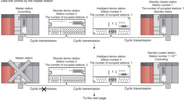
\*1 When the master station goes down and the standby master station starts to take in control of data link, the station number of the standby master station becomes 0.
