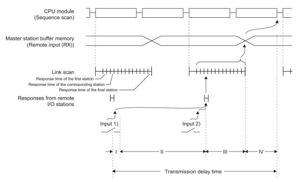
I: Delay time due to response delay of the remote I/O station
