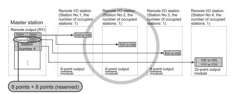
When the number of remote I/O stations is odd, eight points cannot be set in the remote station points.
