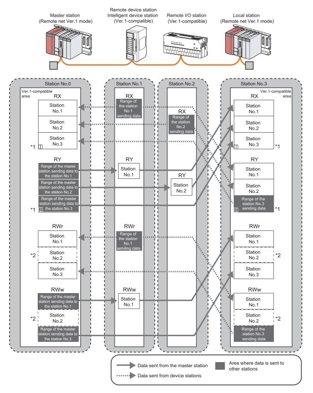
\*1 The last two bits in RX and RY cannot be used for communications between a master station and a local station.
