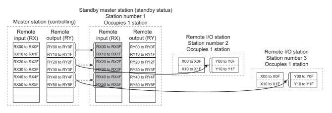
Outputs (RY/RWw) from the master station are stored in inputs (RX/RWr) of the standby master station (shaded areas in the figure above).
