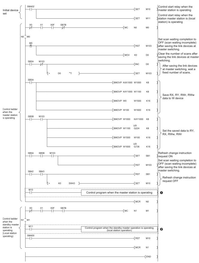
\*1 After saving the link devices, wait a fixed number of scans and execute the processing that sets the link devices saved at master switching and Refresh instruction at standby master switching (SB0001). For details, refer to Page 143, Section 8.2.5 (5).
