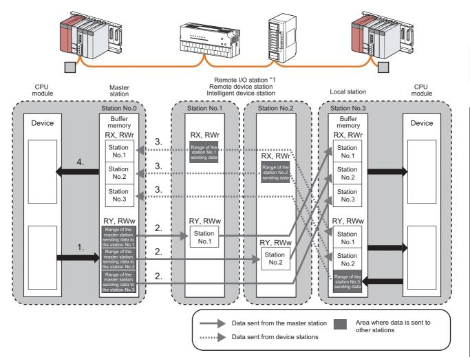
\*1 RWr and RWw are not used for a remote I/O station. Note, however, that buffer memory areas are occupied depending on the mode of the master/local module. (SP Page 46, Section 3.6.3, Page 55, Section 3.6.6)
