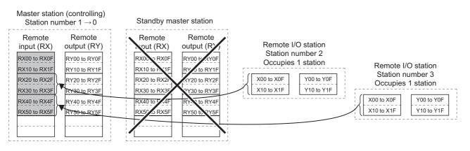
Inputs (RX/RWr) of the standby master station are stored in the outputs (RY/RWw) of the master station. By transferring the outputs (RY/RWw) of the master station to the inputs (RX/RWr), inputs from the device stations are continued (shaded areas in the figure above). ([] Page 147, Section 8.2.5 (7))
