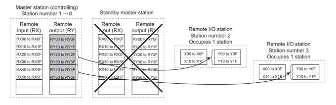
Outputs (RY/RWw) of the standby master station are stored in inputs (RX/RWr) of the master station. By transferring the inputs (RX/RWr) of the master station to the outputs (RY/RWw), outputs to the device stations are continued (shaded areas in the figure above). ([] Page 147, Section 8.2.5 (7))
