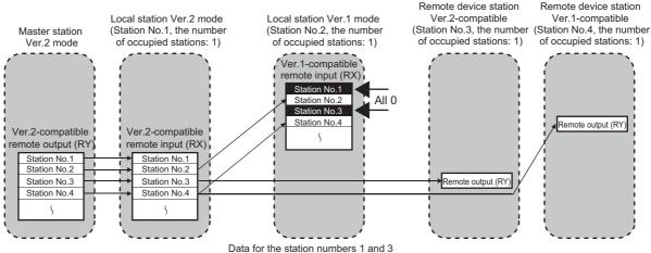
Data for the station numbers 1 and 3 in the Ver.2-compatible device station is 0.
