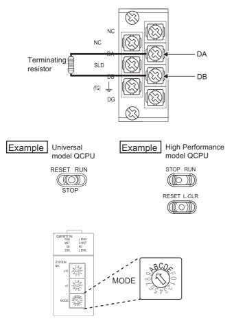
Connect the terminating resistor provided with the master/local module between the DA and DB terminals on the terminal block of the master/local module.
