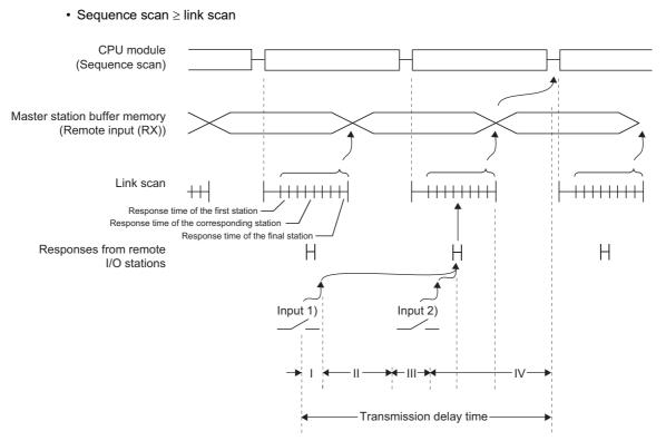
I: Delay time due to response delay of the remote I/O station
