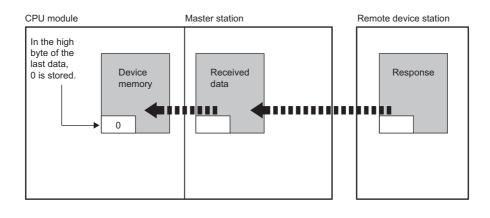
• When the receive data size ((s1)+4) is an odd byte (when data received from a remote device station is an odd byte)
