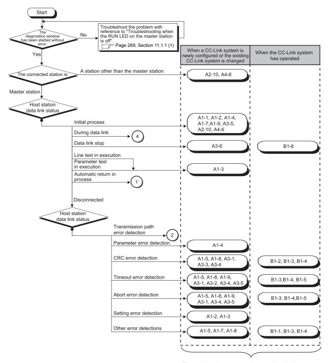
The numbers above correspond to those listed in the "Check item" column in Section 11.2.1 "Problems due to disconnection of a device station". Take corrective action with reference to the corresponding item.
