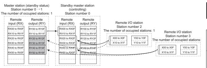
Inputs (RX/RWr) from device stations to the standby master station are stored in outputs (RY/RWw) of the master station (shaded areas in the figure above).
