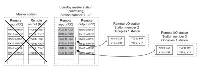
Inputs (RX/RWr) of the master station are stored in outputs (RY/RWw) of the standby master station. By transferring the outputs (RY/RWw) of the standby master station to the inputs (RX/RWr), inputs from the device stations are continued (shaded areas in the figure above). (
