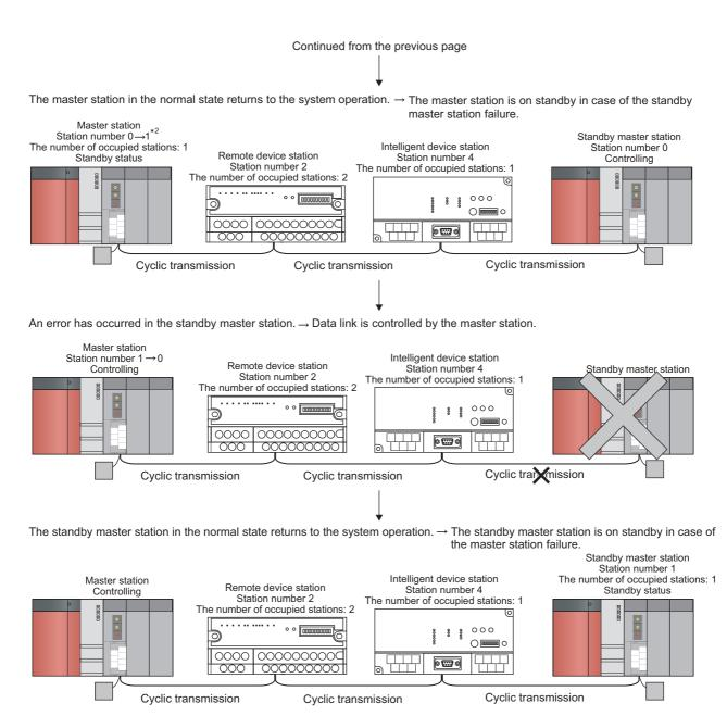
\*2 When the master station returns as a standby master station, the station number of the master station becomes the number set in "Standby Master Station No." of the network parameter.
