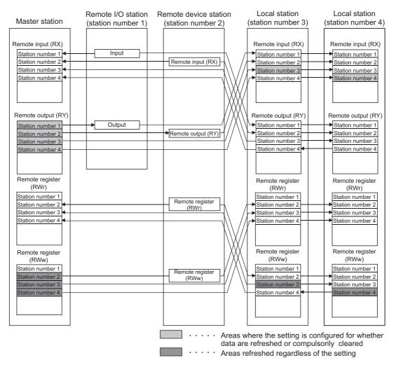
Only remote output (RY) is refreshed or compulsorily cleared according to the setting. Remote input (RX) and remote register (RWr/RWw) are refreshed even if the switches on the CPU modules in the master station and local stations are set to STOP, regardless of the setting.
