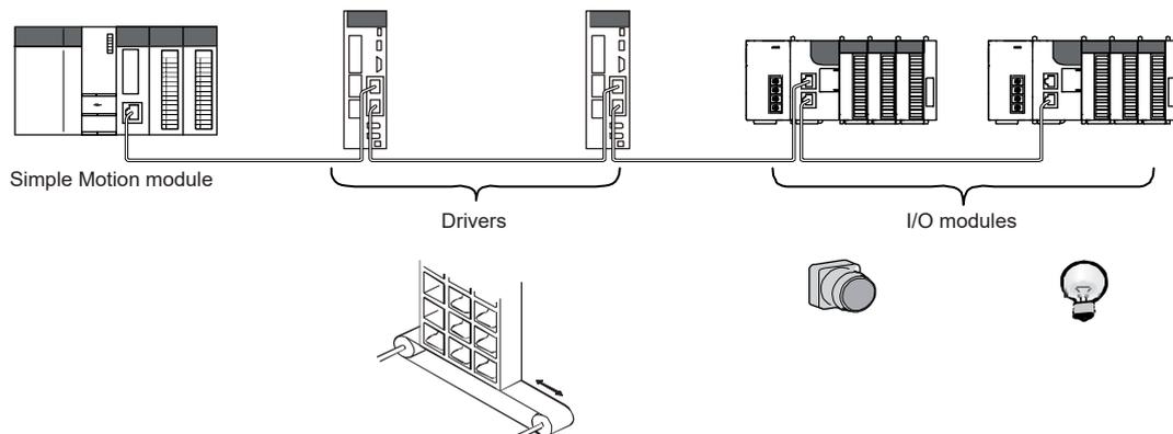
(3) Multiple axes system configuration
