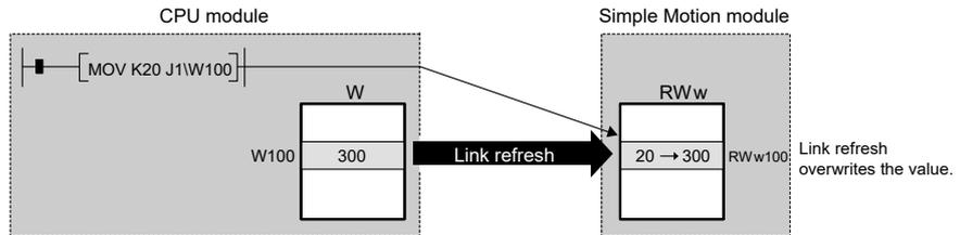
Good example (In addition to direct access, writing the same data to the CPU module device)
