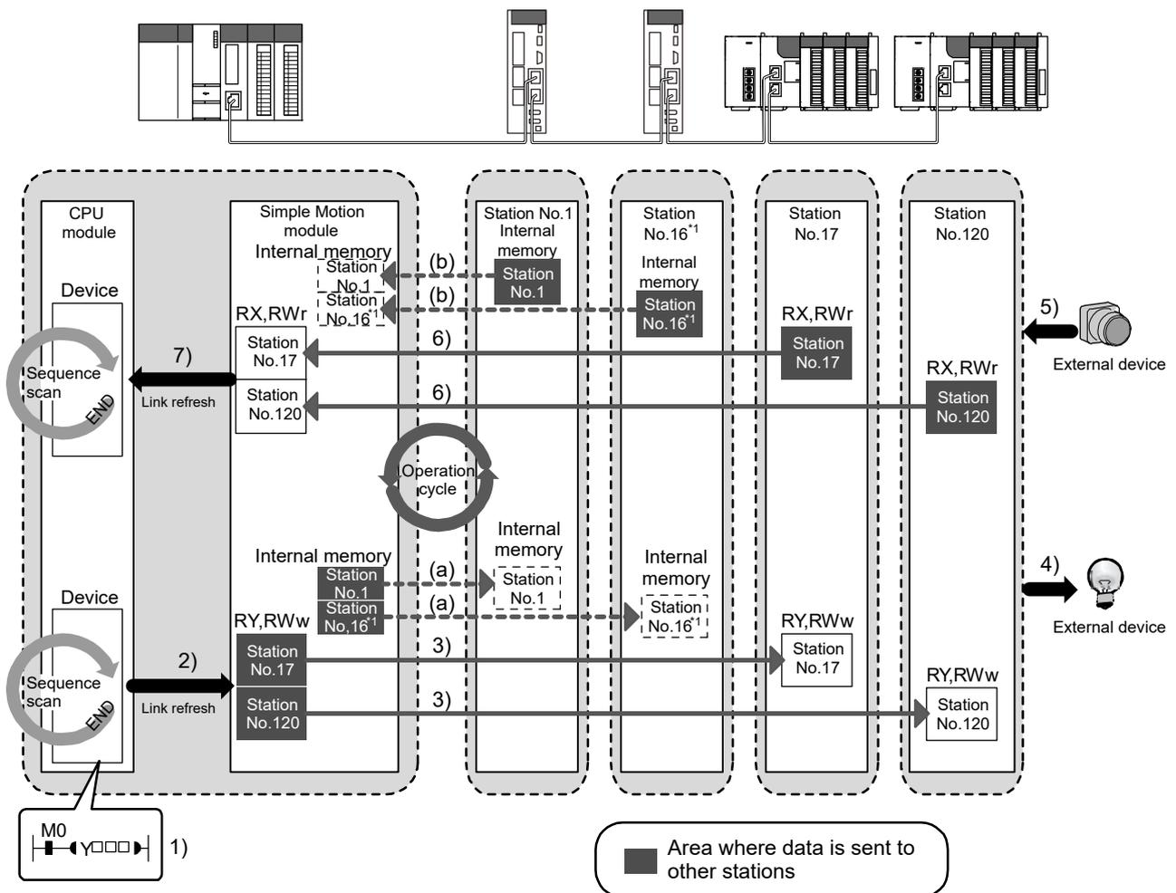
\*1: The range from the station No.1 to 4 is valid in the 4-axis module, and the range from the station No.1 to 8 is valid in the 8-axis module.
