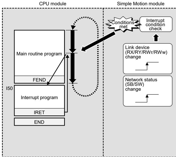
Interrupt program events by the Simple Motion module are shown below.
