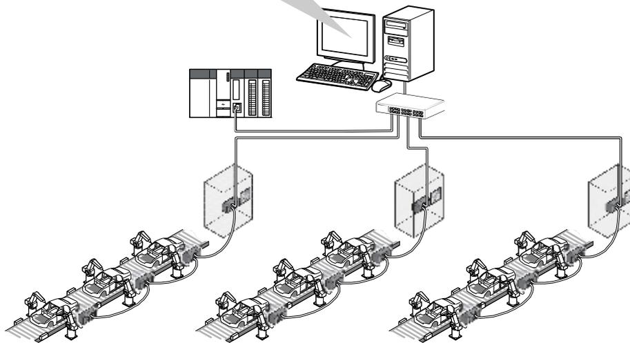
(7) Adding CC-Link IE Field Network devices without stopping the system
