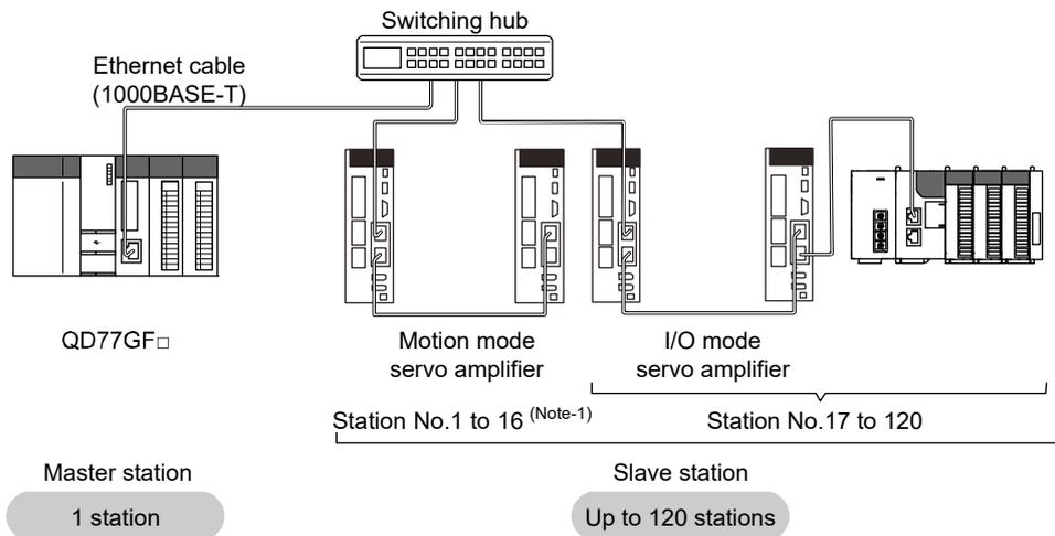
Set the station No. as shown below depending on the connected device to the Simple Motion module.
