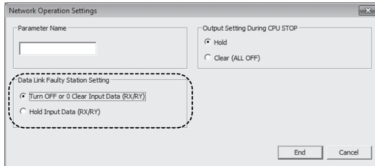
(b) Cyclic data output when a stop error occurs in the CPU module
