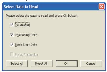
4) Check the data to read and click . The set data is read to the QD75P\(\text{N}\)/QD75D\(\text{N}\).
