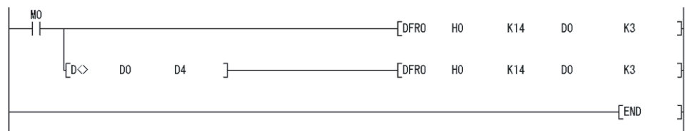
Figure 5.13 Periodic pulse counter value reading program example
