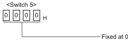
**Figure 6.7 Intelligent function module switch setting: Use prohibited**
