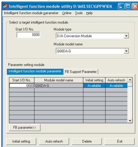
Enter "Start I/O No.", and select "Module type" and "Module model name".
