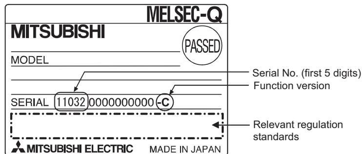
(b) Checking on the front of the module
