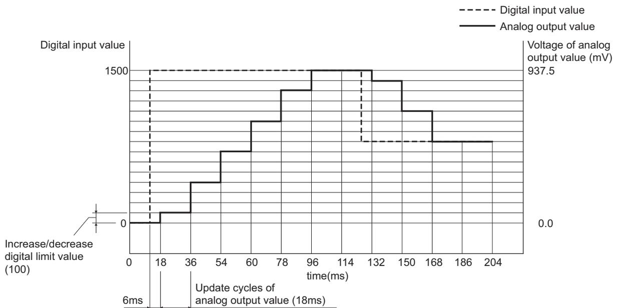
When the digital input value changes, the analog output value increases or decreases in update cycles as follows:
