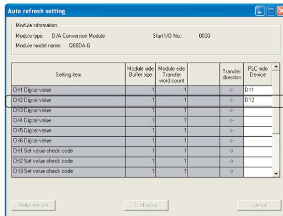
This one row is counted as one setting. Blank rows are not counted. Count up all the setting items on this screen, and add the total to the number of settings for other intelligent function modules to get a grand total.
