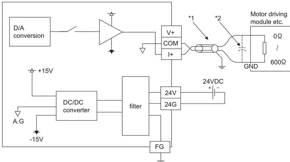
\*1 For wire, use the shielded twisted pair cable.
