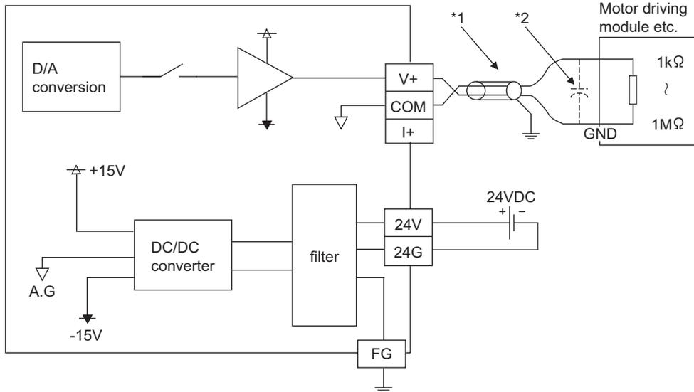
\*1 For wire, use the shielded twisted pair cable.
