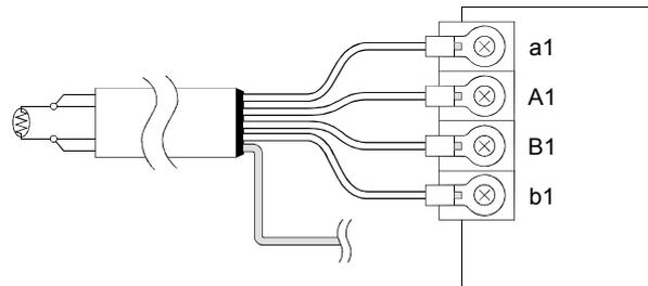
When 3-wire type is selected in switch 3 of intelligent function module switch setting
