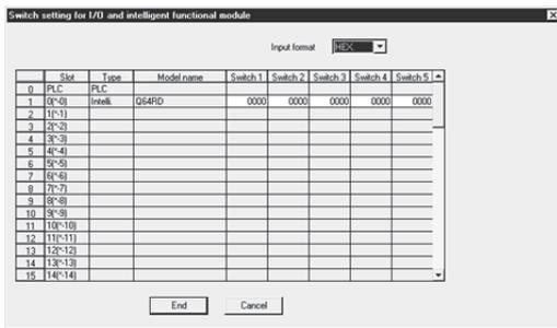
(b) Switch setting for intelligent function module screen
