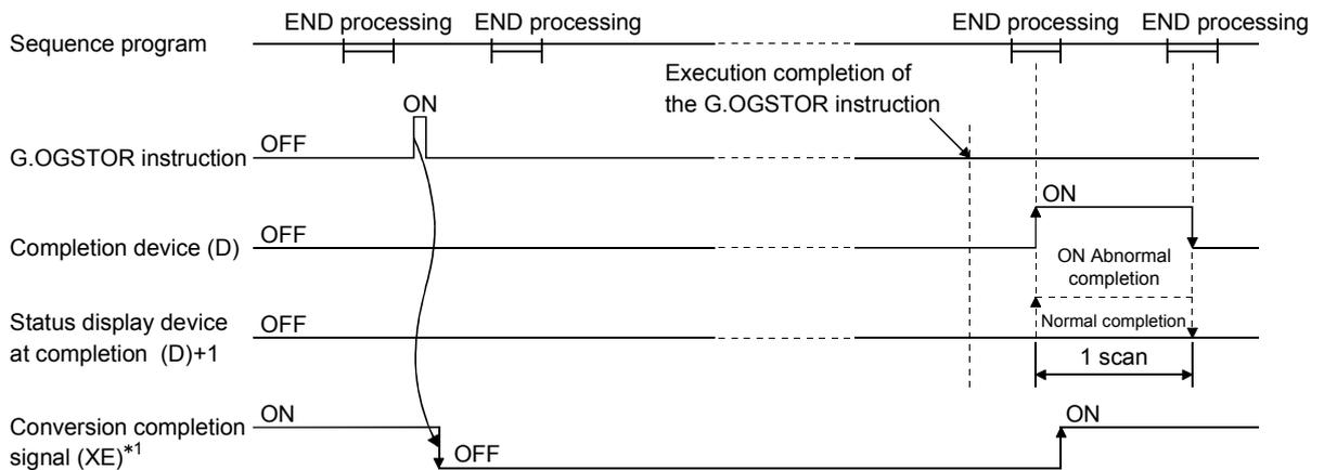
\*1 When the G(P).OGSTOR instruction is executed, A/D conversion is not performed. After the completion device (D) turns ON, A/D conversion starts, the A/D conversion value is stored into the buffer memory, and the conversion completion signal (XE) then turns ON.
