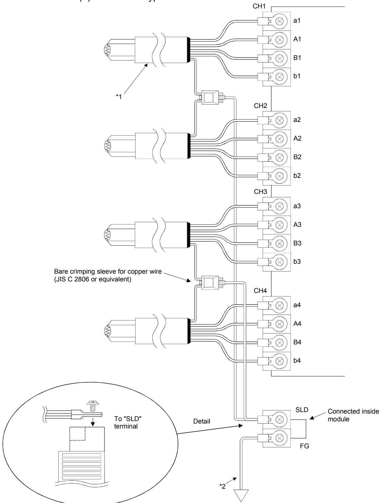
\* 1 Use the conducting cable with shield and make the wiring length as short as possible.
