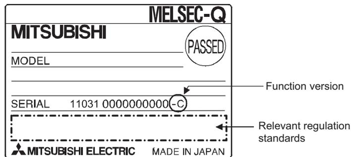
Figure 2.2 Rating plate on the side of module
