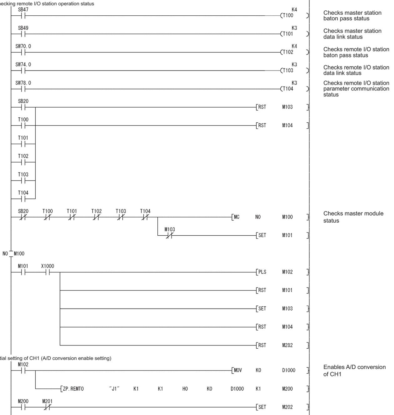
Figure 9.24 Program example without using GX Configurator-AD
