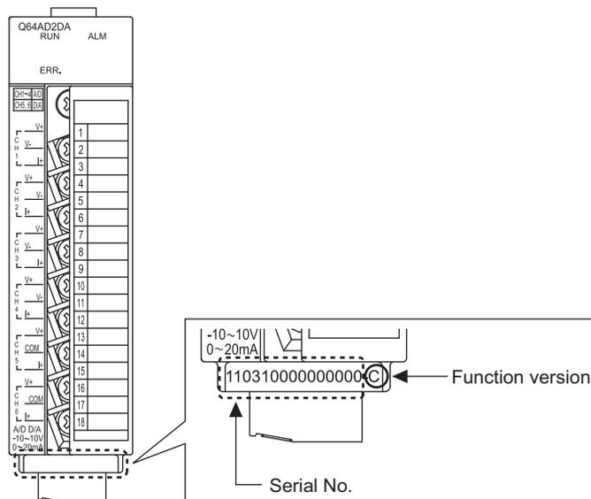
Figure 2.3 Description on the front part of module
