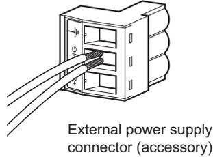
**Figure 3.1 When inserting two cables into one terminal**
