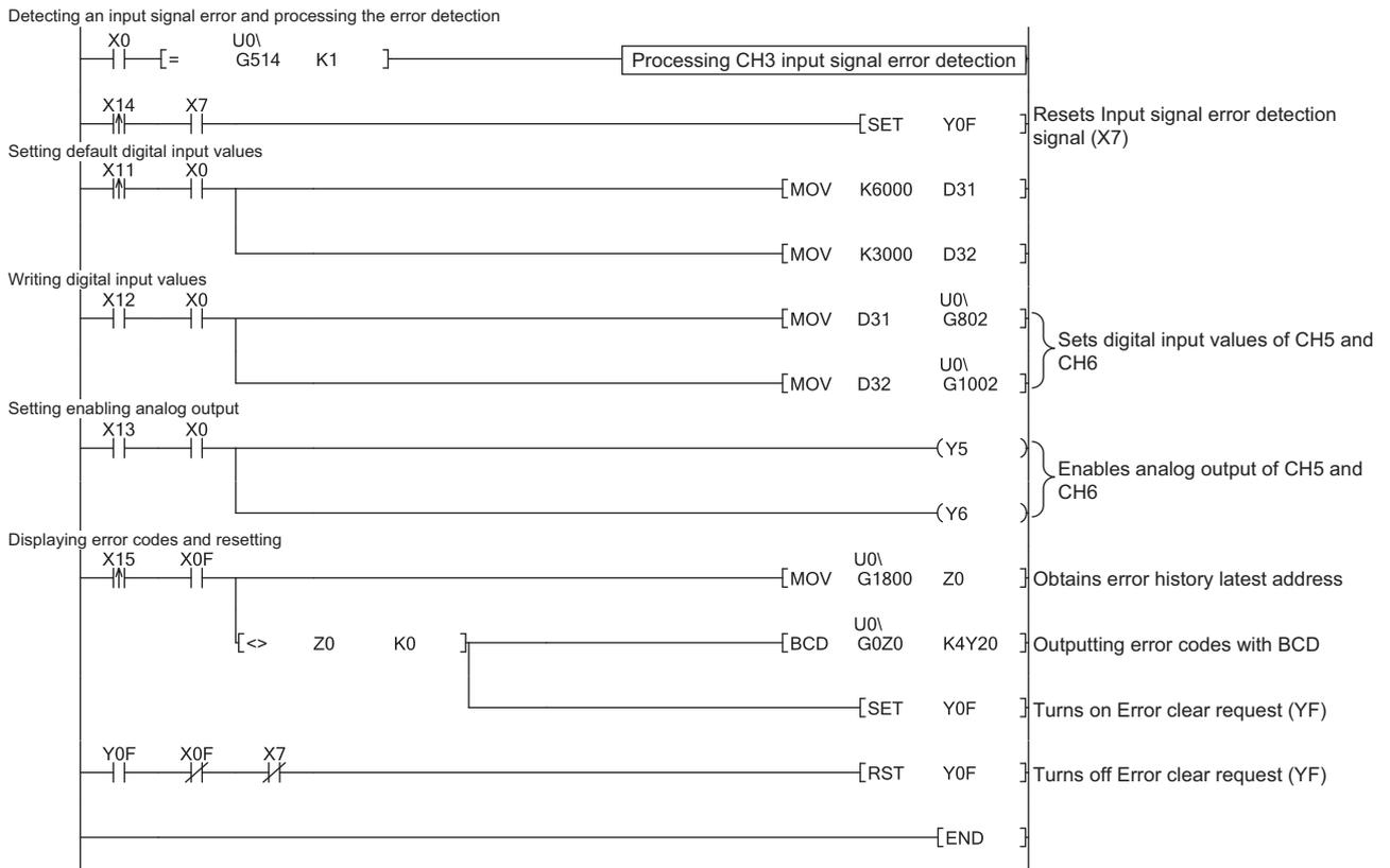
Figure 9.15 Program example without using GX Configurator-AD (continued)
