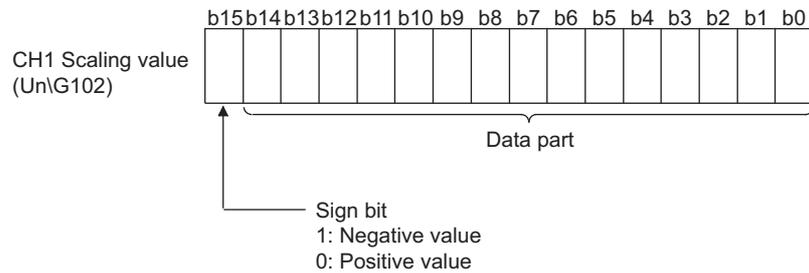
Figure 6.5 Storage data of CH1 Scaling value (Un\G102)
