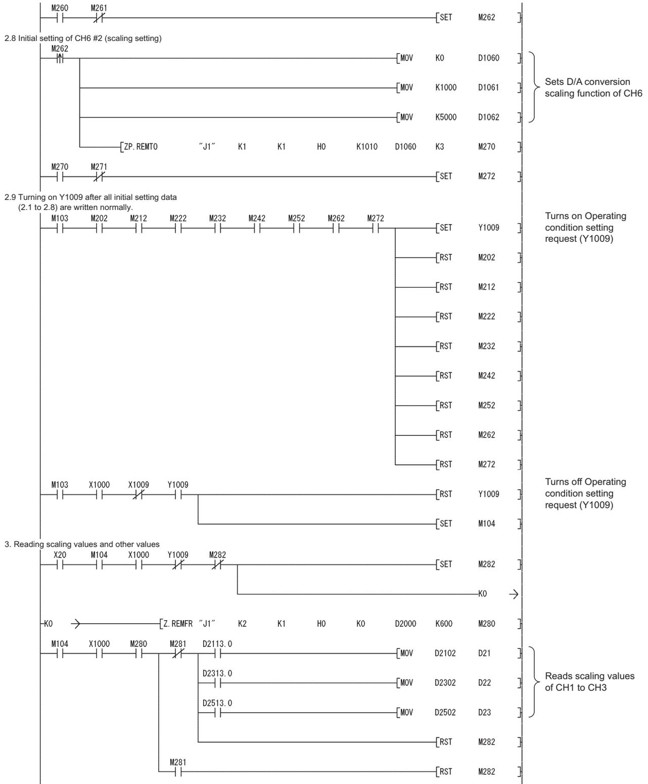
Figure 9.24 Program example without using GX Configurator-AD (continued)
