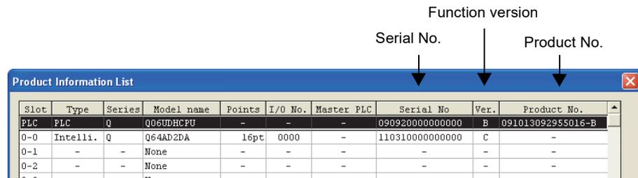
Figure 2.4 Checking the serial number and function version
