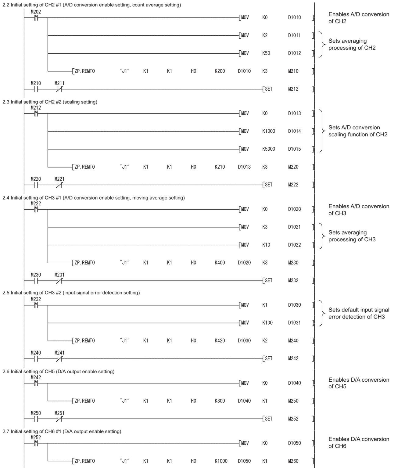
Figure 9.24 Program example without using GX Configurator-AD (continued)
