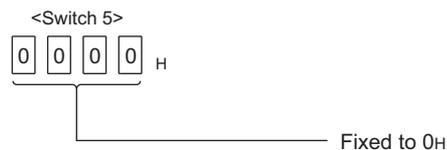
Figure 9.8 Intelligent function module switch setting: Use prohibited
