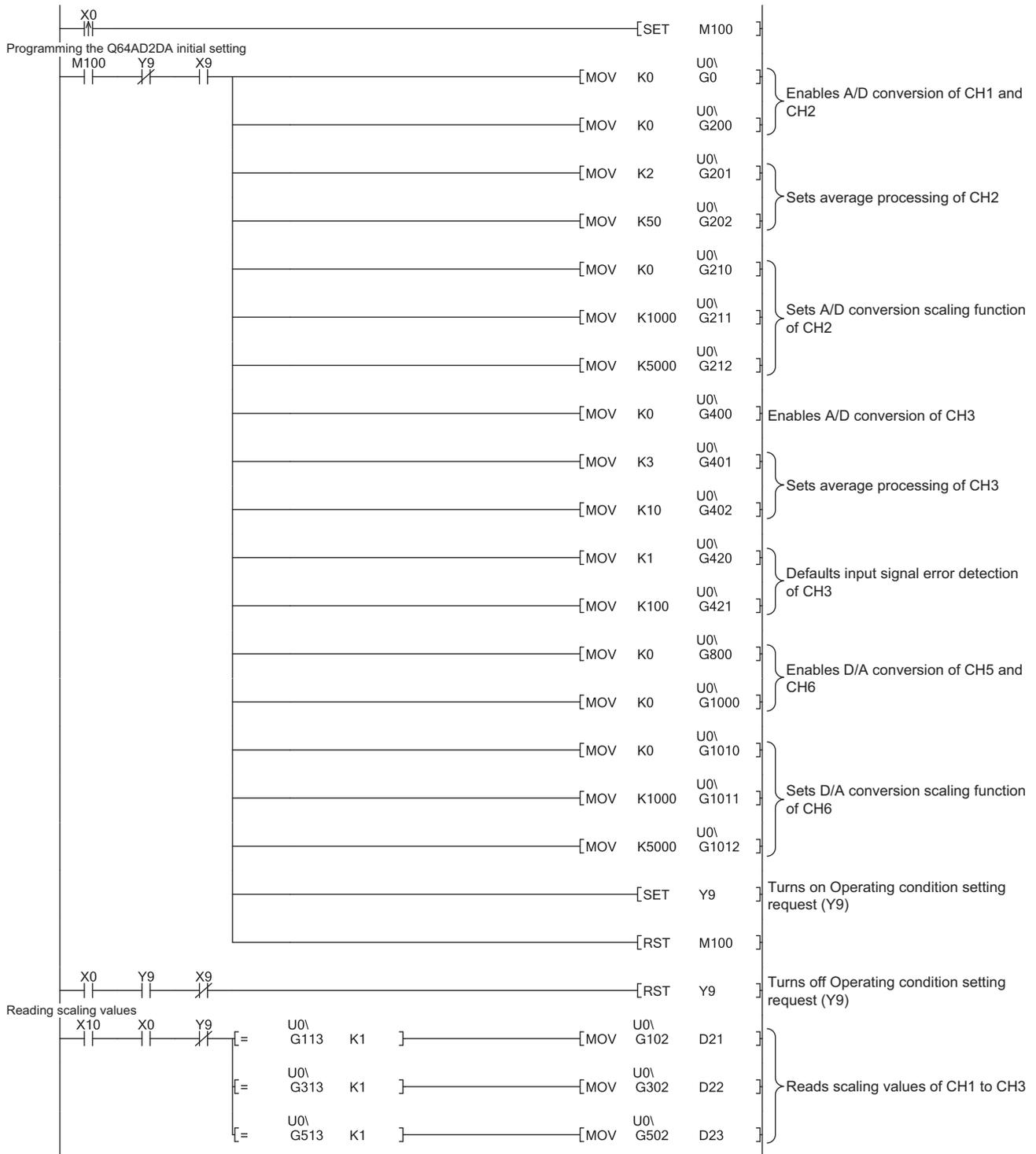
Figure 9.15 Program example without using GX Configurator-AD
