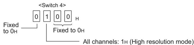
Figure 9.7 Intelligent function module switch setting: Resolution setting
