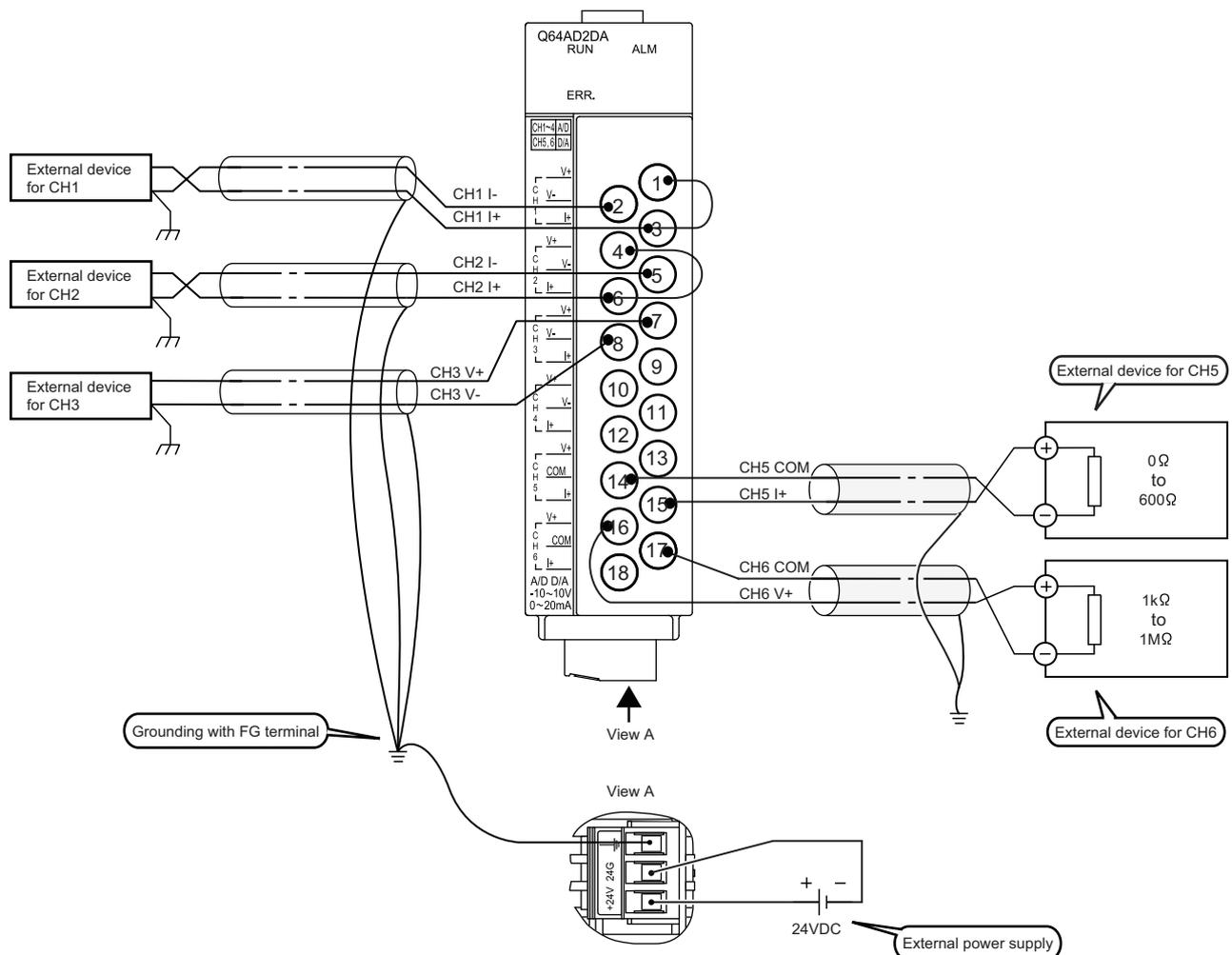
Figure 9.3 Wiring example for the program examples
