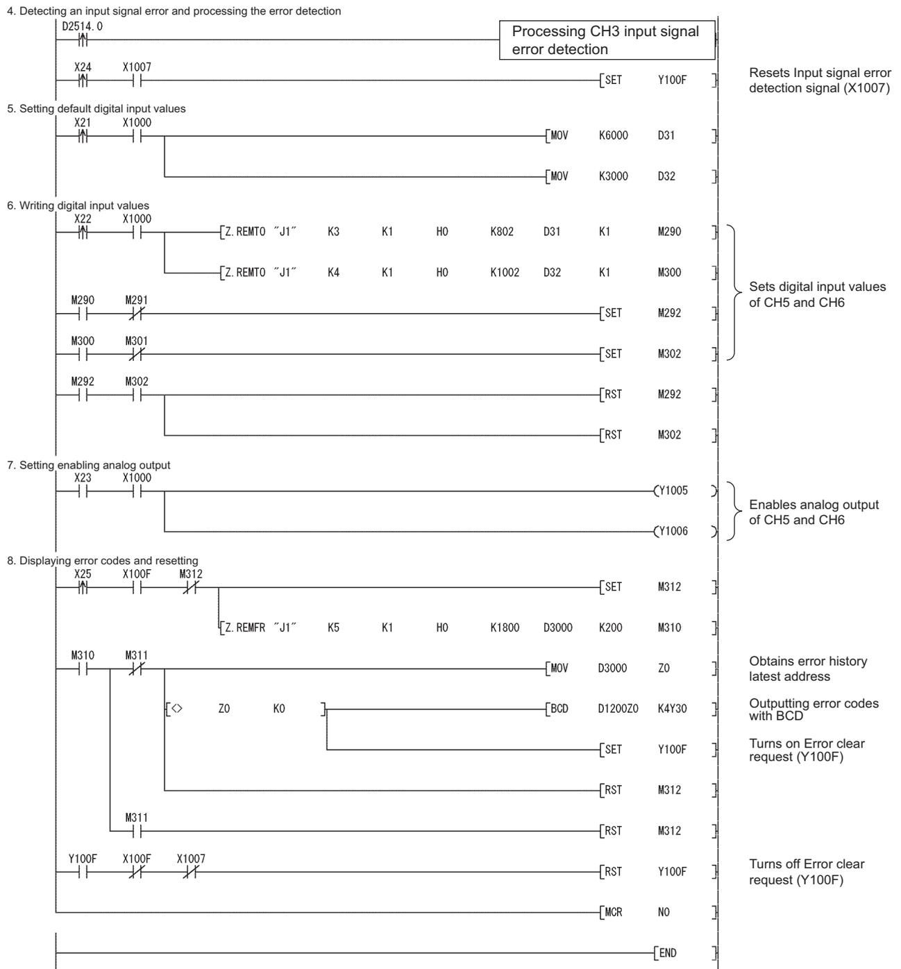
Figure 9.24 Program example without using GX Configurator-AD (continued)
