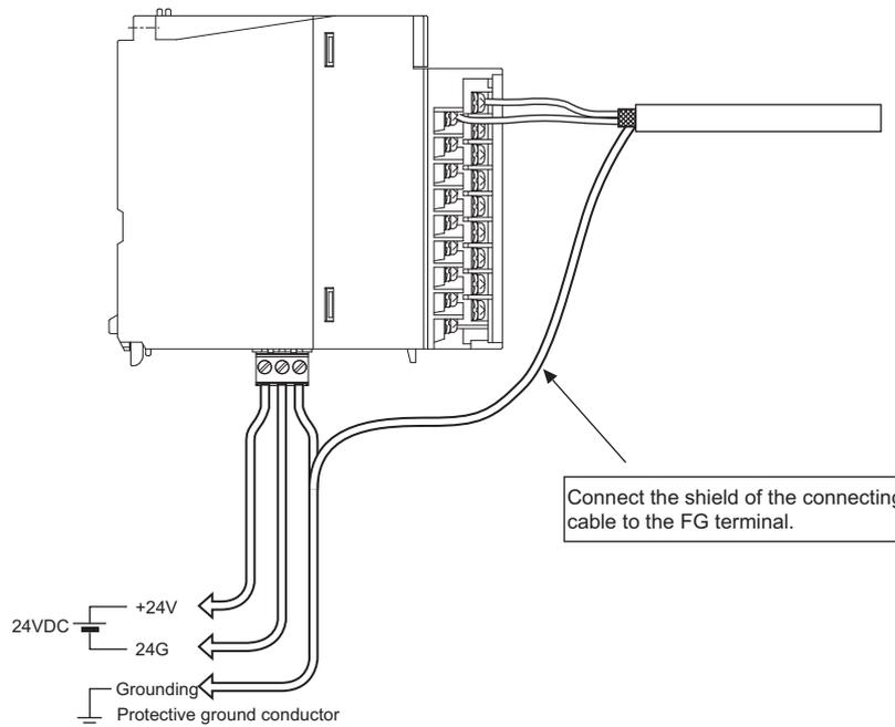
Figure 7.9 Wiring example of shielded twisted pair cable
