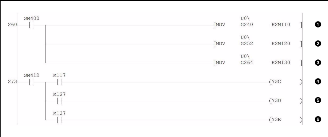
Fig. 6-14: HART field device status check and error processing
