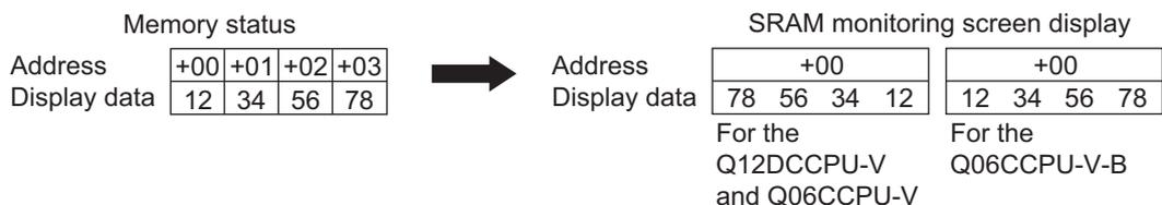
**Figure 4.7 Display example when "32 bits" is selected**
