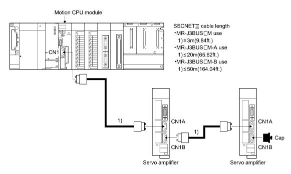
(Note): It cannot communicate if the connection of CN1A and CN1B is mistaken.
