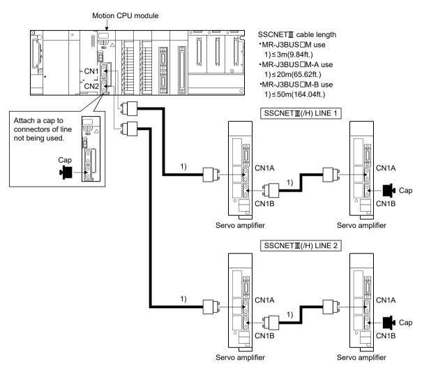
(Note): It cannot communicate if the connection of CN1A and CN1B is mistaken.
