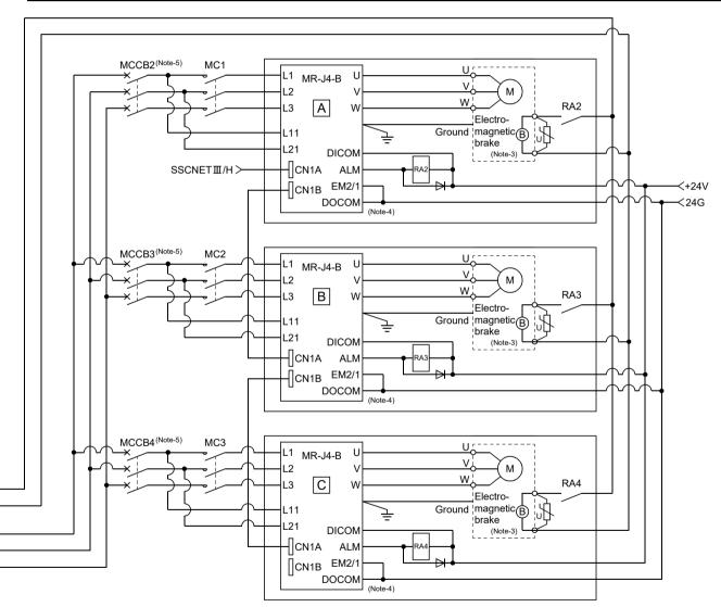
(Note-1): When the control power supply of servo amplifier is shut off, it is not possible to communicate with the servo amplifier after that. Example) When the control power supply L11/L21 of servo amplifier in figure  $\Box$  above is shut off, it is also not possible to communicate with the servo amplifier  $\Box$ .
