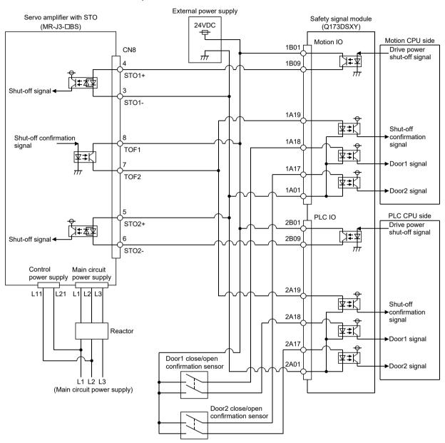
(c) Wiring example for external pulse input to safety signal module. The wiring diagram for external pulse input signal and safety signal module shows below.
