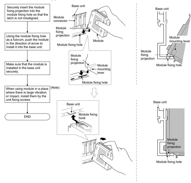
(Note): Screw the Motion CPU module to the main base unit.
