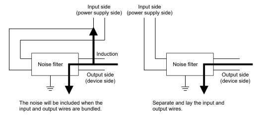
Figure 7.4 Precautions on noise filter
