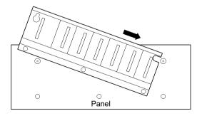
(c) Place the left-hand side pear-shaped hole of the base unit onto the left-hand side screw.
