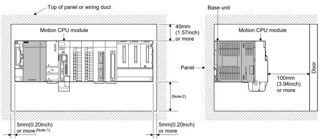
(Note-1): 20mm (0.79inch) or more when the adjacent module is not removed and the extension cable is connected. (Note-2): Q173DSCPU/Q172DSCPU use-----70mm (2.76inch) or more Q173DCPU(-S1)/Q172DCPU(-S1) use ----100mm (3.94inch) or more
