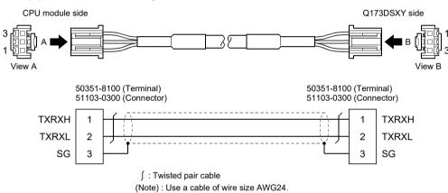
APPENDIX 1.7 SSCNETⅢ cables (SC-J3BUS□M-C) manufactured by Mitsubishi Electric System & Service Co., Ltd.
