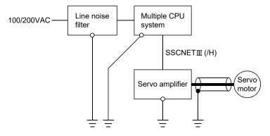
(Note): Be sure to ground the line noise filter, Multiple CPU system, servo amplifier and servo motor. (Ground resistance:  $100 \Omega$  or less)
