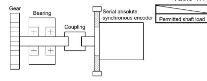
(2) Excessive load is applied to the shaft of serial absolute synchronous encoder by the large mounting errors in eccentricity and angle of deviation. As a result, it might damage the machine or shorten extremely the life. Minimize loads applied to the shaft such that they make within the permitted shaft load range.
