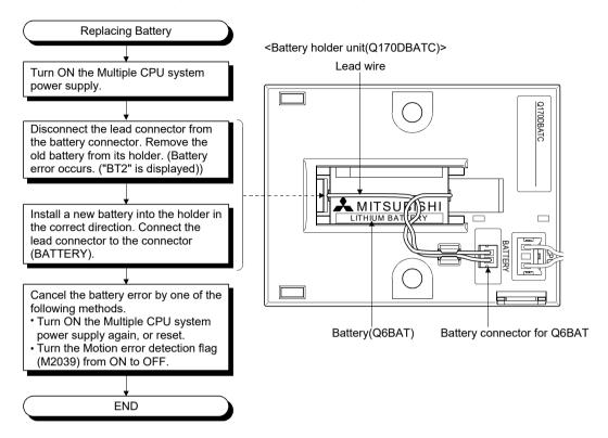
(2) Q172DEX module battery replacement procedure
