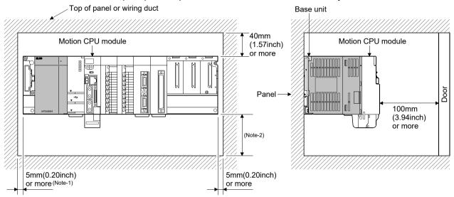
(Note-1): 20mm (0.79inch) or more when the adjacent module is not removed and the extension cable is connected. (Note-2): Q173DSCPU/Q172DSCPU use-----70mm (2.76inch) or more Q173DCPU(-S1)/Q172DCPU(-S1) use ----100mm (3.94inch) or more
