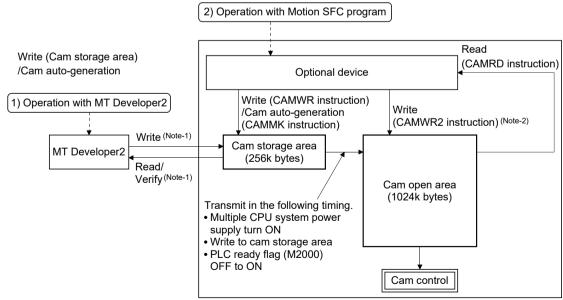
(Note-1): Write/read/verify from MT Developer2 is executed toward cam storage area. (Note-2): The directly writing in cam open area is not transmitted to cam storage area. The data in cam open area will be returned as cam storage area such as the Multiple CPU system power supply ON again.
