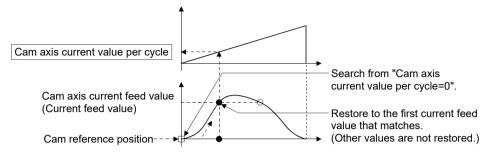
2) Search from a value in the middle of the cam axis current value per cycle. (Cam data starting point = 0)
