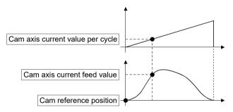
Select from 3 objects as follows in [Pr.462] Cam axis position restoration object (D15102+150n) which position is to be restored.
