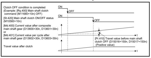
(7) [Pr.411] Main shaft clutch smoothing method (D15018+150n) Set the smoothing method for clutch ON/OFF.
