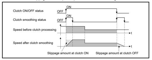
(c) Operation at input speed deceleration during slippage method smoothing When the speed before clutch processing decreases, the speed after clutch smoothing is controlled without exceeding the speed before clutch processing.
