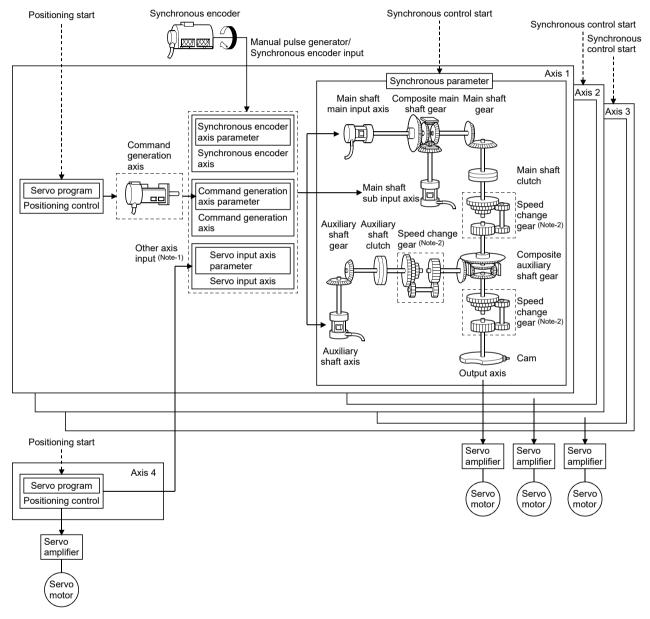
(Note-1): It is possible to drive the servo input axis except the positioning control (home position return, manual control, speed-torque control, synchronous control).
