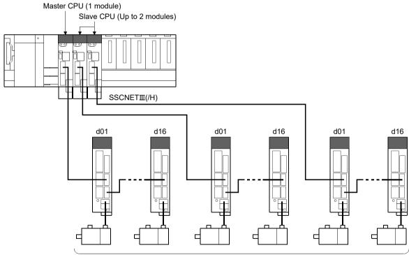
MR-J5(W)- $\square$ B/MR-J4(W)- $\square$ B/MR-J3(W)- $\square$ B/MR-JE- $\square$ B model servo amplifier Up to 96 axes (32 axes × 3 CPU)/system
