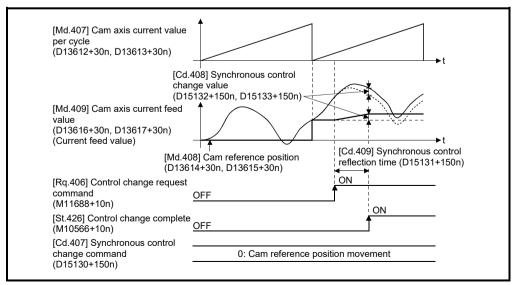
When [Rq.406] Control change request command (M11688+10n) is reset to OFF while executing the cam reference position movement command, operation is stopped midway. If the cam reference position movement command is executed again, the remainder travel value is not reflected, and the operation starts with [Cd.408] Synchronous control change value (D15132+150n,D15133+150n) to be used again.
