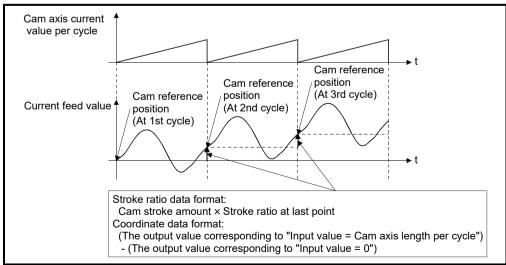
Create cam data for two-way cam operation as shown below.
