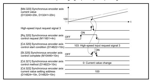
Set the control method for the synchronous encoder axis in [Cd.321] Synchronous encoder axis control method.
