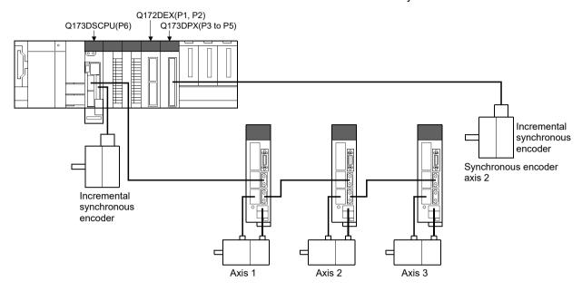
Set the following in [Pr.320] Synchronous encoder axis type for the synchronous encoder axis 2 on the synchronous encoder axis parameter screen of MT Developer2.
