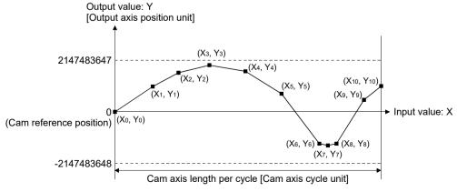
When the coordinate data corresponding to an input value that is 0 or when the cam axis length per cycle setting does not exist, the coordinate is calculated from the line segment between the nearest two coordinates.
