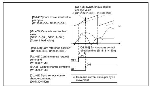
When [Rq.406] Control change request command (M11688+10n) is reset to OFF while executing the cam axis current value per cycle movement, operation is stopped midway. If the cam axis current value per cycle movement is executed again, the remainder travel value is not reflected, and the operation starts with [Cd.408] Synchronous control change value (D15132+150n, D15133+150n) to be used again.
