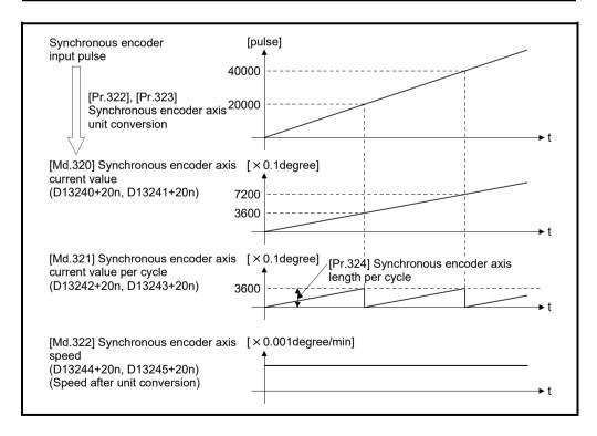
(5) [Pr.325] Synchronous encoder axis smoothing time constant Set the averaging time to execute a smoothing process for the input travel value from synchronous encoder.
