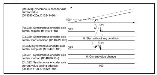
When this signal is ON, if "101 to 132" is set to [Cd.320] Synchronous encoder axis control start condition (D14822+10n), the synchronous encoder axis control starts based on the corresponding high-speed input request signal.
