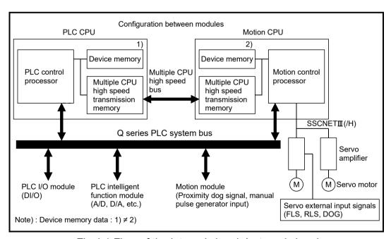
Fig.4.1 Flow of the internal signals/external signals
