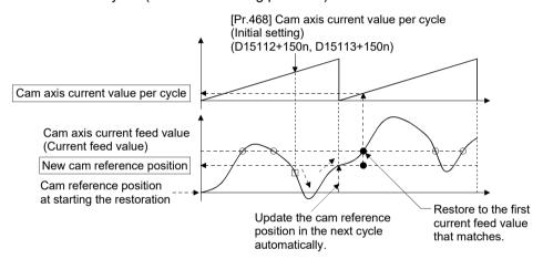
3) Search from a value in the middle of the cam axis current value per cycle. (Cam data starting point  $\neq$  0)
