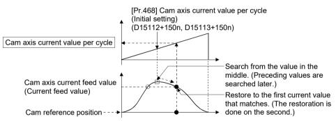
Search from a value in the middle of the cam axis current value per cycle. (Cam data starting point ≠ 0)
