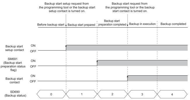
If the backup start contact is turned on while the value in SD690 is  $0_H$  (Before backup start) or  $1_H$  (Backup start prepared), data are not backed up.
