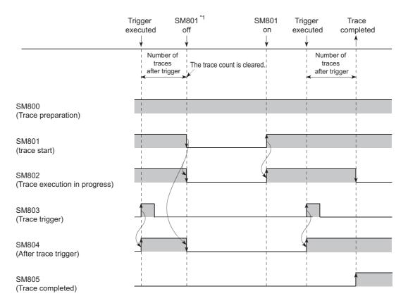
\*1 SM800 also turns off when the sampling trace is suspended by programming tool.
