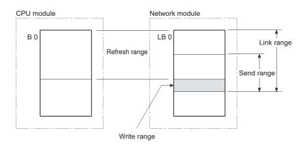
Although writing can be done to a refresh range portion (specified by refresh parameters) within the link device range, the link module's link device data will be overwritten when a refresh occurs.
