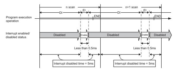
The execution time of a fixed scan execution type program whose execution interval is set to 10ms increases 100ms ( $5 \div 0.5 \times 10 = 100$ ) at the most.
