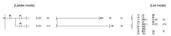
In Example 2, in the ladder block starting from the step 15, the AND<> instruction of the step 17 or 21 is supposed to be not executed when M0 (valid data flag) is off.
