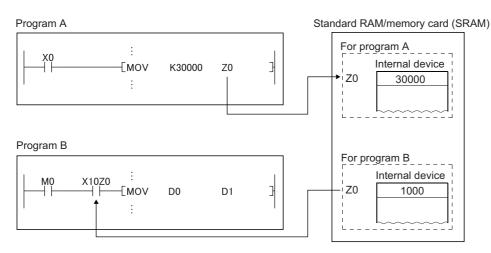
Ex. When the index register is not used as a local device
