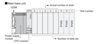
The number of points for the empty slots will be either value set on the PLC system tab, or on the I/O Assignment tab in the PLC parameter dialog box. (The default is 16 points.)
