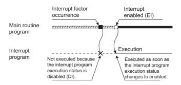
When the same interrupt factor occurs more than one time before the interrupt program execution status is enabled, the interrupt factors of I0 to I15, I28 to I31, I45, I50 to I255 and fixed scan execution type programs are stored only once. For details on the IMASK instruction, refer to the following.
