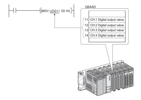
If the intelligent function module device is used, device comments can be attached to the buffer memory areas.
