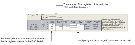
Once the points for the extended data register (D) and extended link register (W) is set, areas for these devices are reserved in the file register file.
