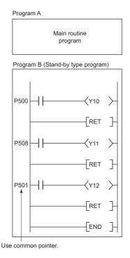
After execution of the standby type program, the CPU module re-executes the program that called a program in the standby type program. The following figure shows the operation when the subroutine and interrupt programs in the standby type program are executed.
