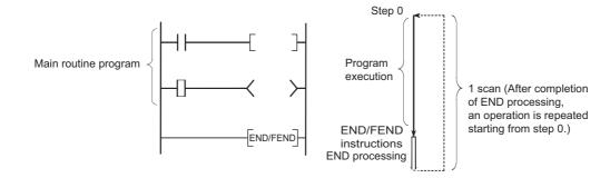
A main routine program can be divided into subroutine programs. A subroutine program is from a pointer (P<sup>II</sup>) to the RET instruction, and is created between the FEND and END instructions. This program is executed only when called by an instruction, such as CALL(P) and FCALL(P), from a main routine program.
