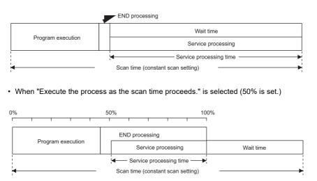
Even when there is no waiting time, the service processing (0.2ms) is performed. Therefore, when the waiting time is less than 0.2ms, the constant scan time may be exceeded.
