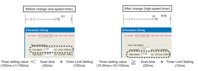
The following show the examples of the coil and the contact being simultaneously turned on if the values are set to become "Timer setting value < Scan time + Timer Limit Setting":
