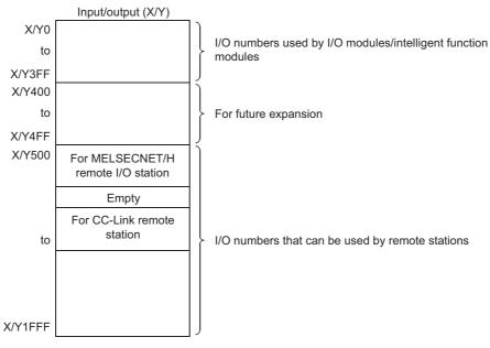
When X/Y0 to 3FF (1024 points) are used by I/O modules and/or intelligent function modules and X/Y400 to 4FF (256 points) are secured for future extension
