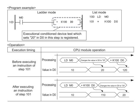
Note that there may be a case where a device value will not be changed depending on the execution timing even though the specified step is executed. The following instructions need to be noted when registering executional conditioned device test settings.
