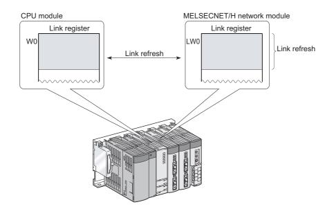
In the link register, numeric data (-32768 to 32767, or  $0000_{\text{H}}$  to FFFF<sub>H</sub>) are stored.
