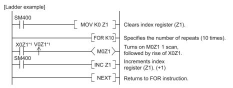
\*1 The on/off information for X0Z1 is stored in the V0Z1 edge relay. For example, the on/off information of X0 is stored in V0, and that of X1 is stored in V1.
