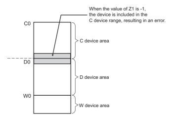
When an error is detected, check the index modification value (value of Z1 in the above example) and remove the error cause.
