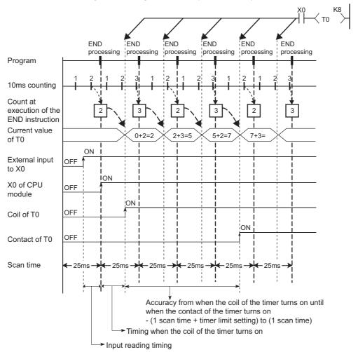
Timer limit setting=10ms, Setting value of T0=8 (10ms×8=80ms), Scan time=25ms
