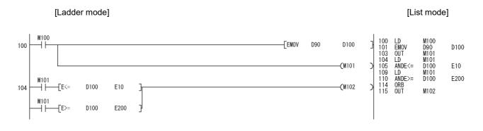
Ex.5) Program after modification for Example 3) ("OPERATION ERROR" (error code: 4140) is no longer detected.)
