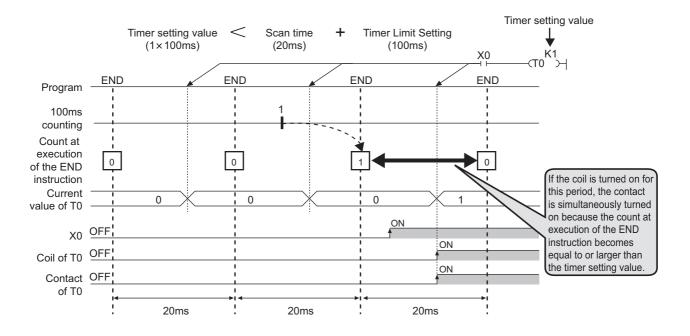
Ex. When the timer setting value is 2 (2 × 100ms), the scan time is 110ms, and the timer limit setting is 100ms If the coil of the timer (T0) is turned on at the next scan after the values satisfy "Count at execution of the END instruction ≥ Timer setting value", the coil and the contact are simultaneously turned on because the values satisfy "Timer current value = Timer setting value" at the start of the timer.
