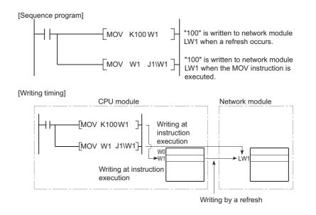
• If data are written to another station's write range using a link direct device, the data will be overwritten with other data that are received from the corresponding station.
