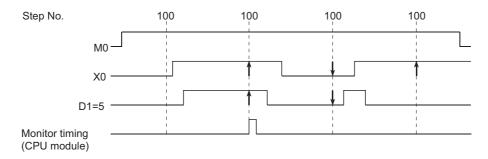
• With the High-speed Universal model QCPU and Universal model Process CPU, only the first data which satisfies the specified conditions is collected if the step between the FOR and NEXT instructions is specified.
