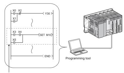
Change a program with programming tool and write it to the CPU module in the RUN status.
