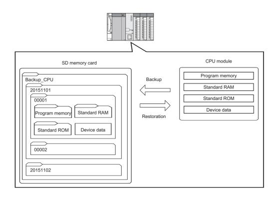
The following table lists the backup and restoration methods of the CPU module data backup/restoration function.
