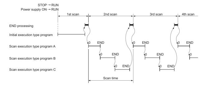
When multiple scan execution type programs are executed, the scan time will be the time required for completing all the scan execution type program execution. If an interrupt program or fixed scan execution type program is executed, execution time of the executed program will be added to the scan time.
