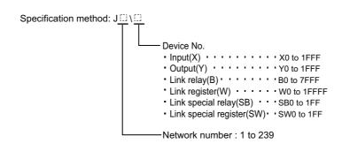
For a CC-Link IE Field Network master/local module, specify the device with a network number and a device number as shown below.
