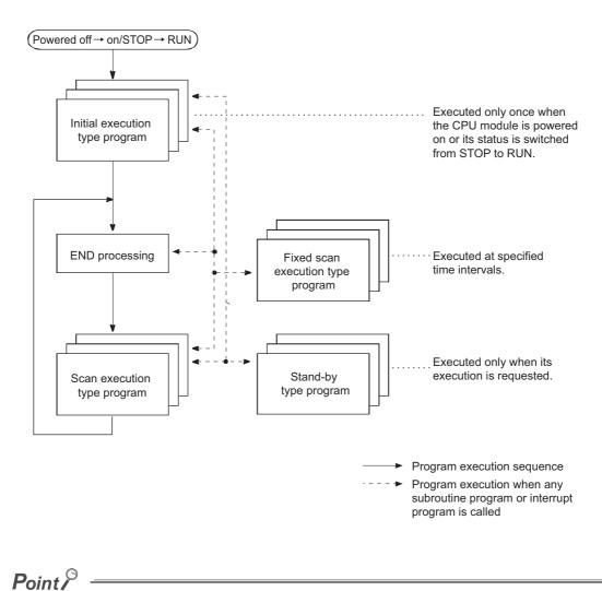
Use initial execution type program, stand-by type program, and fixed scan execution type program as required.
