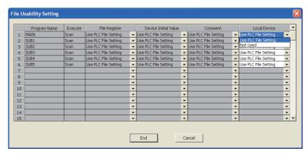
\*1 Even file usability of local device file cannot be set if the serial number (first five digits) of the Q02UCPU, Q03UDCPU, Q04UDHCPU, or Q06UDHCPU is "10011" or earlier. If the local device is set to be used in the PLC file tab of the PLC parameter dialog box in the High Performance model QCPU, all the programs use the local device in the Universal model QCPU after replacement.
