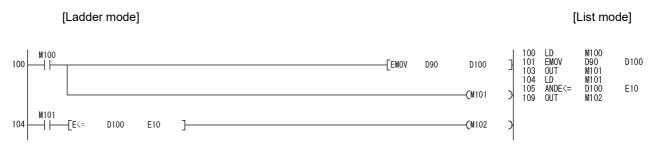
In the ladder block starting from the step 104, the ANDE<= instruction of the step 105 is not executed when the M101 (valid data flag) is off.
