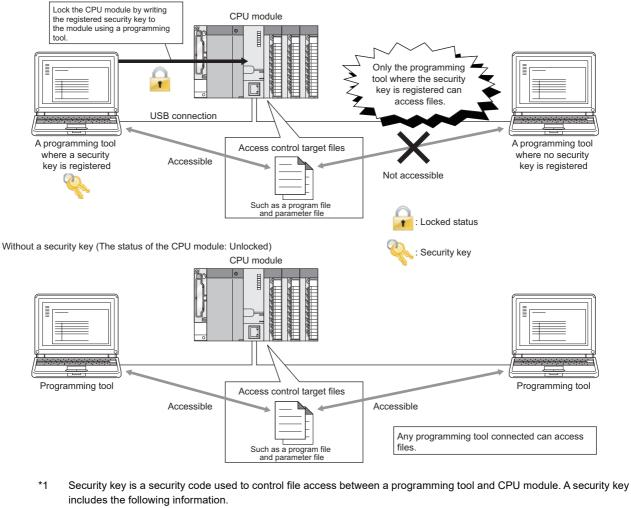
With a security key (The status of the CPU module: Locked)
