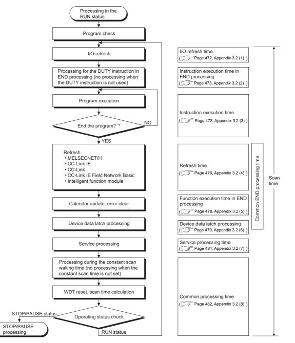
\*1 End of a program indicates the timing when the END, GOEND, FEND, or STOP instruction is executed.
