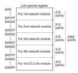
For details of the link special register, refer to the manual for each intelligent function module that has the link special register.
