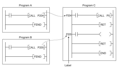
The common pointer is used to call subroutine programs from all programs that are being executed.
