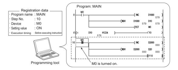
Note that a device value is changed within the specified step regardless of an execution status of the instruction in the specified step.
