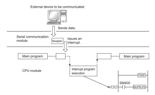
To execute an interrupt program by an interrupt from the intelligent function module, select "Intelligent Function Module Interrupt Pointer Setting" in "Intelligent Function Module Setting" of the PLC system tab in the PLC parameter dialog box.
