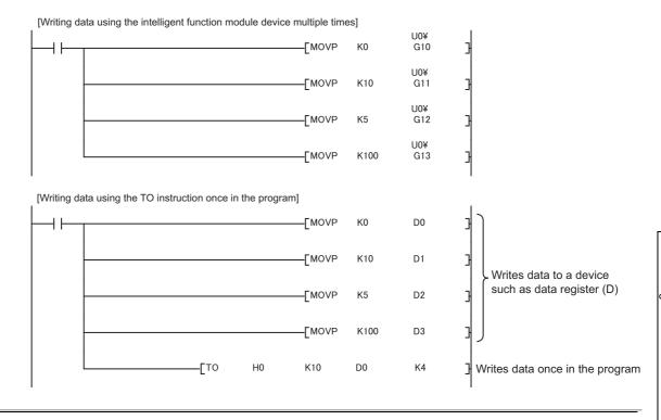
For buffer memory addresses and applications, refer to the manual for each intelligent function module used. For the FROM and TO instructions, refer to the following.
