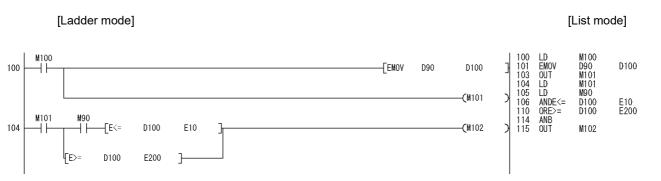
In the ladder block starting from the step 104, the ANDE<= instruction of the step 106 and the ORE>= instruction of the step 110 are not executed when the M101 (valid data flag) is off.
