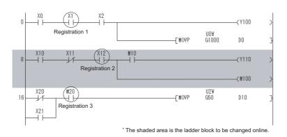
Example 2) When multiple ladder blocks are changed online, ladder blocks between the change target ladder blocks will be included in the change target. For this reason, if the online change function is executed as follows, all registrations 1 to 3 are disabled.
