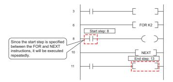
· High-speed Universal model QCPU and Universal model Process CPU The High-speed Universal model QCPU and Universal model Process CPU recognize only the first start step and ignores the second and later start steps. Scan time required to execute the program between the first start step and the end step is measured.
