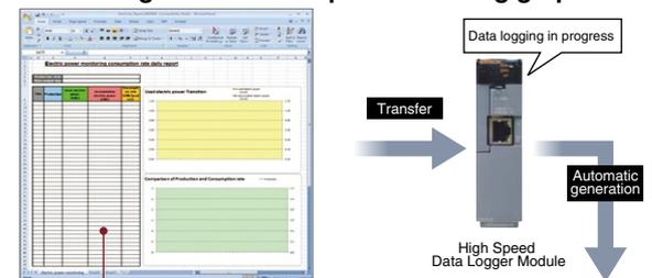
Layout files (forms that are empty) are created in Excel® and transferred to the module using the configuration tool.
