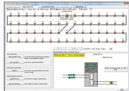
View the network connection status of entire system to identify problems at a glance. The cause of problems can be quickly identified and suggested remedies implemented to minimize down time.
