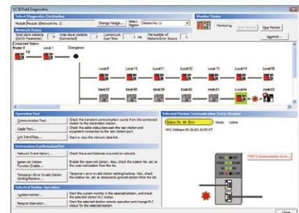
The network diagnostic tools in GX Works2\*3 allow problems to be identified rapidly. In addition to a visual overview of the network and several other tools, detailed monitoring of CPUs and modules from any station, to any station is possible.
