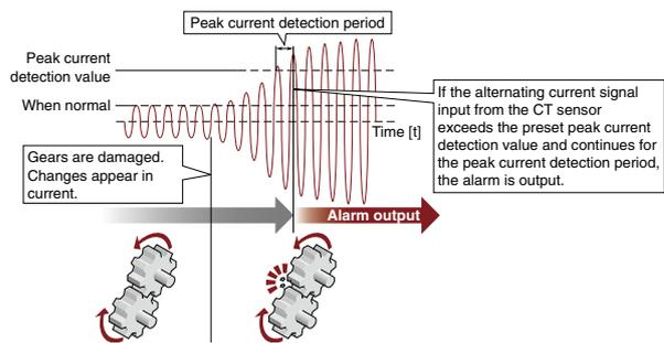
Input signal error detection function
