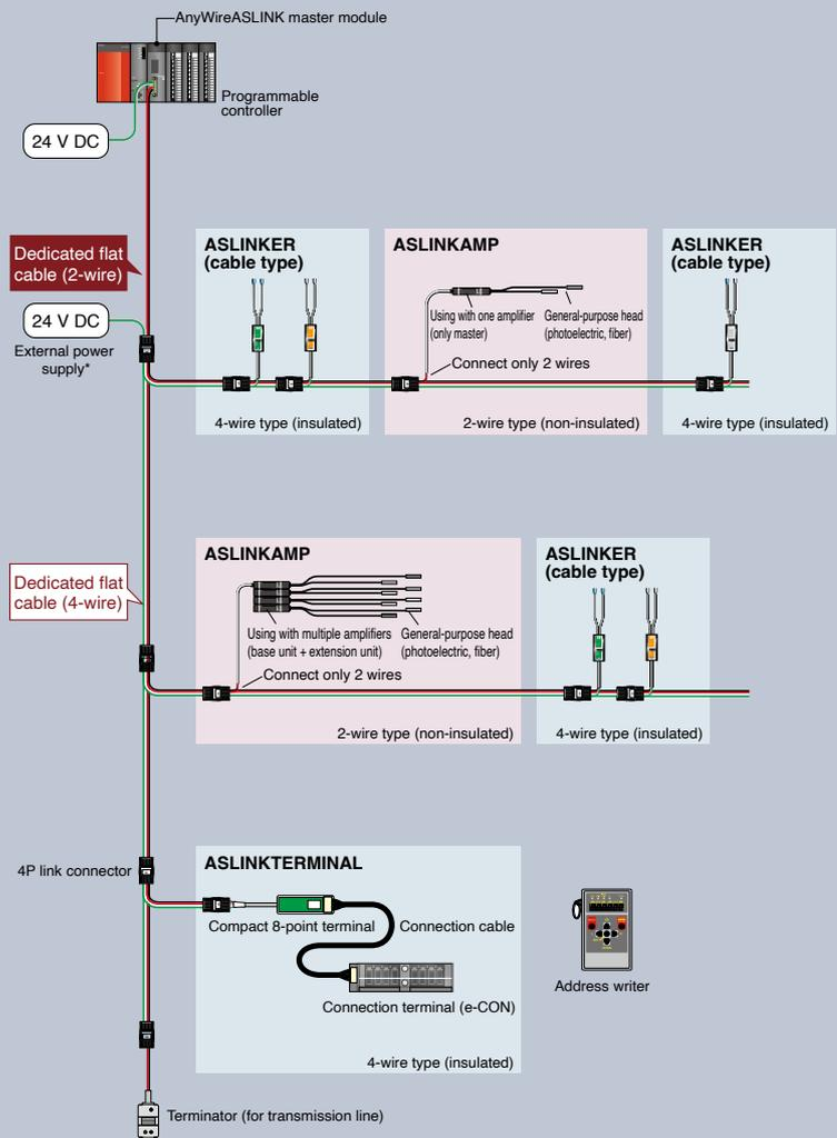
\* External power for 4-wire type wiring.
