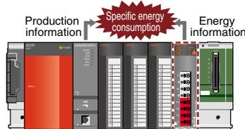
\*3. The specific energy consumption is a numerical value displayed by “dividing energy consumption by production volume,” which is one type of index that measures energy productivity. Improving this number leads to improved productivity and energy conservation.
