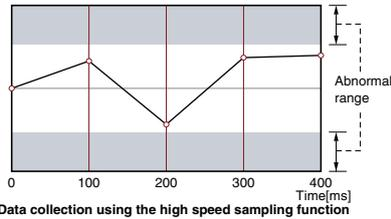
The high speed data logger module is capable of sampling data at much higher intervals as to detect fast changing values. (fastest down to 1 ms)
