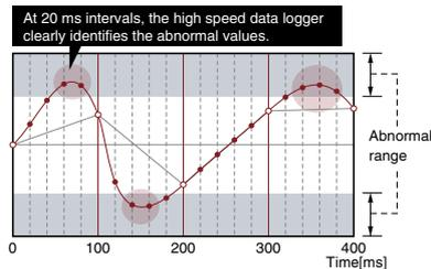
**CPUs that support the high speed data sampling function**
