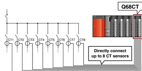
**Predictive maintenance of devices by detecting the peak current.**
