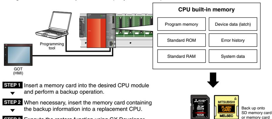
**STEP 1** Insert a memory card into the desired CPU module and perform a backup operation.
