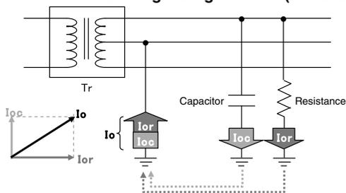
$I_{or}$ : Leakage current caused by insulation deterioration (resistive component in the leakage current)
