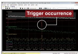
By only saving data immediately before and after a trigger occurrence, the search for problems and their causes is made highly efficient.
