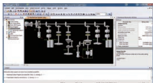
Programming screen using mechanical system program
