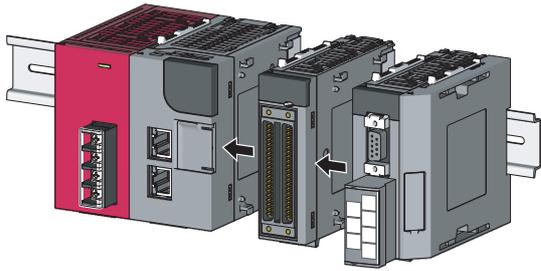
**7. Lock the module joint levers.**
