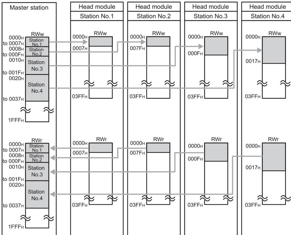
The data flow between the master station and the head module (station number 1) is shown in Page 73, Section 8.2 (1) (a).
