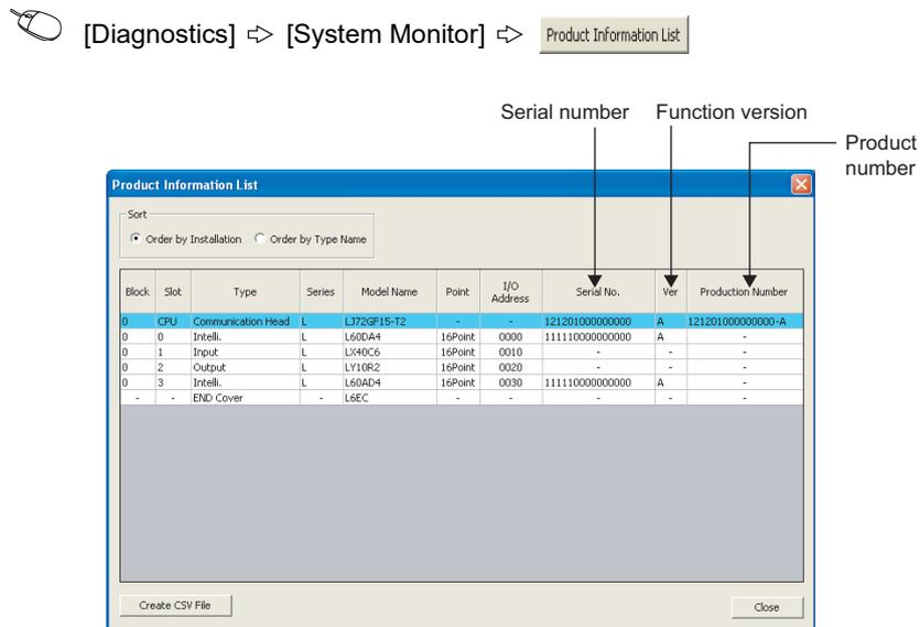
On the window, the serial number and function version of each intelligent function module can be checked as well.
