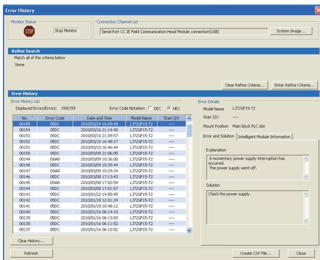
3. Check the error that has occurred before the head module is reset or the system is powered off in the "Error History" window.
