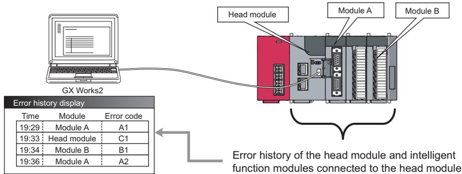
Error history of the head module and intelligent function modules connected to the head module
