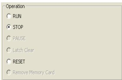
4. Select a remote operation to the head module in "Operation".
