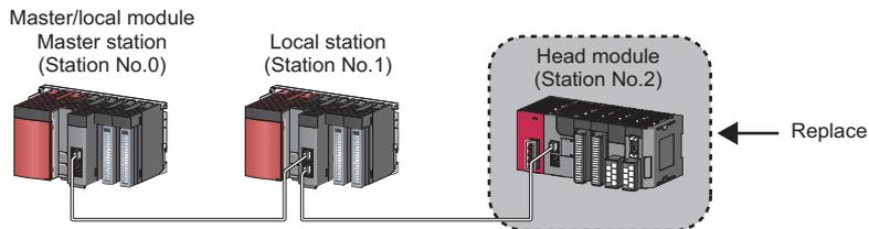
5. If the new head module does not have a station number, connect GX Works2 to the master station, and assign a station number to the head module from the CC-Link IE Field Network diagnostics.
