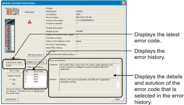
2. Check the error that has occurred before the head module is reset or the system is powered off in the "Error History" window.
