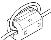
**(b) Noise filter (power supply line filter)**
