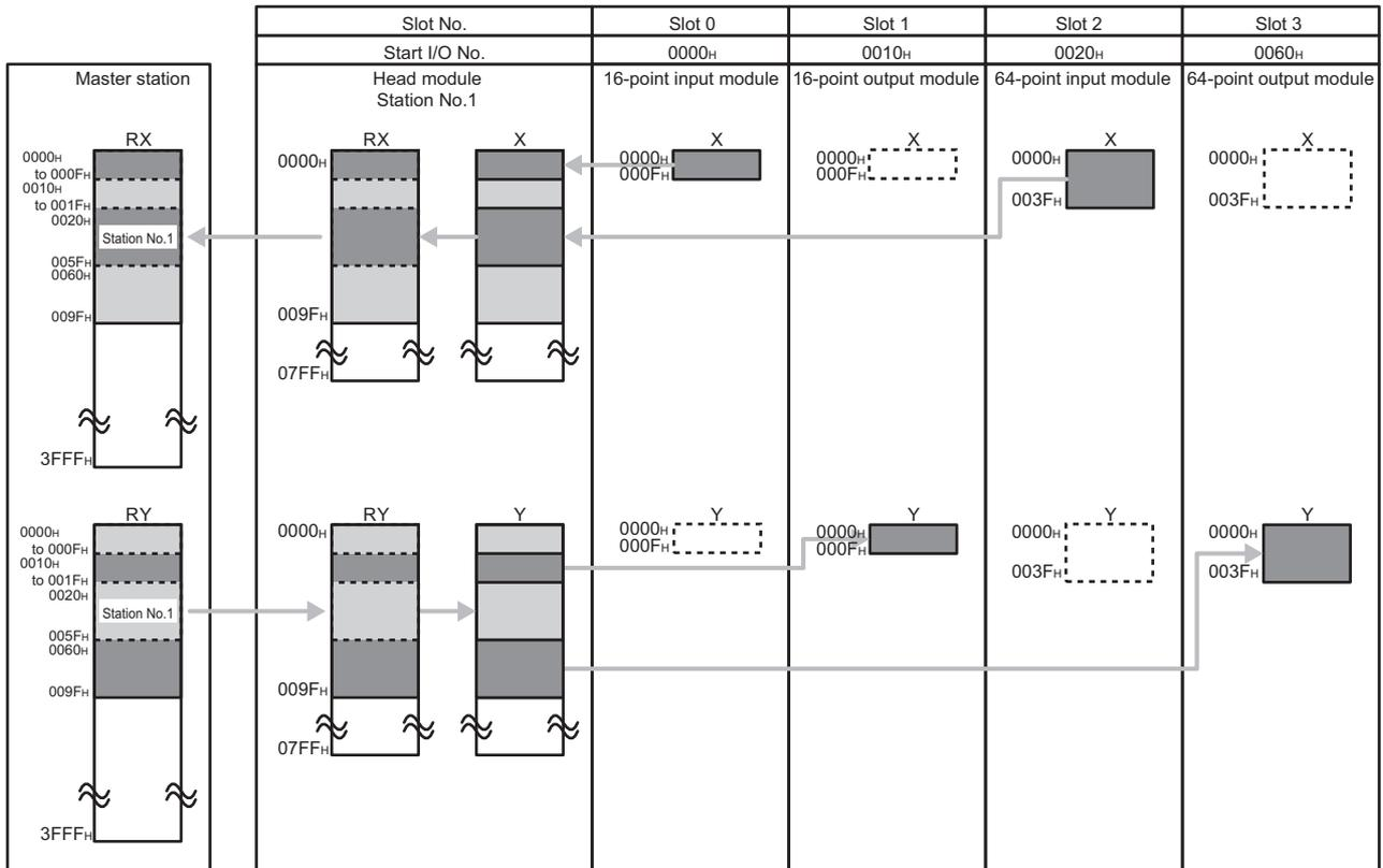
**(b) Data flow when "0000H" is set to the start number of RX/RX of the master station and the I/O assignment setting for the head module is changed**
