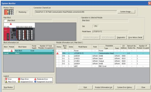
1. Connect GX Works2 to the head module, and open the "System Monitor" window.
