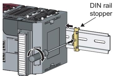
**5. Hitch the bottom hook of the DIN rail stopper to the bottom of the DIN rail.**
