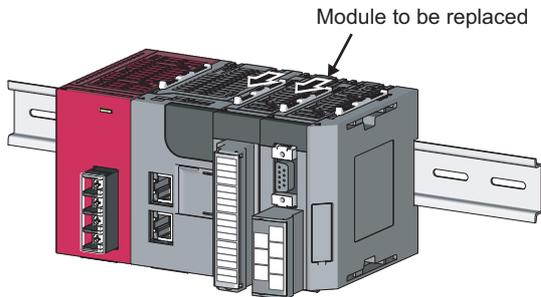
3. Release the module joint levers on the modules.
