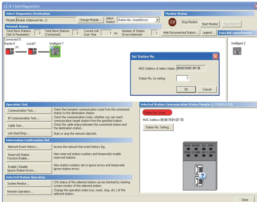
6. Write the parameters read in step 1 to the new head module.
