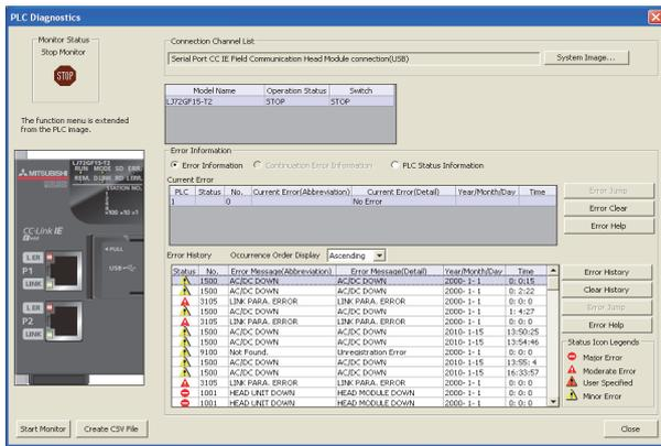
1. Select the head module in the "System Monitor" window and click the **Diagnostics** button to open the "PLC Diagnostics" window.
