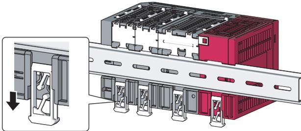
1. Remove the DIN rail stopper on the right side.
