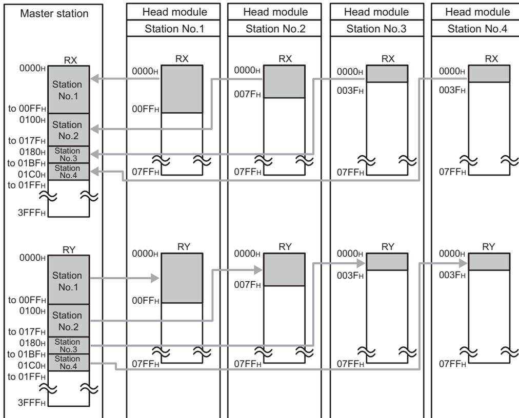
The I/O data flow between the master station and the head module (station number 1) is shown in Page 67, Section 8.1 (1) (a) and Page 68, Section 8.1 (1) (b).
