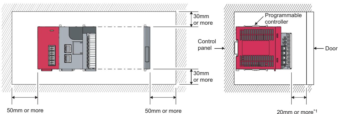
\*1 When using connectors for external devices, provide clearance of 80mm or more.
