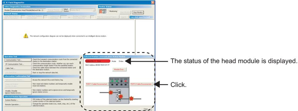
**4. Various tests and operations can be performed from "Operation Test" and "Selected Station Operation" on the bottom left of the window. (👉 Page 80, Section 9.4 to Page 81, Section 9.7)**
