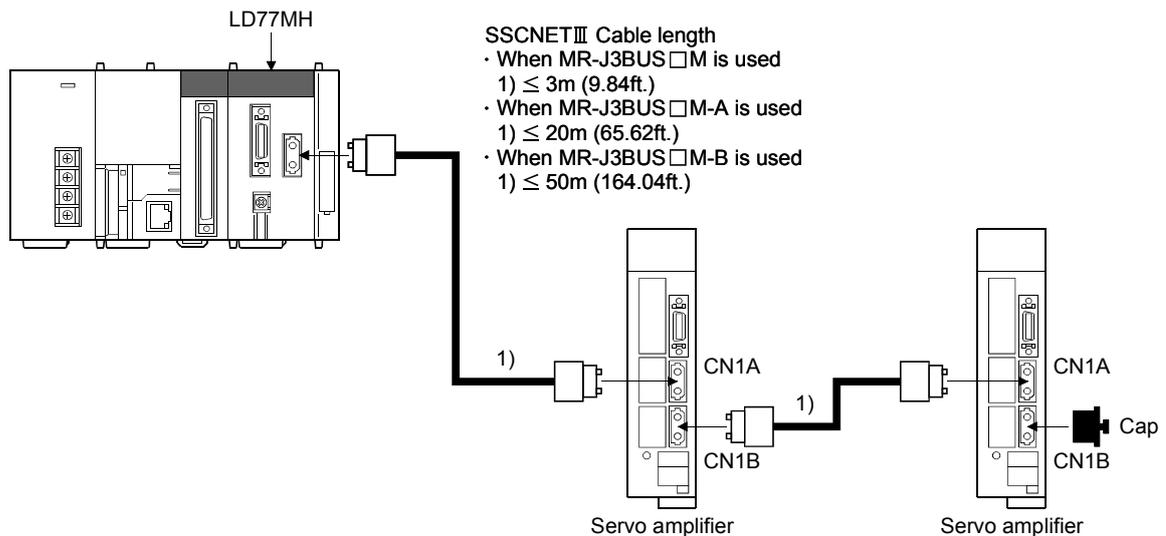
(Note): It cannot communicate with that the connection of CN1A and CN1B is mistaken.
