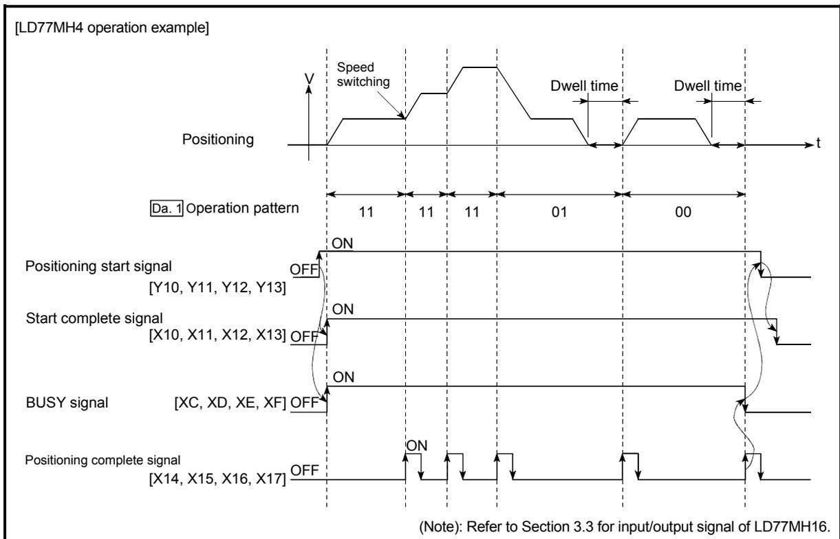
Fig. 9.4 Operation for the standard speed switching mode
