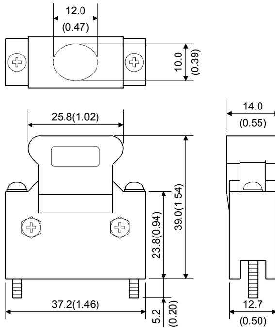
(c) Pressure-displacement type (Quick release metal latch type)
