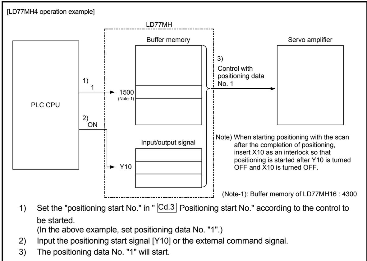
Fig. 6.2 Procedures for starting control (for axis 1)
