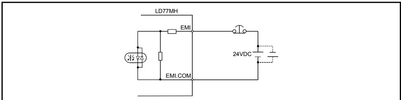
Fig. 13.21 Wiring when using the forced stop
