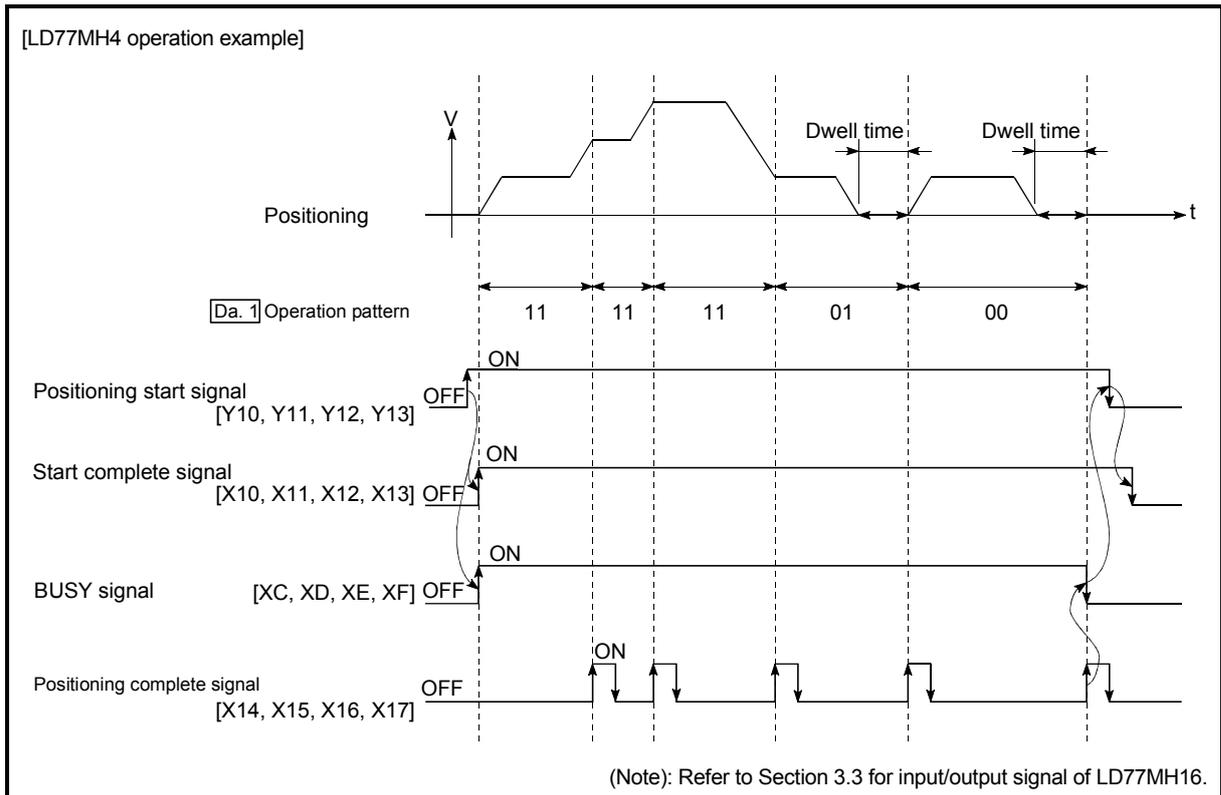
Fig. 9.5 Operation for the front-loading speed switching mode
