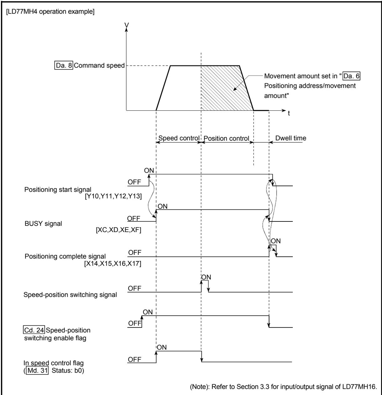
Fig. 9.13 Speed-position switching control (INC mode) operation timing
