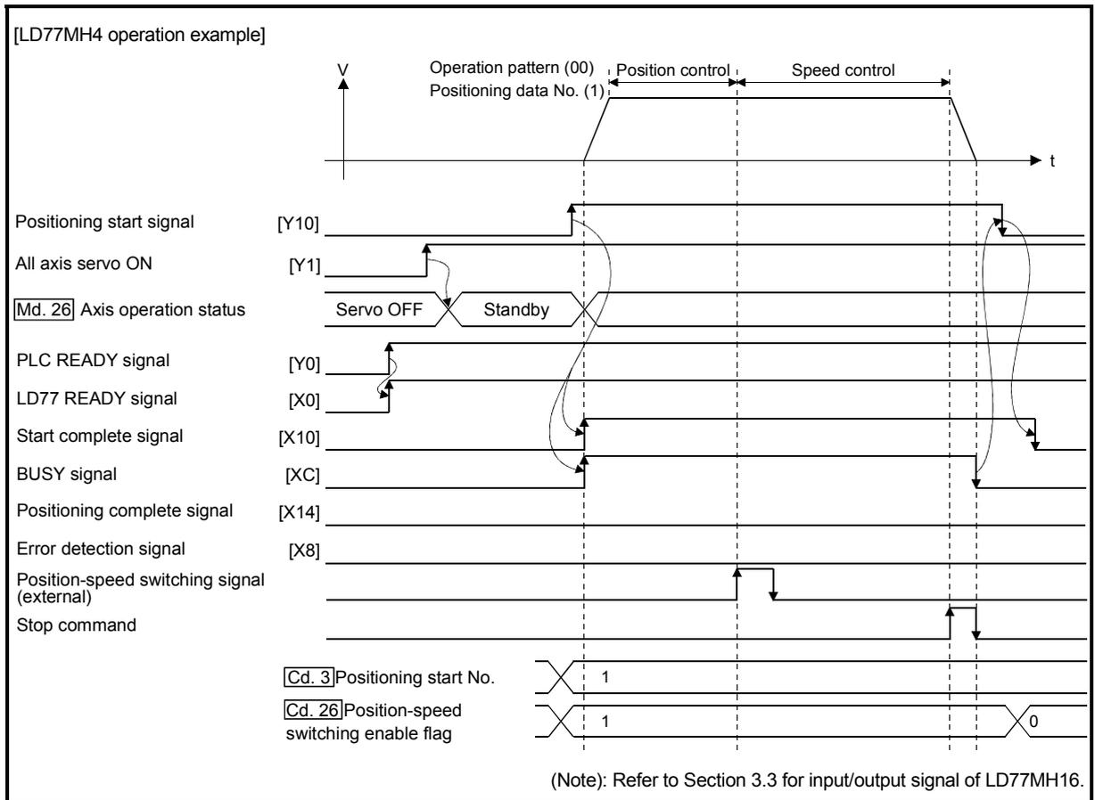
Fig. 6.8 Time chart for starting "position-speed switching control"
