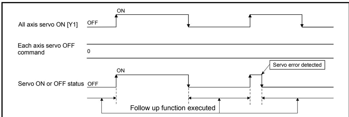
Fig. 13.54 Operation timings of follow up function
