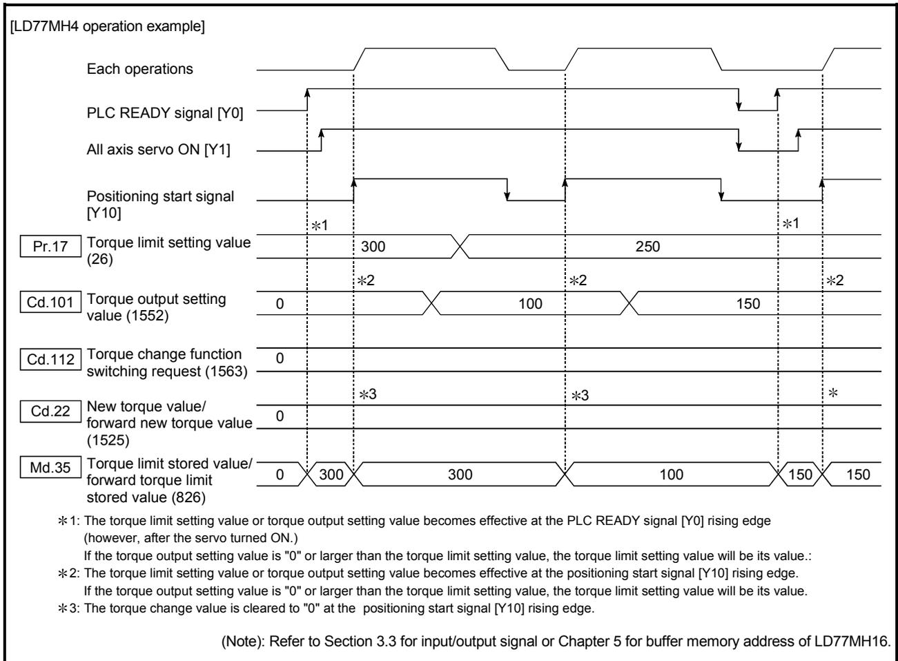
Fig. 13.11 Torque limit function operation
