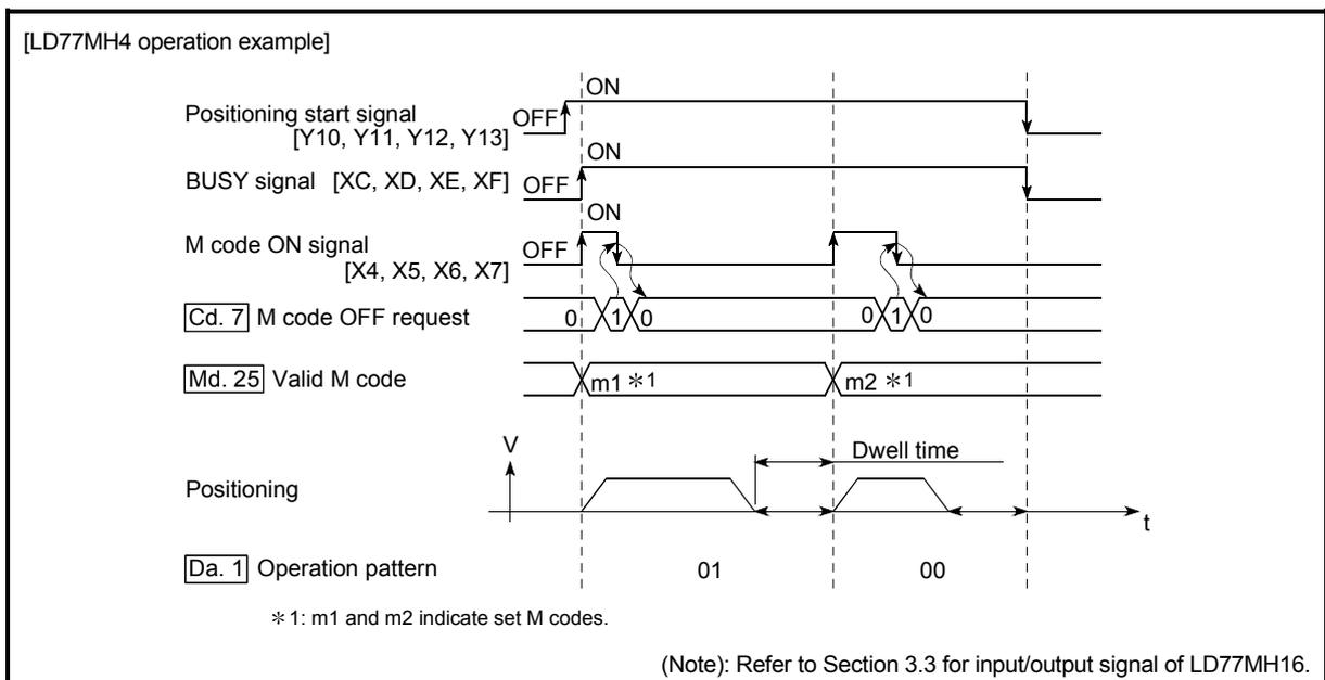
Fig. 13.40 M code ON/OFF timing (WITH mode)
