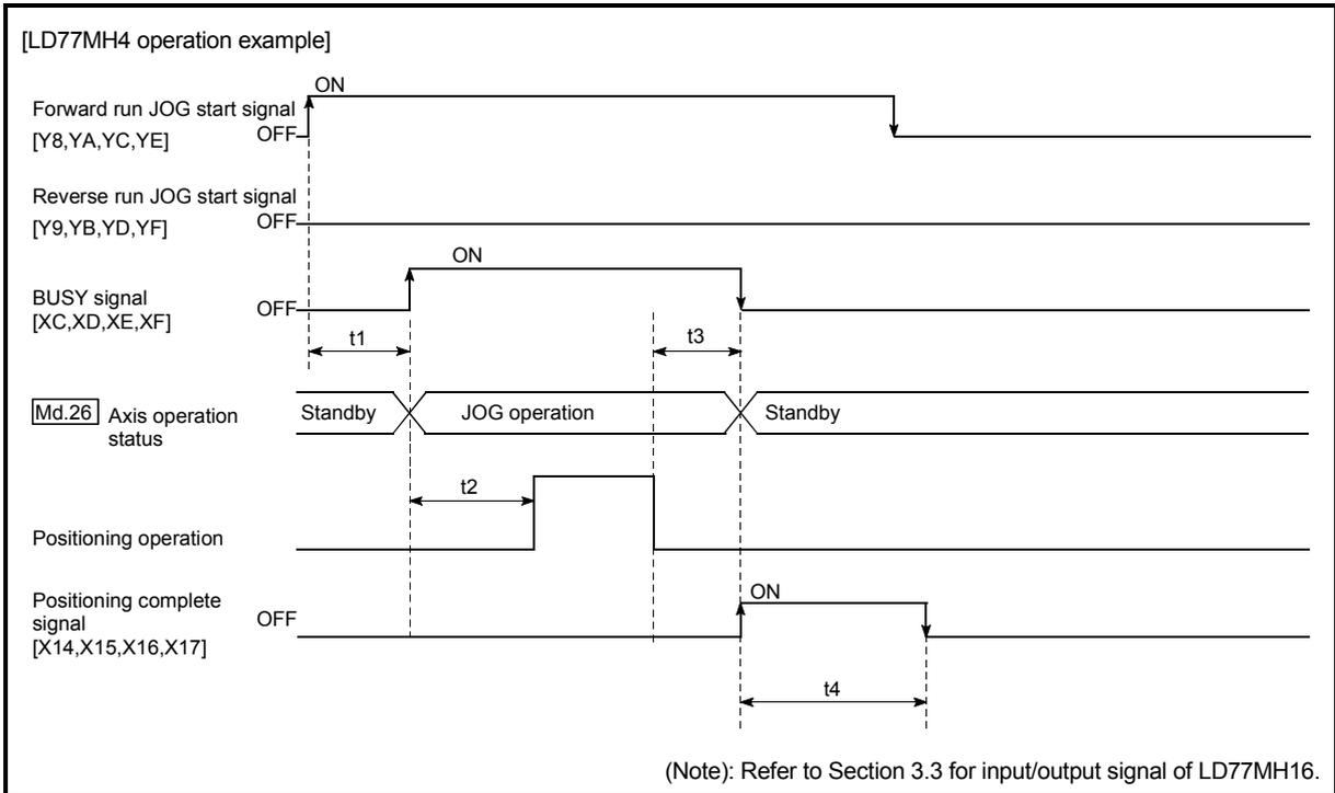
Fig. 11.12 Inching operation timing and processing times
