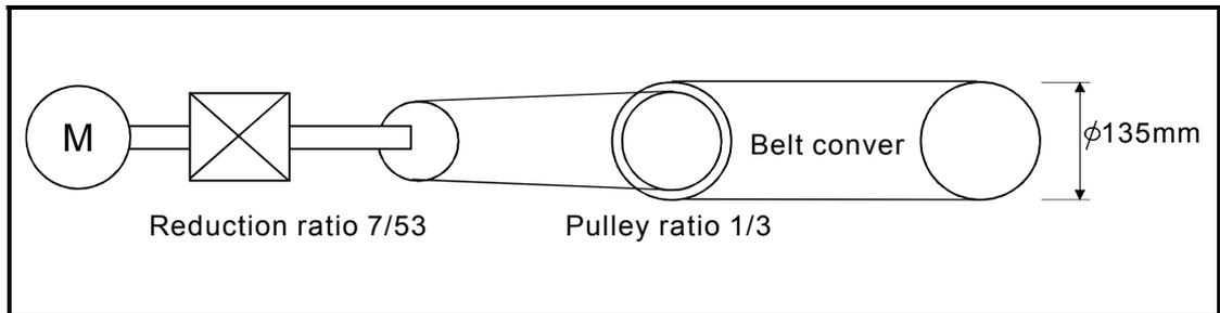
As the travel value of the conveyor is used to exercise control, set "mm" as the control unit.
