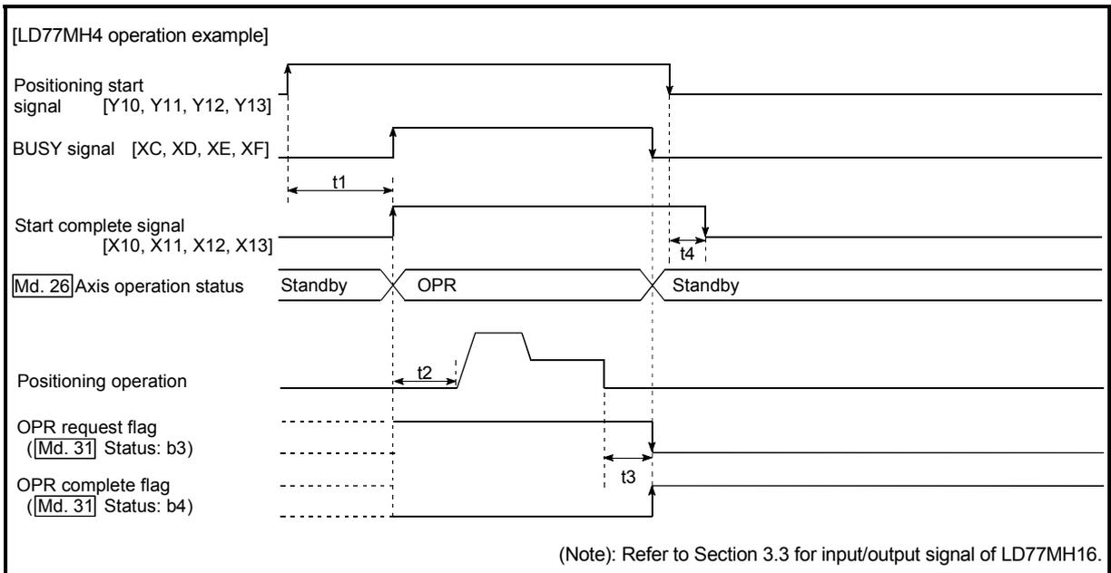
Fig. 6.9 Machine OPR operation timing and process time
