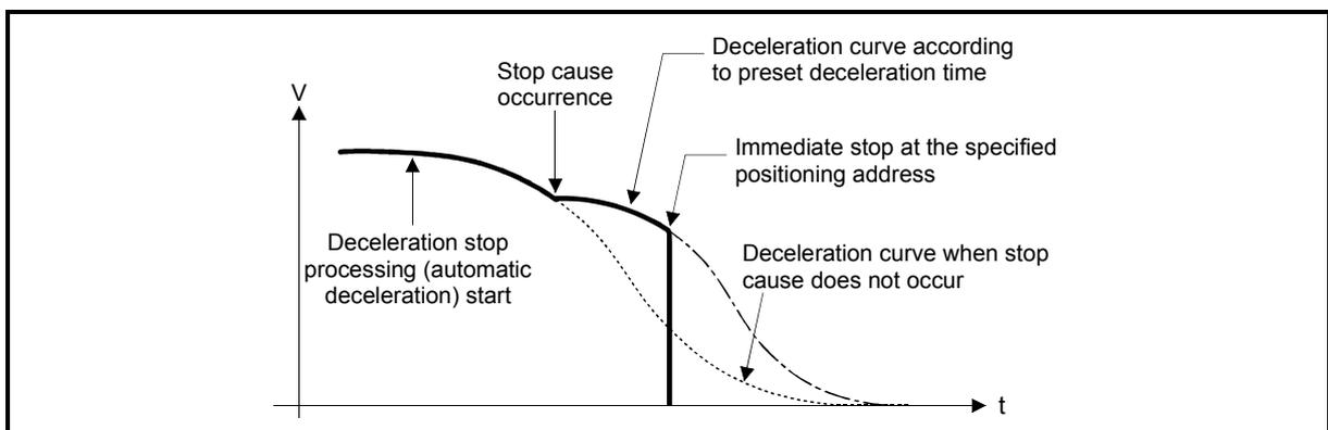
Fig. 13.51 Deceleration curve re-processing operation (for position control or S-curve acceleration/deceleration processing)
