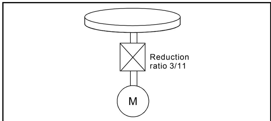
First, find how many degrees the load (machine) will travel ( $\Delta S$ ) when the motor turns one revolution (AP).
