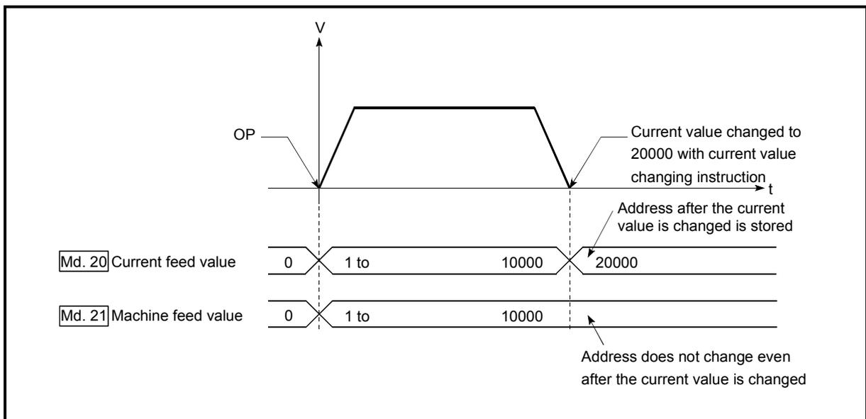
Fig. 9.8 Current feed value and machine feed value
