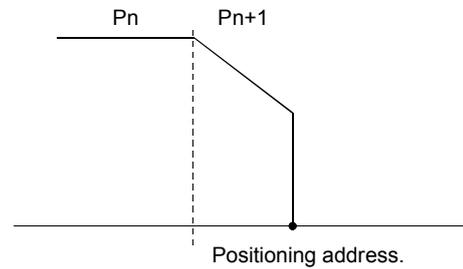
(b) Front-loading speed switching mode
