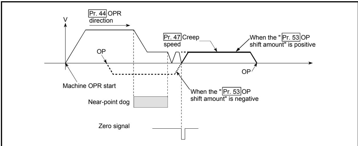
Fig. 13.7 OP shift operation at the creep speed
