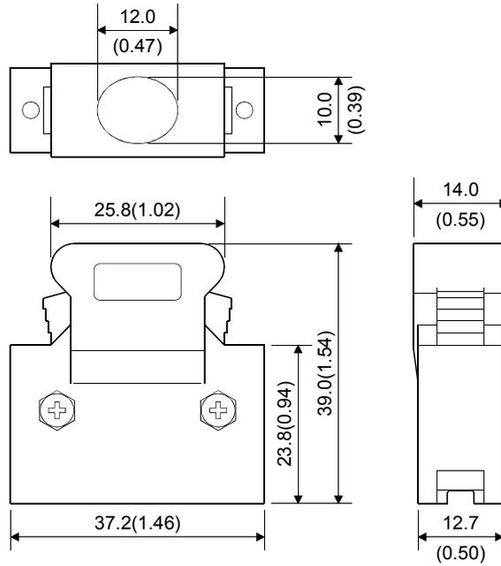
(b) Soldering type (Threaded type)
