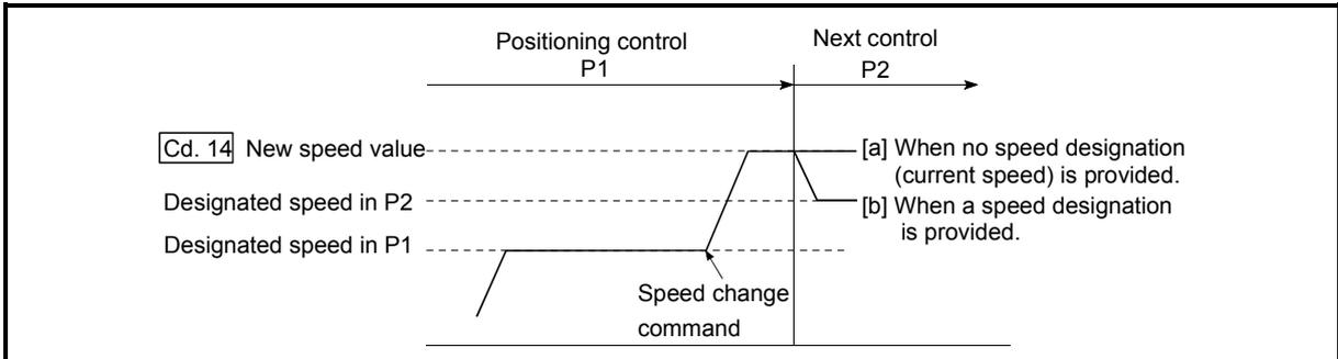
Fig. 13.23 Speed change during continuous path control
