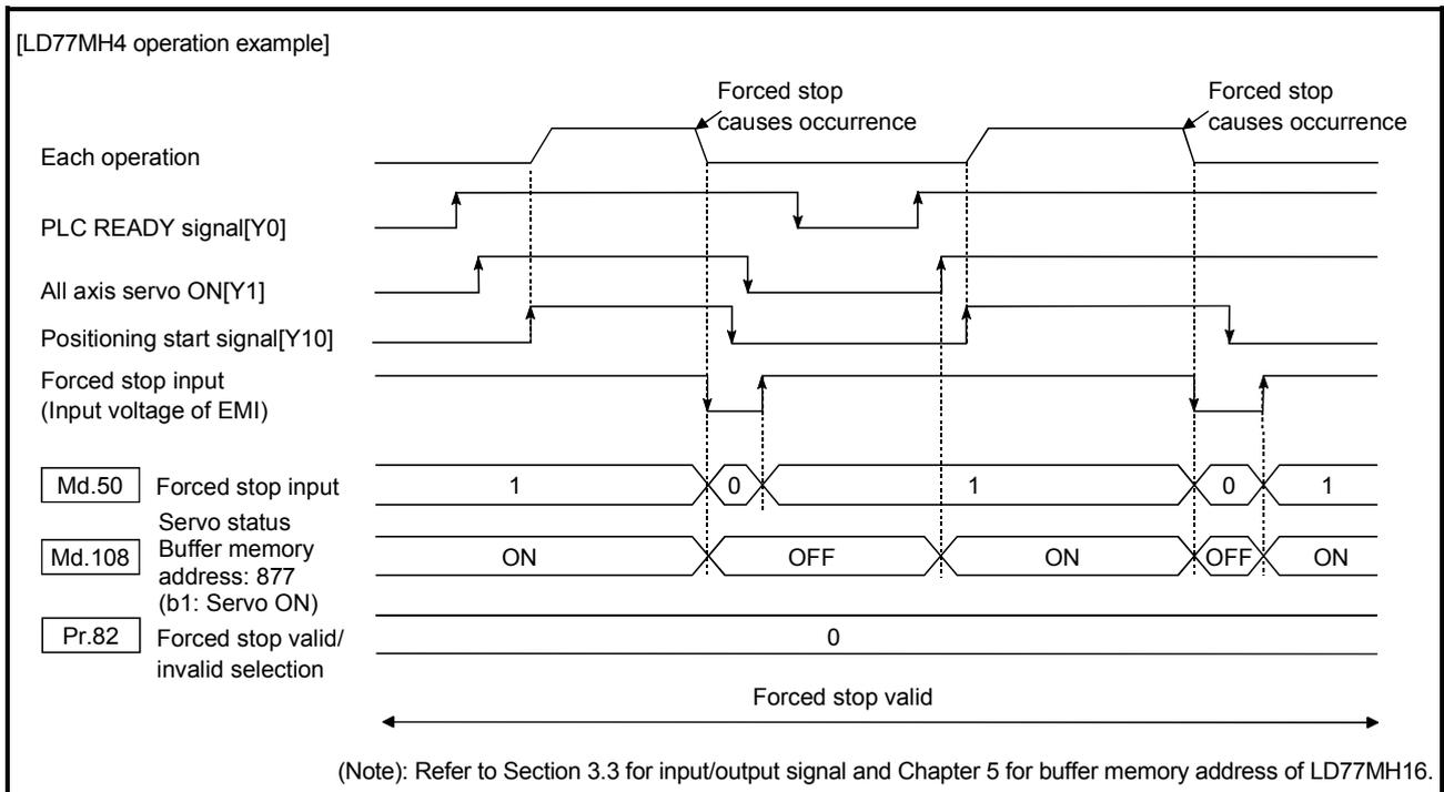
Fig. 13.20 Operation for the forced stop function
