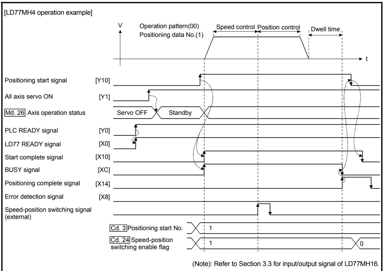
Fig. 6.7 Time chart for starting "speed-position switching control"
