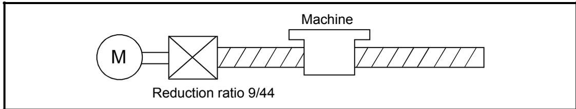
First, find how many millimeters the load (machine) will travel ( $\Delta S$ ) when the motor turns one revolution (AP).
