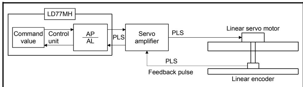
Calculate the number of pulses (AP) and movement amount (AL) for the linear encoder in the following conditions.
