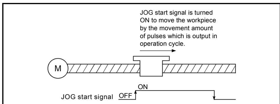
Fig. 11.2 Inching operation
