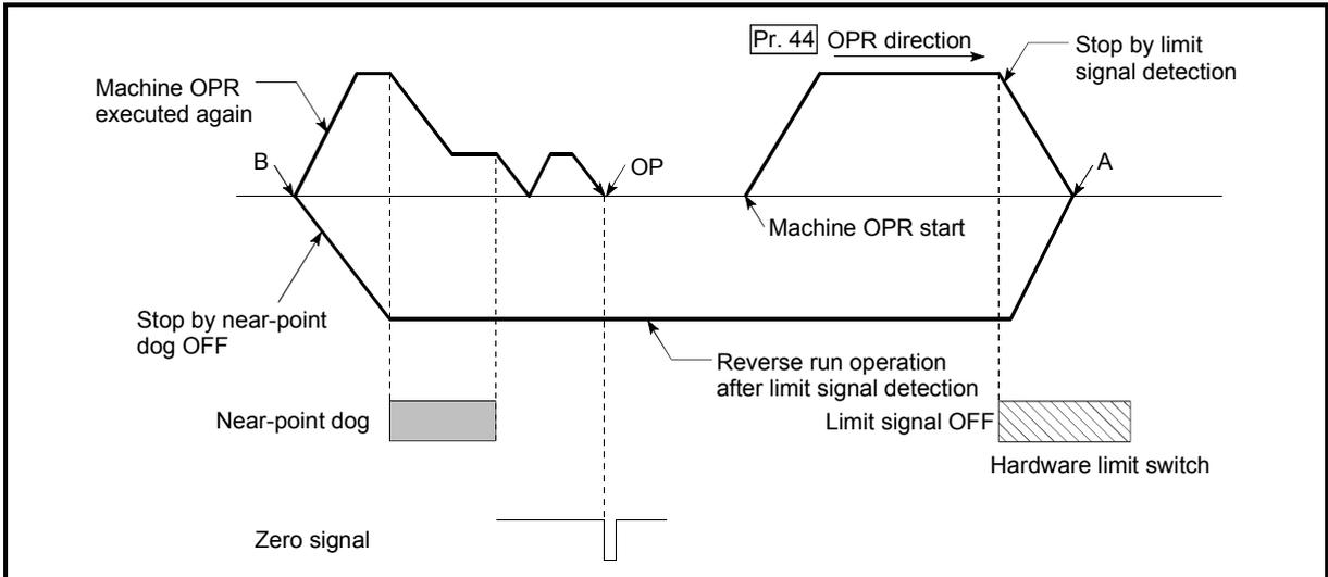
Fig. 13.3 Setting the dwell time during an OPR retry
