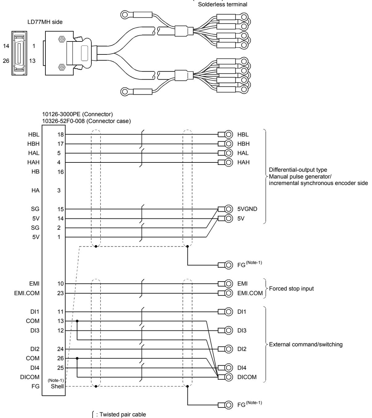
(Note-1): Ground FG terminal on the used equipment side. Also, connect it to the shell of connector side.
