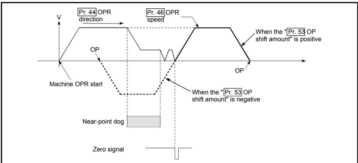
Fig. 13.6 OP shift operation at the OPR speed
