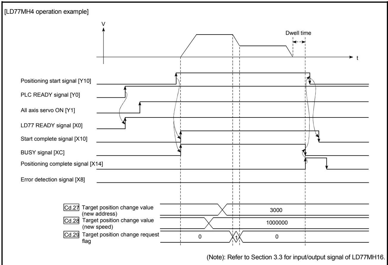
Fig. 13.34 Time chart for target position change from PLC CPU
