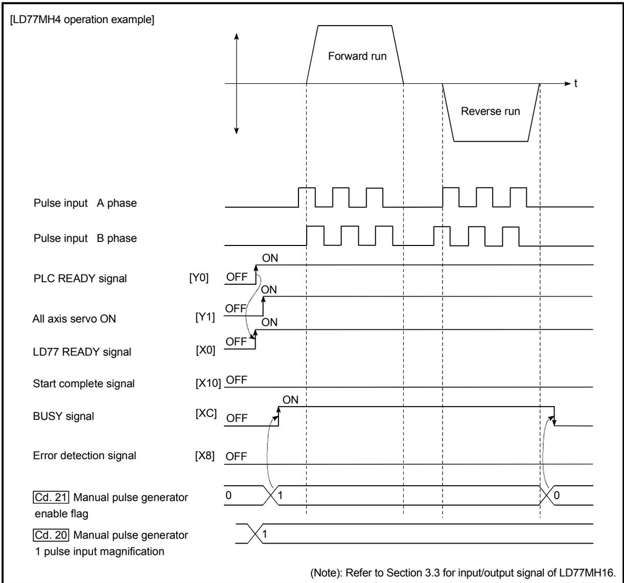
Fig. 11.18 Manual pulse generator operation start time chart
