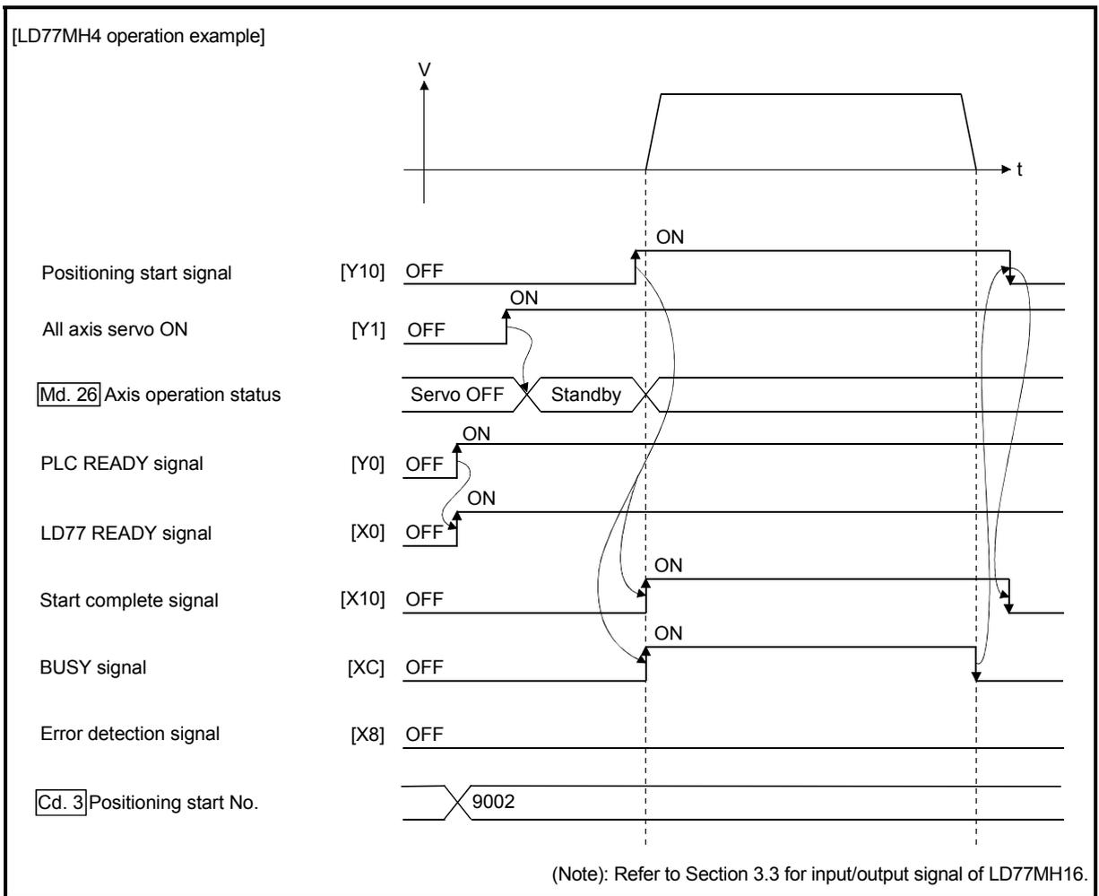
Fig. 6.5 Time chart for starting "fast OPR"
