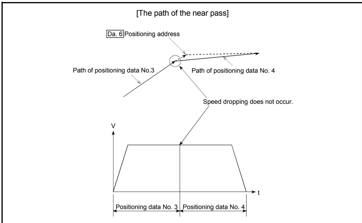
Fig. 13.9 The path of the continuous path control
