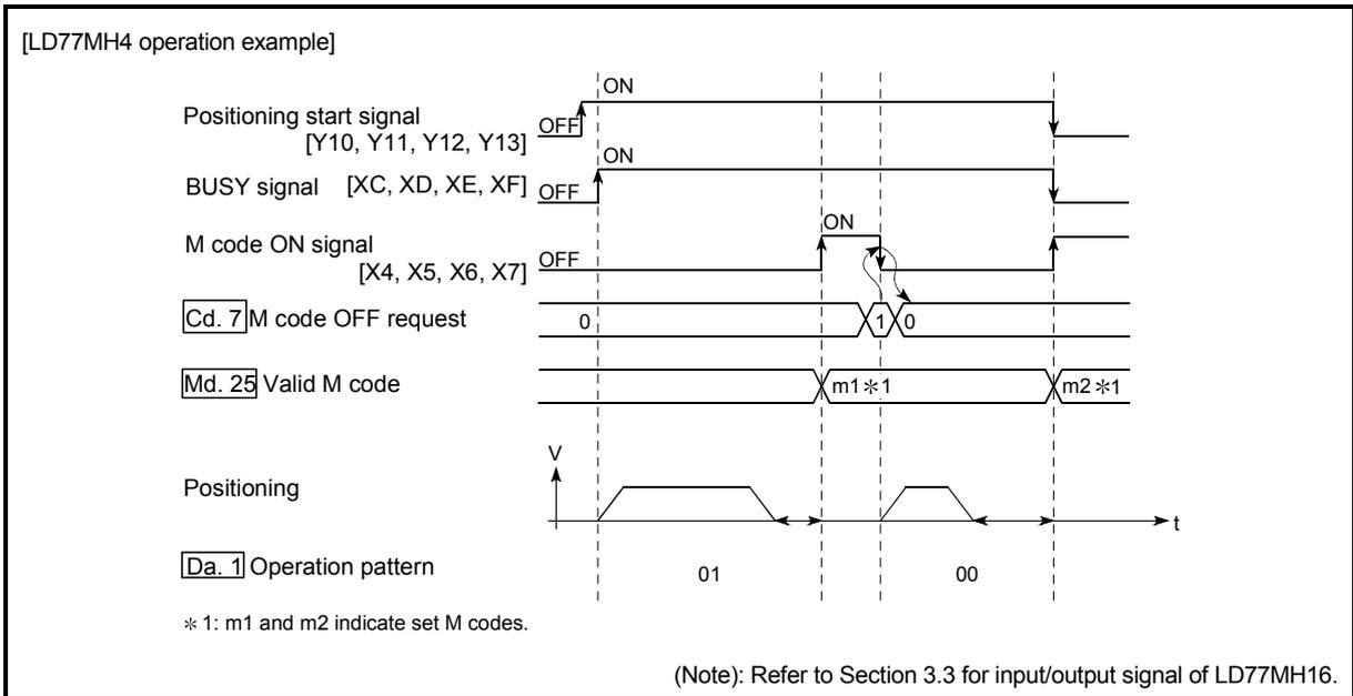
Fig. 13.41 M code ON/OFF timing (AFTER mode)
