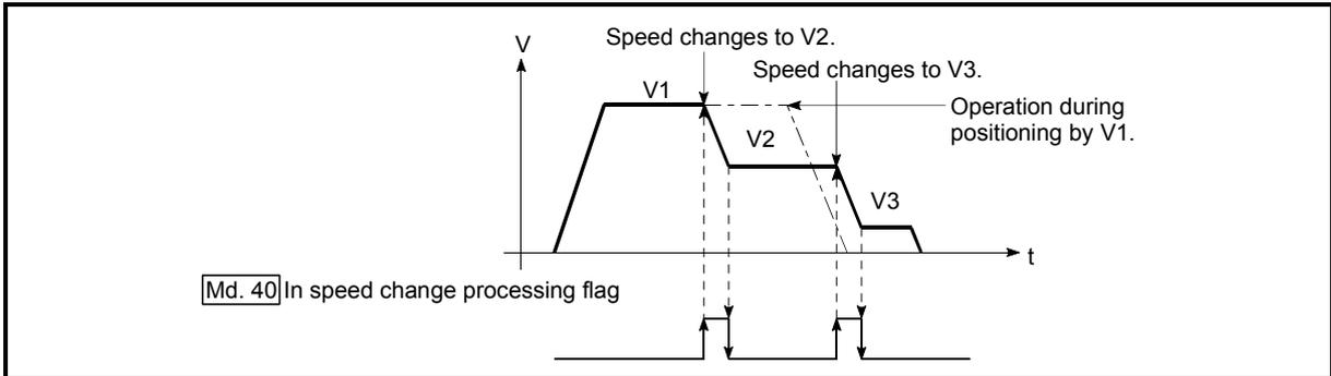
Fig. 13.22 Speed change operation
