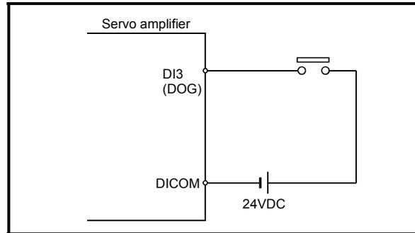
Fig. 8.1 Wiring when using the near-point dog
