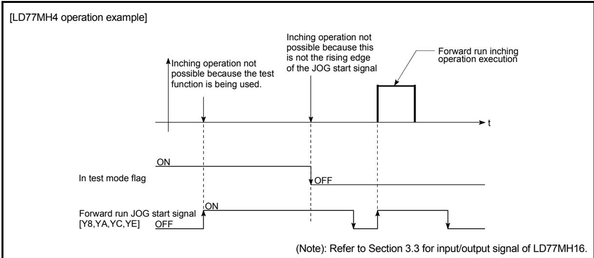
Fig. 11.15 Operation when the JOG start signal is turned ON while the test function is used
