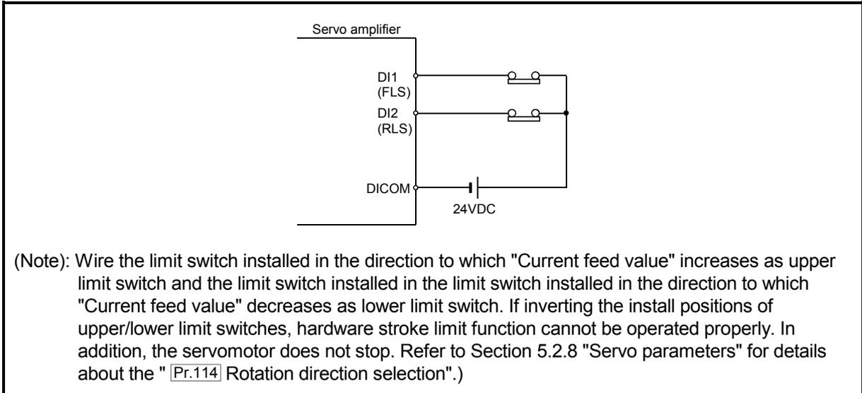
Fig. 13.18 Wiring when using the hardware stroke limit
