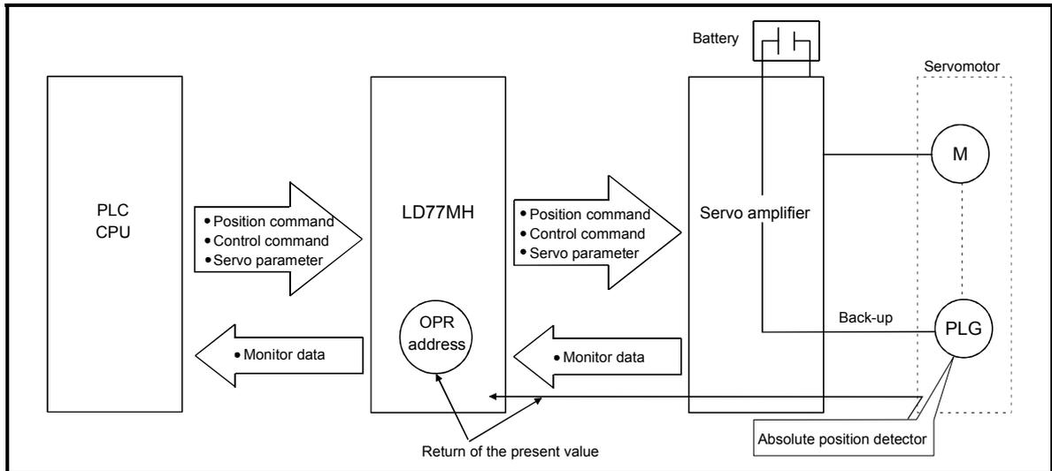
Fig. 13.35 Configuration of absolute position system
