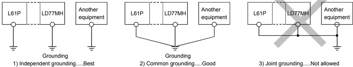
(c) For grounding a cable, use the cable of AWG16 to AWG20 (1.31 to 0.517mm<sup>2</sup>).
