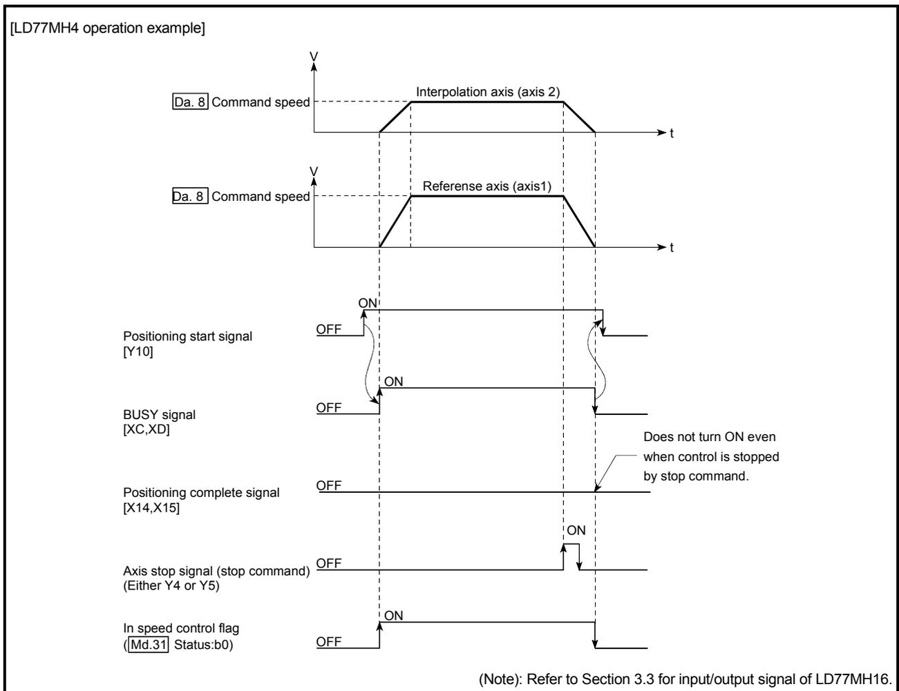
Fig. 9.10 2-axis speed control operation timing
