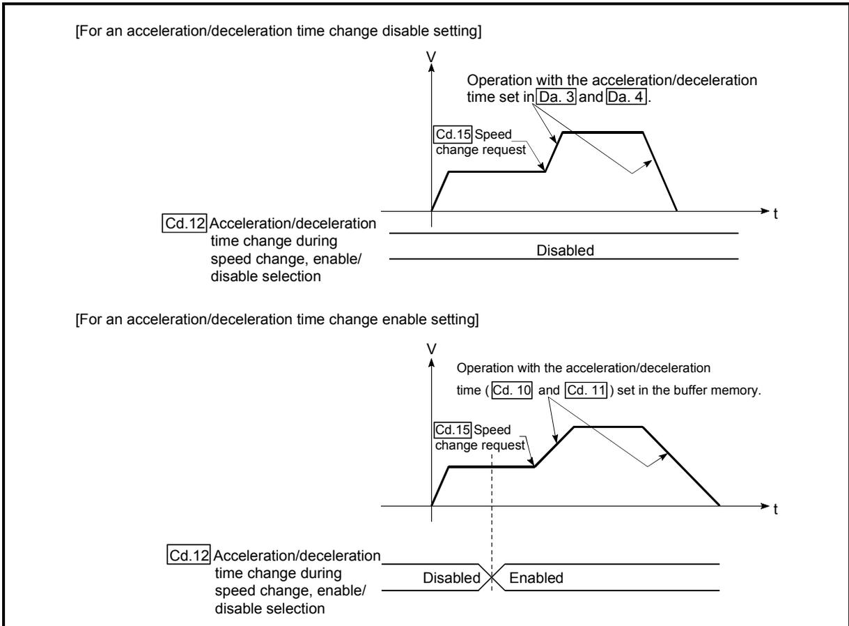
Fig. 13.30 Operation during an acceleration/deceleration time change
