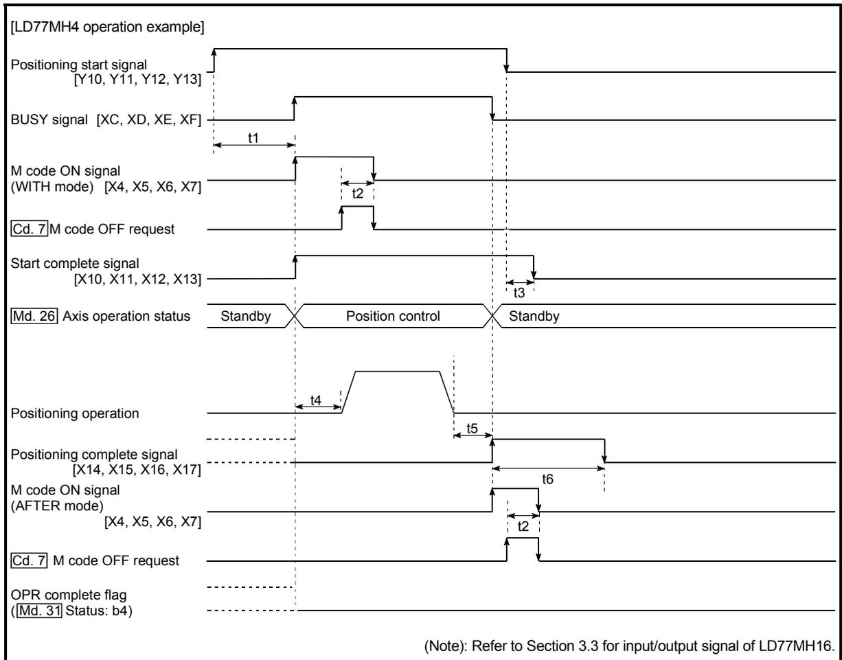
Fig. 6.10 Position control operation timing and process time
