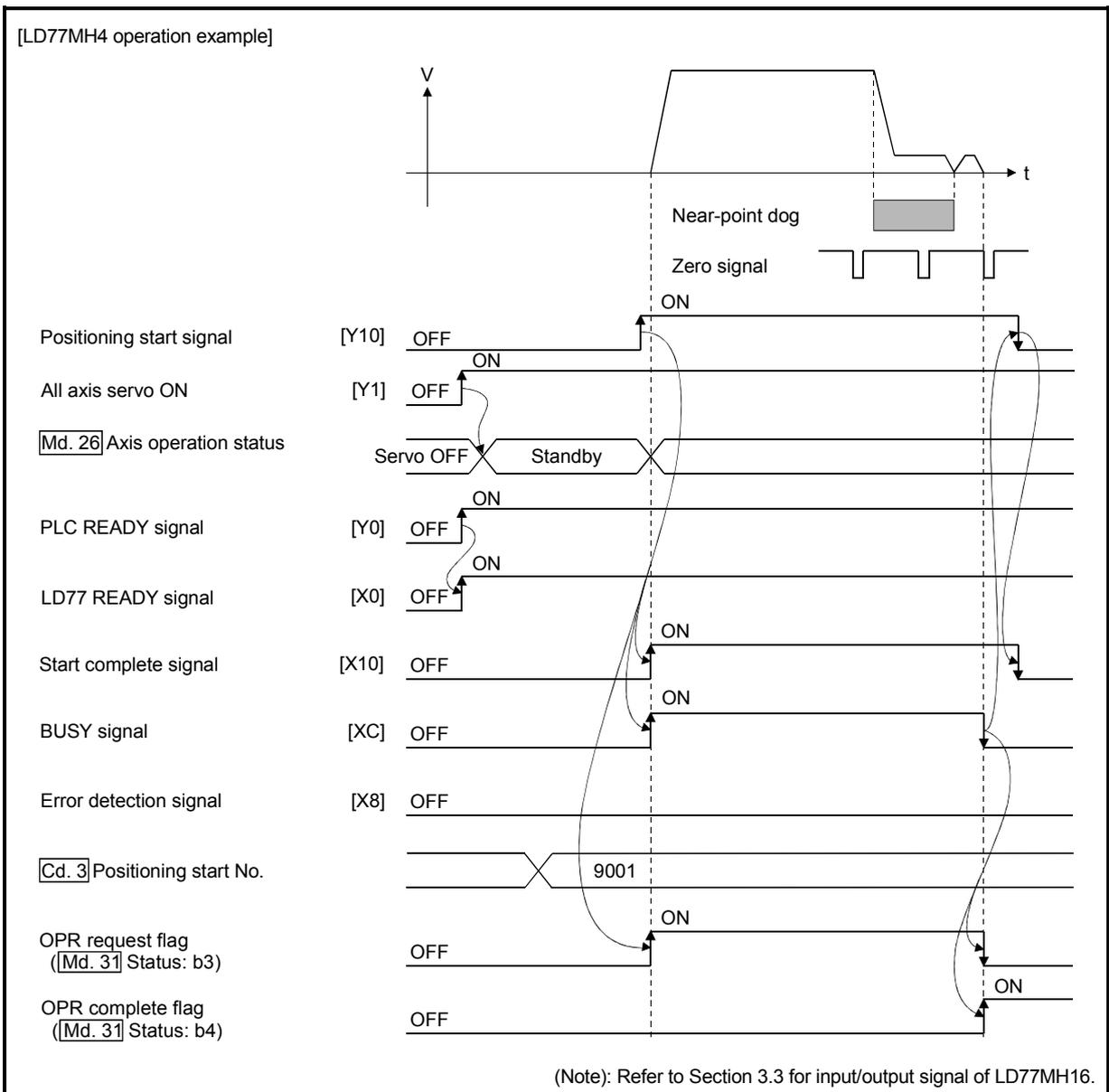
Fig. 6.4 Time chart for starting "machine OPR"
