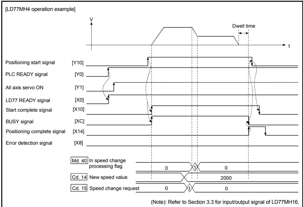
Fig. 13.26 Time chart for changing the speed from the PLC CPU
