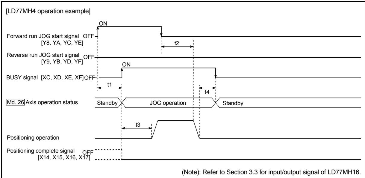
Fig. 11.5 JOG operation timing and processing times
