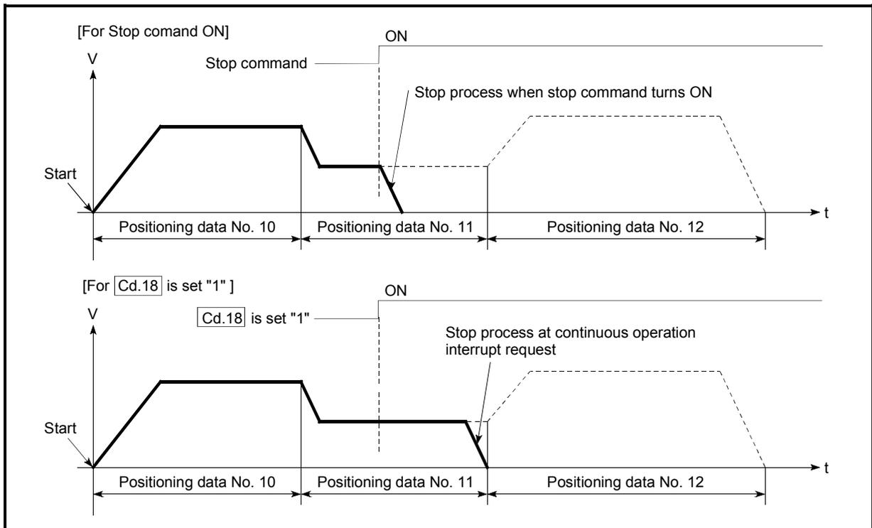
Fig. 6.12 Operation during continuous operation interruption
