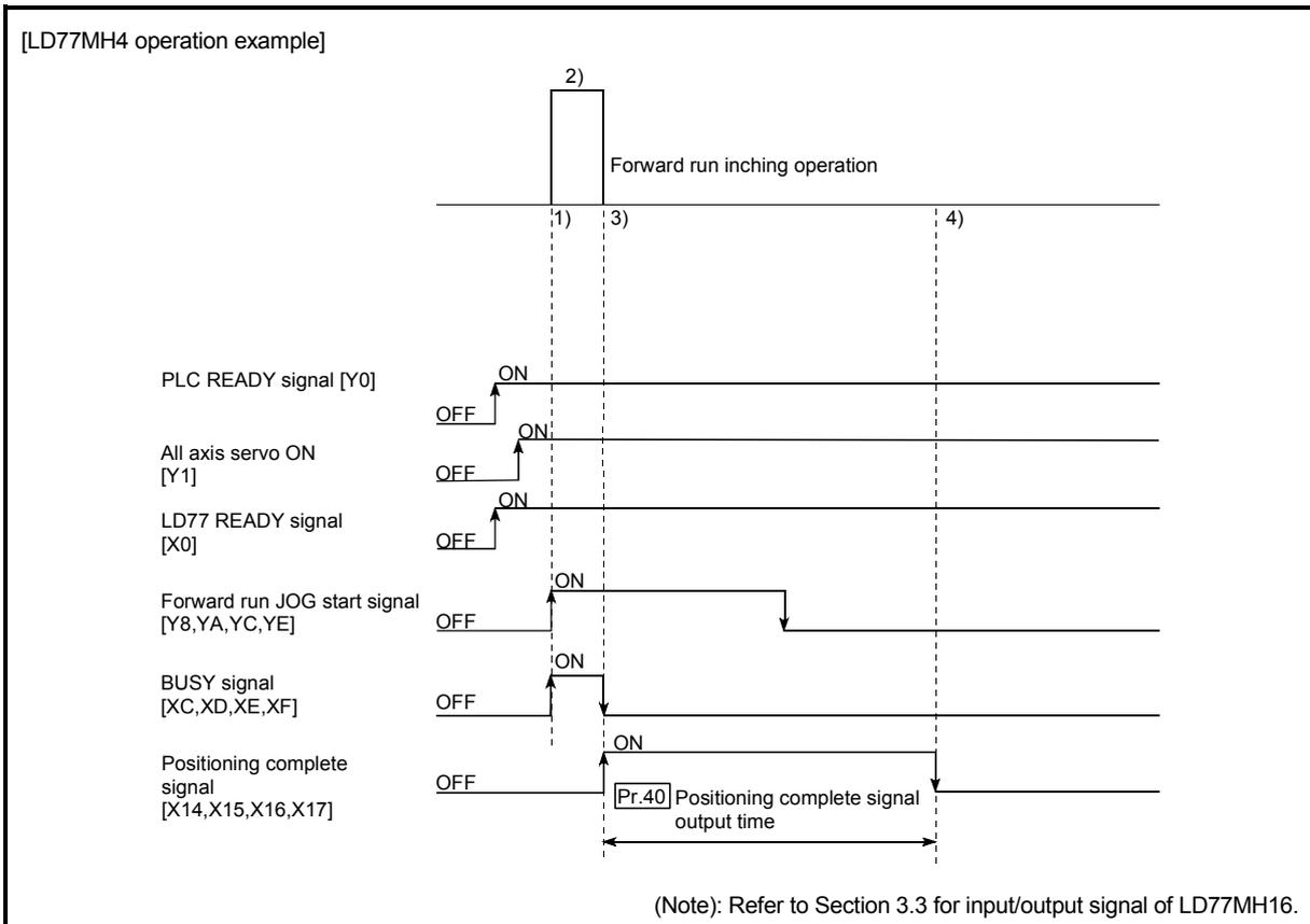
Fig. 11.11 Inching operation
