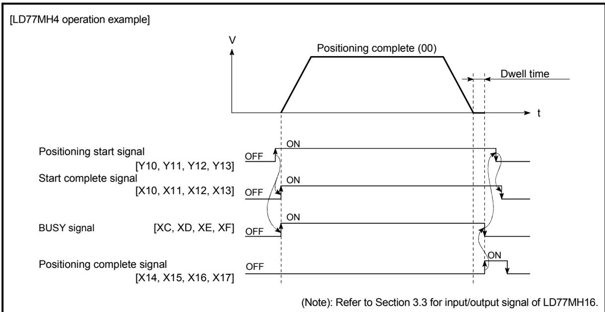
Fig. 9.1 Operation during independent positioning control
