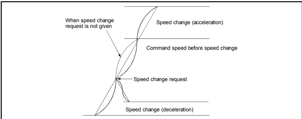
Fig. 13.47 Speed change during S-curve acceleration/deceleration processing
