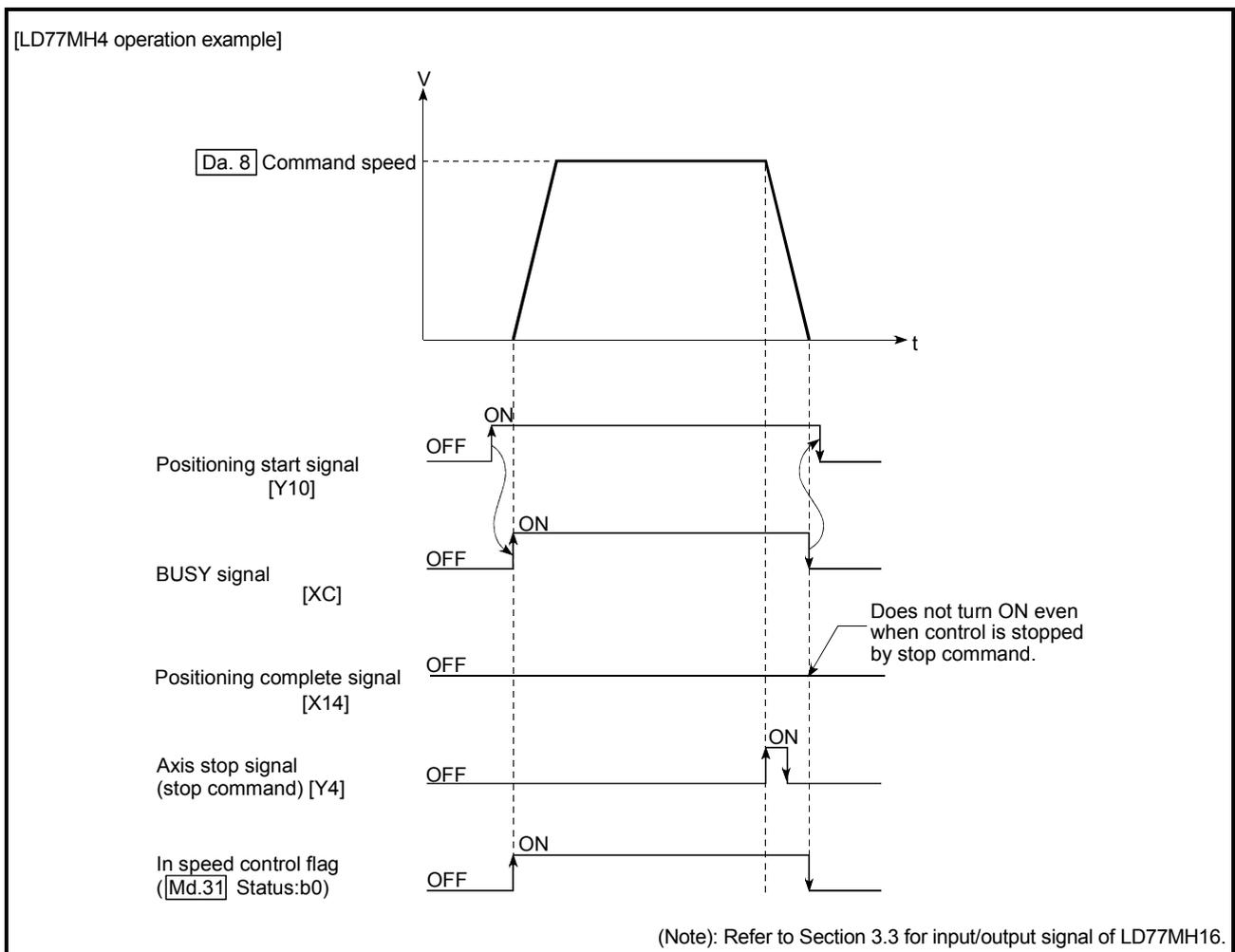
Fig.9.9 1-axis speed control operation timing
