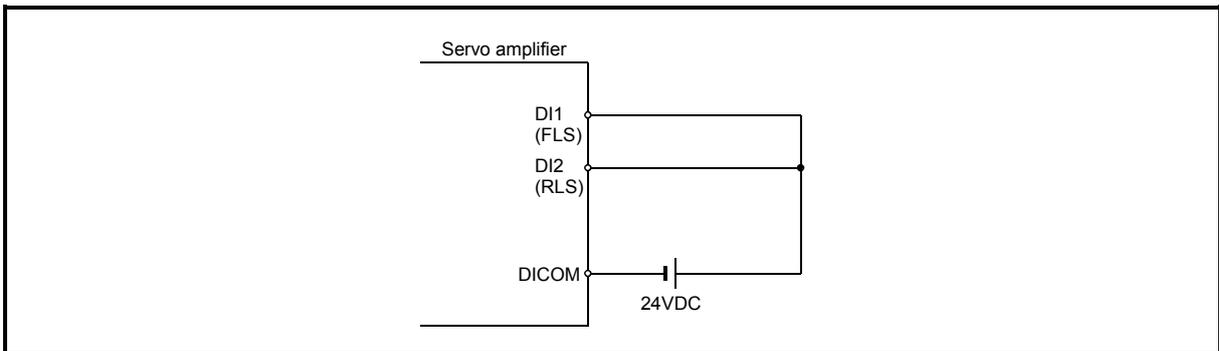
Fig. 13.19 Wiring when not using the hardware stroke limit function
