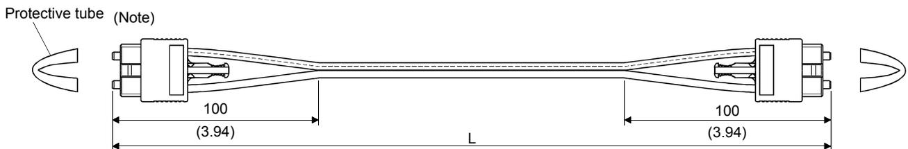
(Note): Dimension of connector part is the same as that of MR-J3BUS015M.
