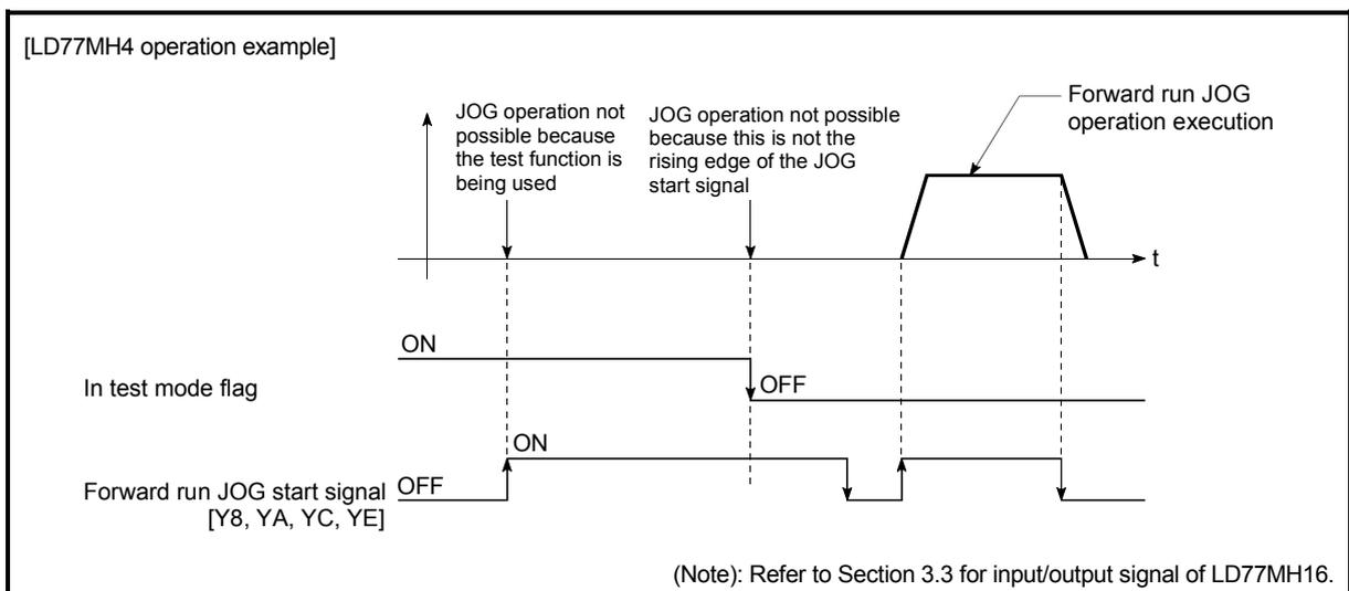
Fig. 11.10 Operation when the JOG start signal is turned ON while the test function is used
