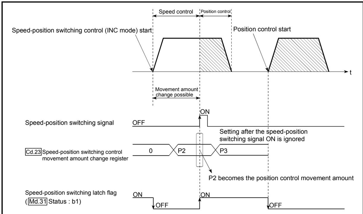
Fig. 9.15 Position control movement amount change timing
