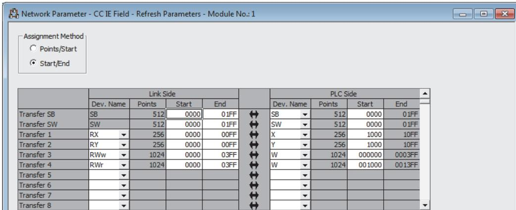
**5. Write the set parameter to the CPU module of the master station and reset the CPU module, or power off and on the programmable controllers.**
