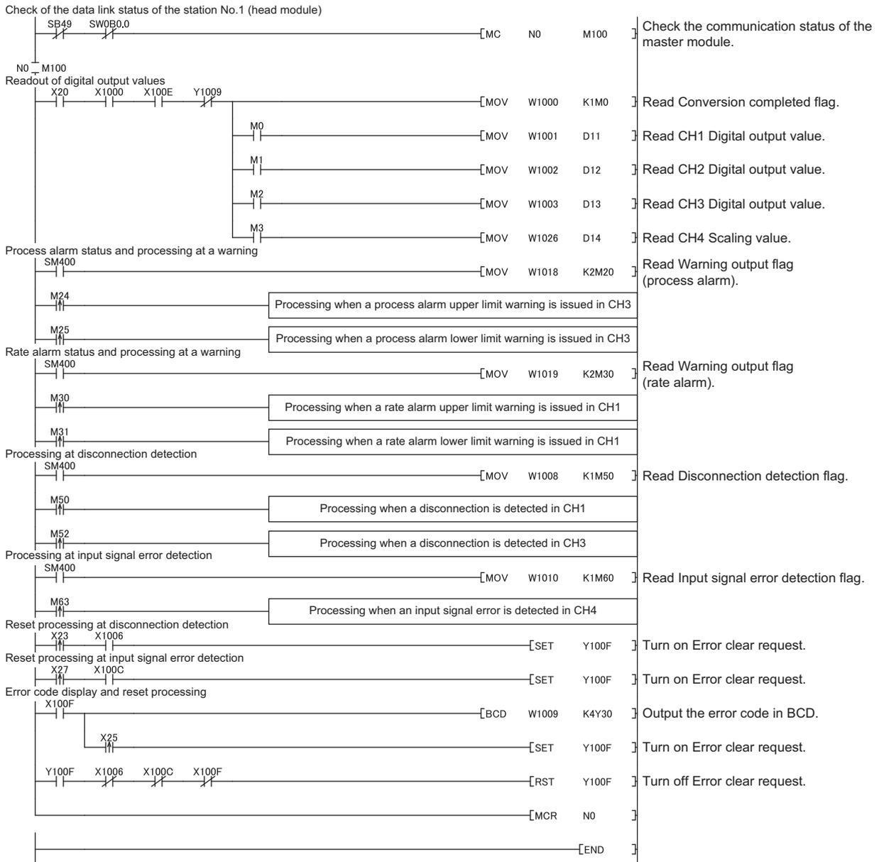
10.3 When a Multiple Input Module is Connected to a Head Module
