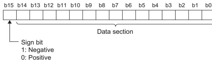
The data to be stored differs depending on the setting value of CH□ Input type/range setting (Un\G500 to Un\G503)
