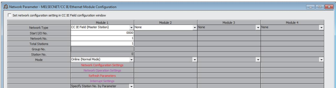
**3. Display the Network Configuration Settings window and configure the setting as follows.**
