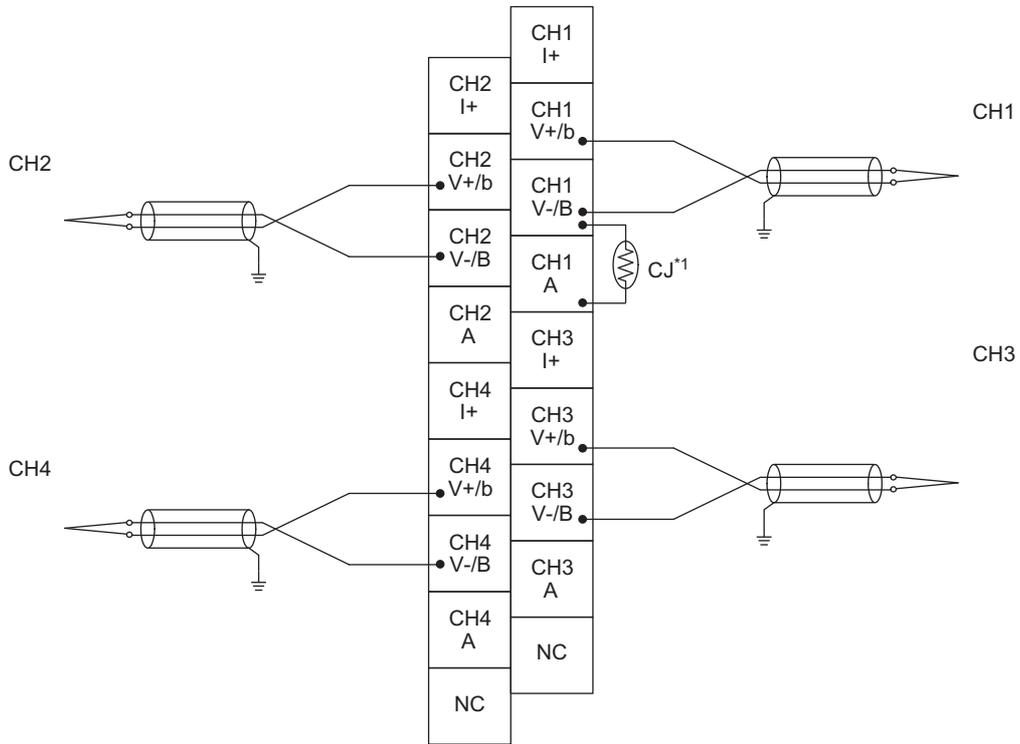
\*1 To use the thermocouple input, always connect the cold junction compensation resistor (CJ) supplied with the module between the CH1 V-/B terminal (pin number 5) and the CH1 A terminal (pin number 7).
