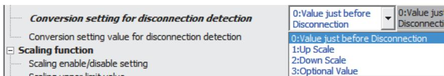
2. When "3: Optional Value" is set, set "Conversion setting value for disconnection detection".
