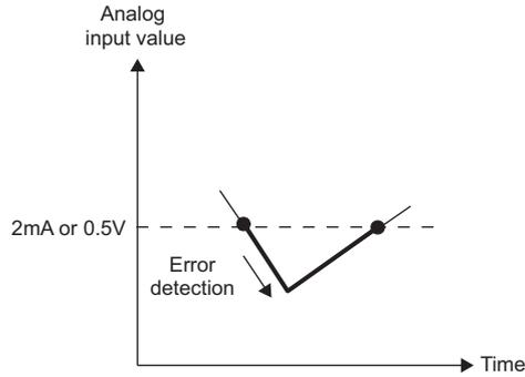
The setting in CH□ Input signal error detection setting value (Un\G412 to Un\G415) is ignored.
