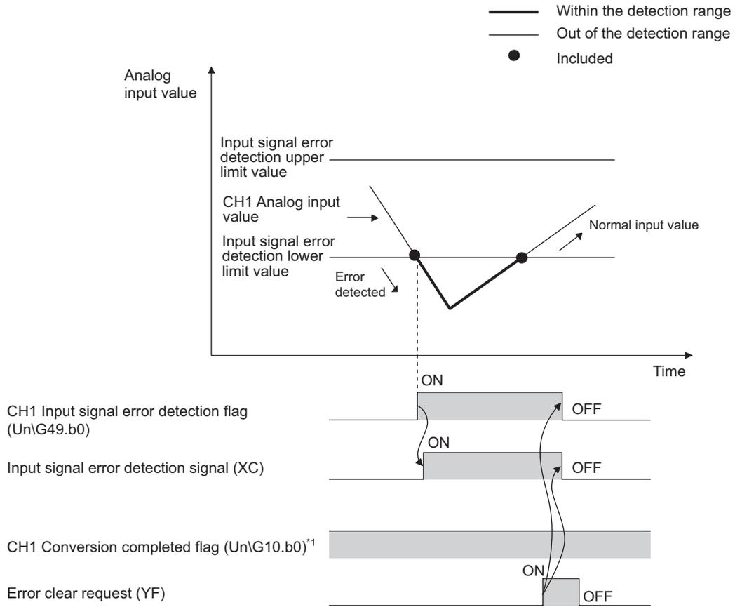
\*1 This flag does not turn off if a input signal error is detected.
