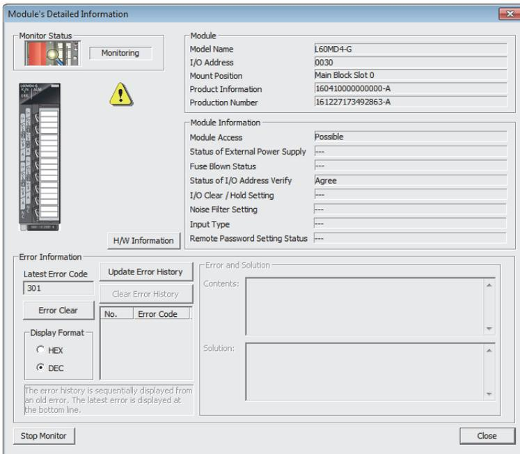
2. "Module's Detailed Information" of the multiple input module is displayed.
