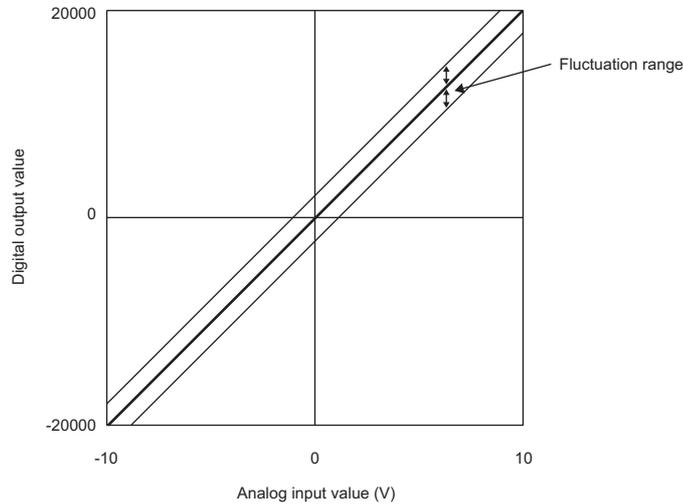
The fluctuation range differs depending on the ambient temperature and the input range as described in the following table.
