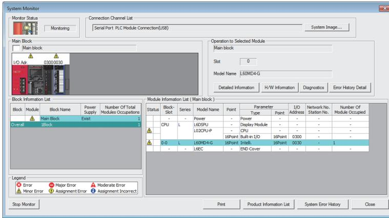
1. Select the multiple input module in "Main Block" and click the **Detailed Information** button.
