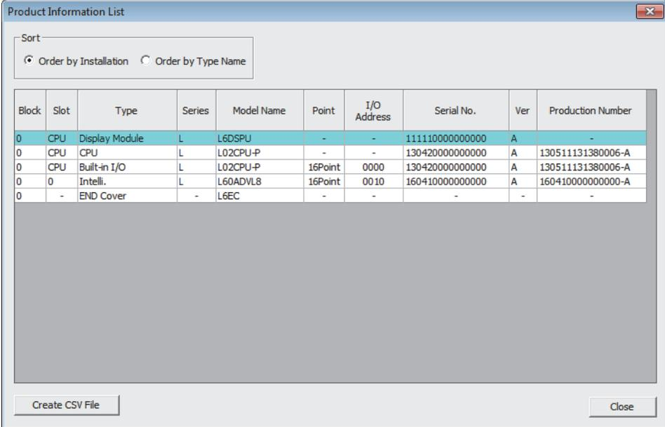
The screenshot shows a window titled "Product Information List" with a table of hardware components. The table has columns for Block, Slot, Type, Series, Model Name, Point, I/O Address, Serial No., Ver, and Production Number. The first row is highlighted in blue.
