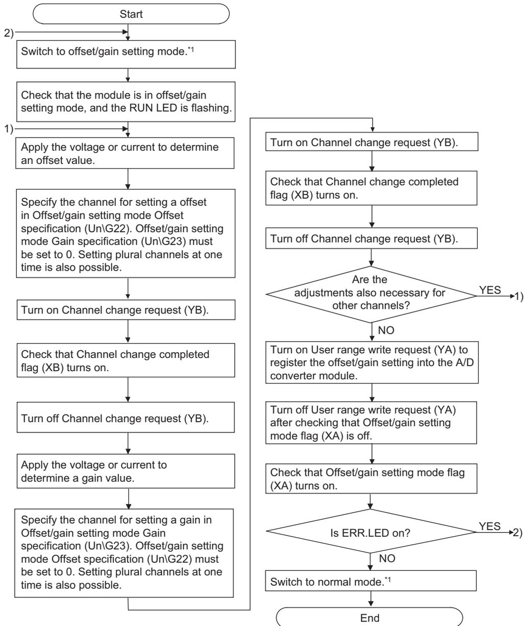
\*1 The following shows the procedure for switching the mode (normal mode → offset/gain setting mode or offset/gain setting mode → normal mode).
