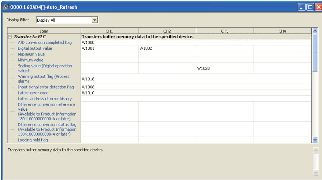
**7. Write the set parameter to the head module and reset the head module, or turn off and then on the programmable controller power supply.**
