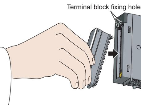
**1.** Fully insert the projections on the top of the terminal block into the terminal block fixing holes and press the terminal block until it snaps into place.
