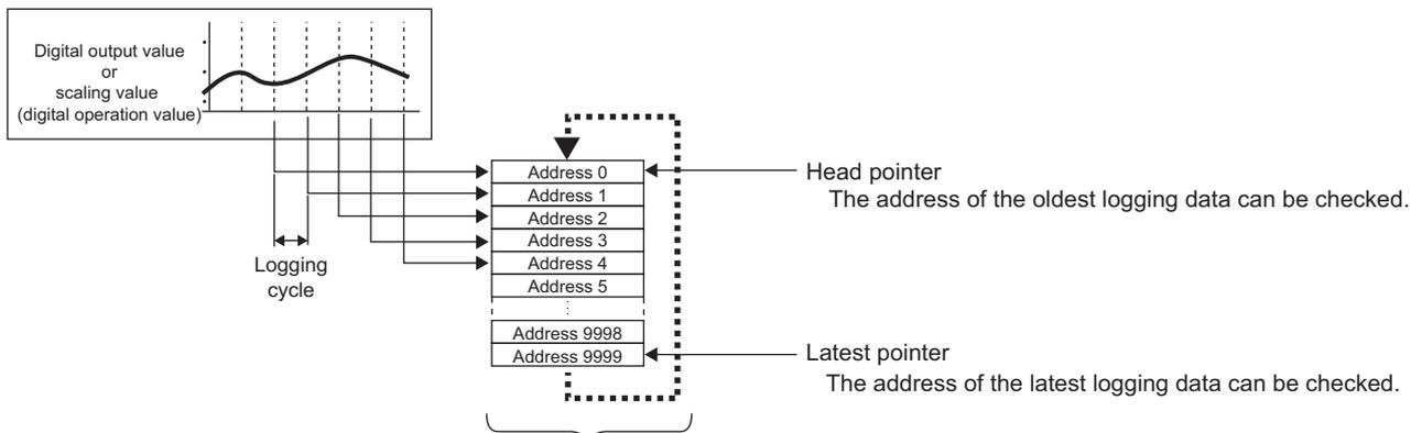
Logging data are stored in buffer memory areas. After the storage number has reached the maximum (10000 points), the stored data is overwritten with the subsequent data in order from the Address 0 area.
