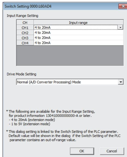
5. Display the initial setting screen for the A/D converter module (L60AD4) and configure the setting as follows.
