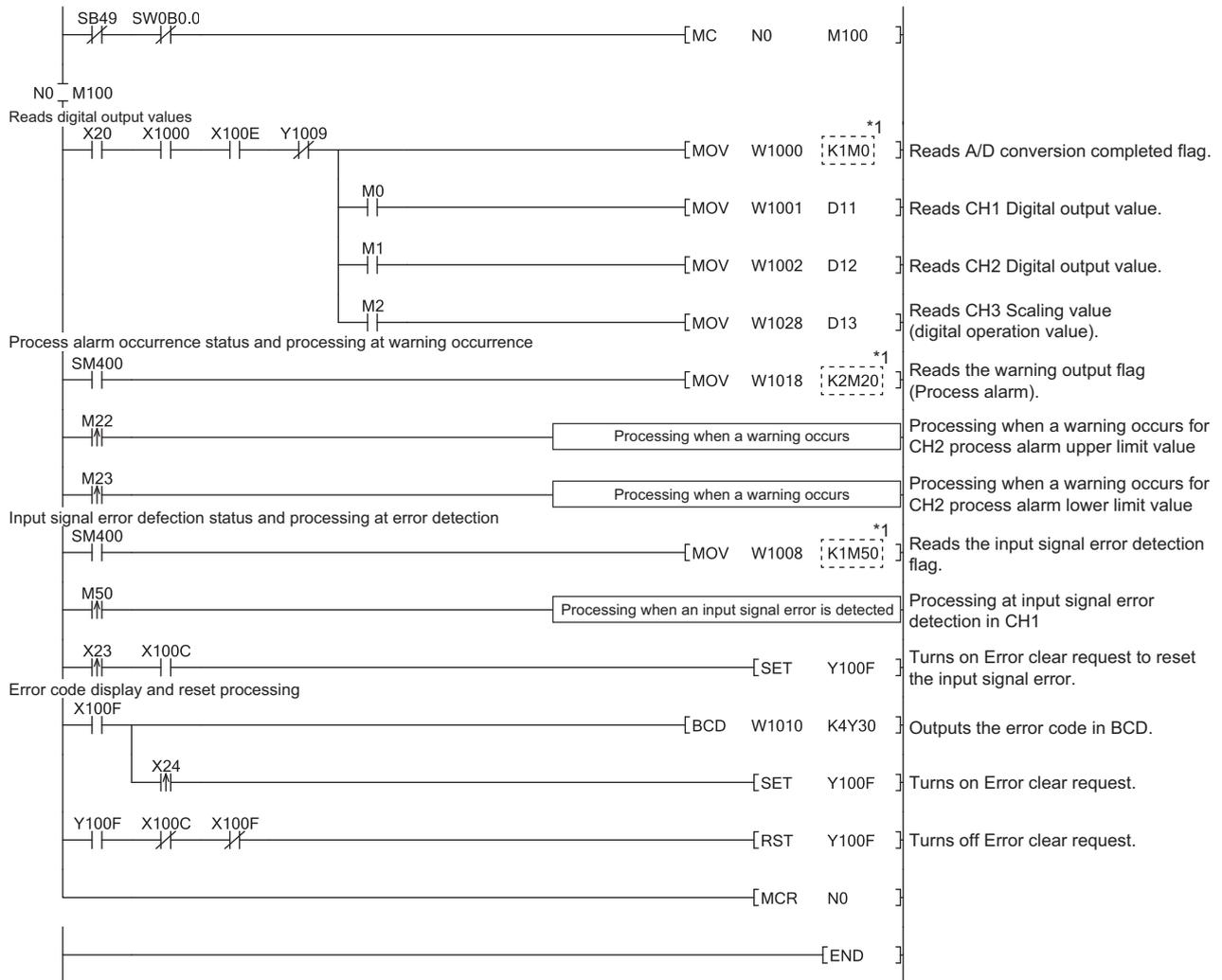
\*1 When using the L60ADVL8 or L60ADIL8 and enabling A/D conversion for five channels or more, increase the number of digits to be specified. (For example, change K1M0 to K2M0.)
