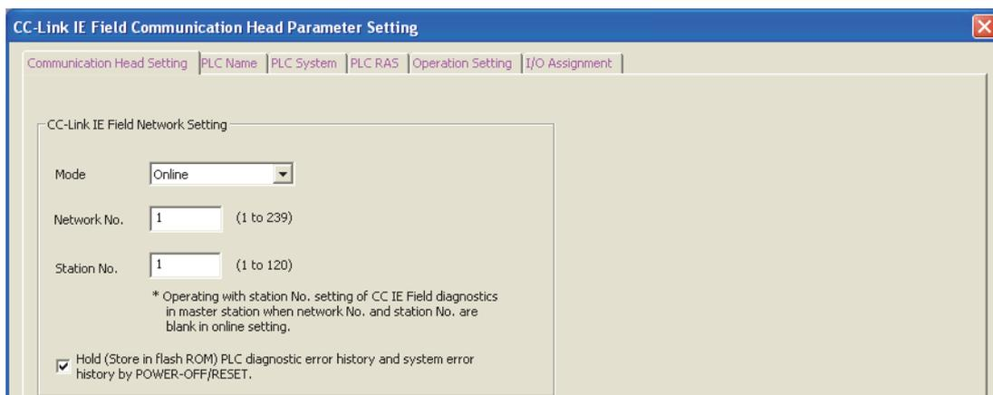
The "CC-Link IE Field Communication Head Parameter Setting" dialog box is shown with the following settings:
