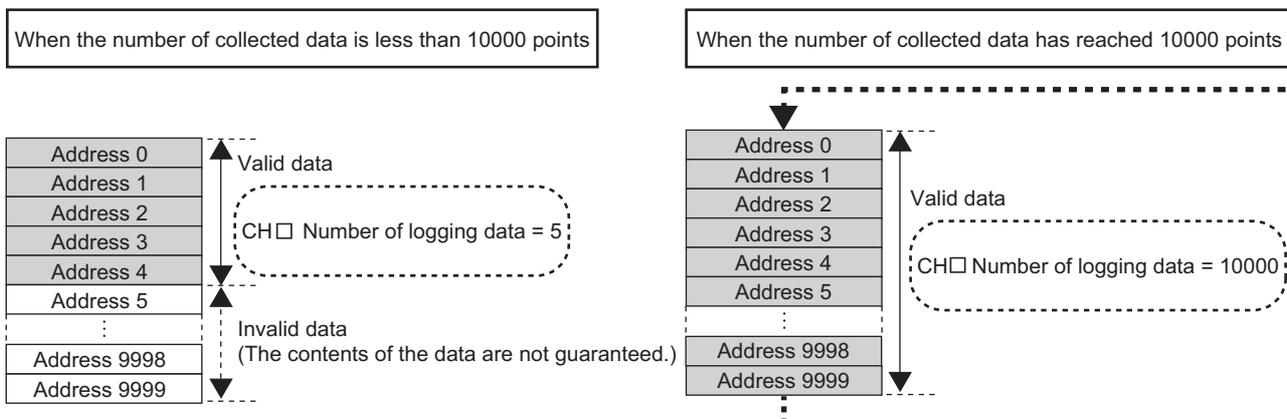
The number of logging data increases one by one each time new data is stored. When CH□ Logging data (Un\G5000 to Un\G44999) becomes full (Number of logging data = 10000), the next data is stored in the first address of CH□ Logging data (Un\G5000 to Un\G44999), and the logging operation continues overwriting the existing data. The number of logging data is fixed to 10000.
