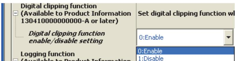
In this case, scale conversion is performed on the digital-clipped digital output value. Therefore, the digital output range of the scaling value (digital operation value) is determined as 0 to 32000.
