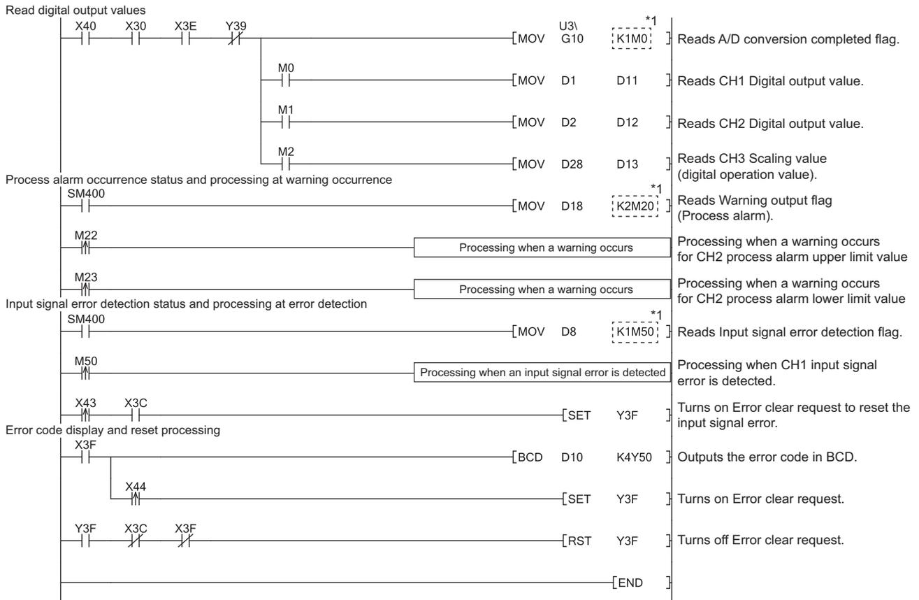
\*1 When using the L60ADVL8 or L60ADIL8 and enabling A/D conversion for five channels or more, increase the number of digits to be specified. (For example, change K1M0 to K2M0.)
