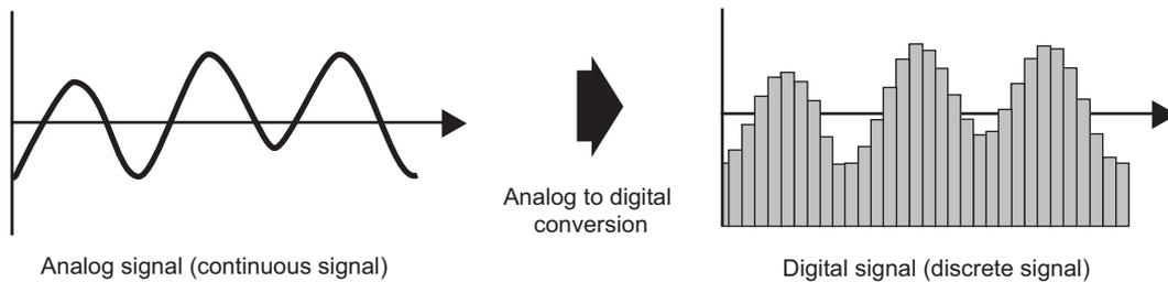
The A/D converter module enables works as follows.
