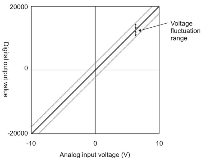
The fluctuation range varies depending on the ambient temperature and input range as shown below.
