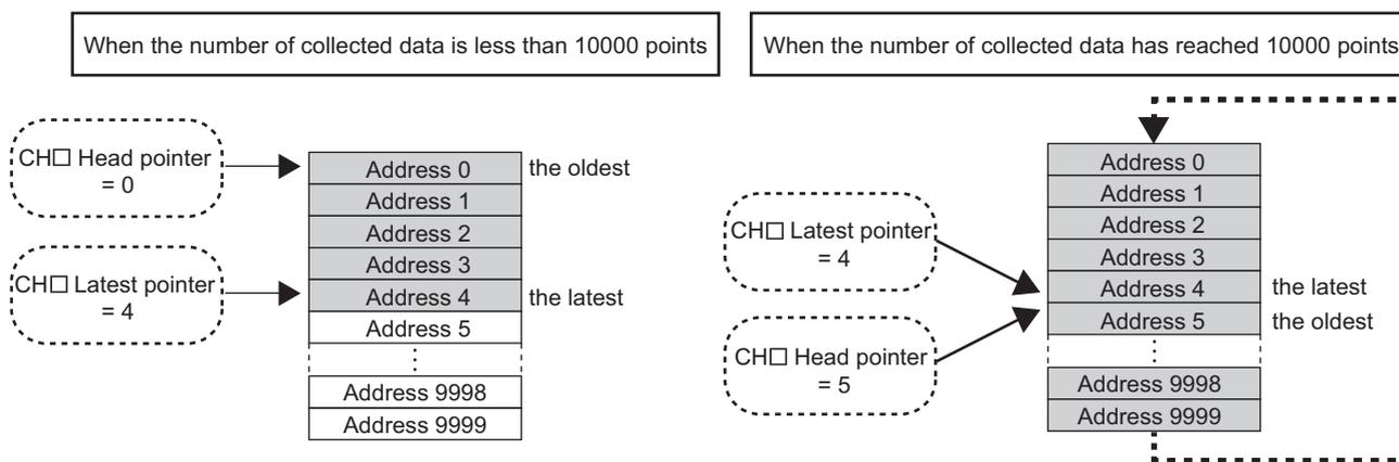
The head pointer does not change until CH□ Logging data (Un\G5000 to Un\G44999) becomes full after the logging start (The value is fixed to 0). The head pointer moves by one point when CH□ Logging data (Un\G5000 to Un\G44999) becomes full and the overwriting of data starts from the first address.
