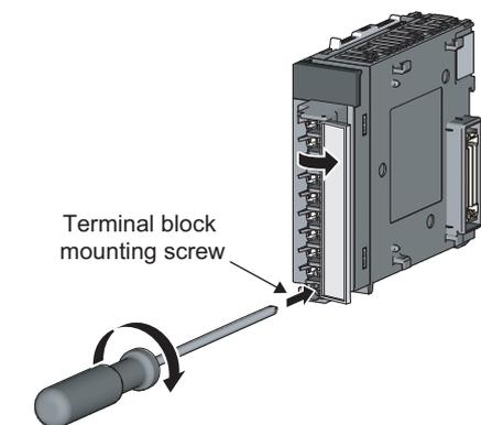
**2.** Open the terminal cover and tighten the terminal block mounting screw.
