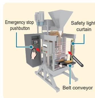
**8** Checking operation of the safety control circuits
