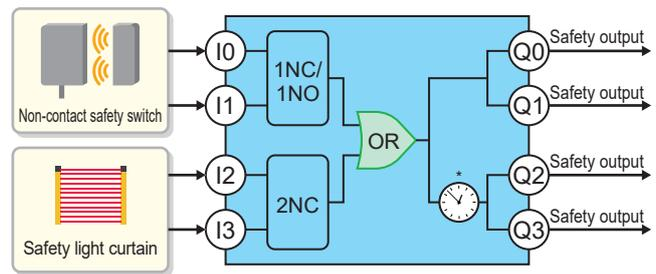
\*: This is an off delay time. The factory default setting of the rotary switch is 0 second.
