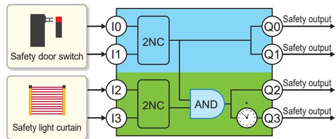
\*: This is an off delay time. The factory default setting of the rotary switch is 0 second.
