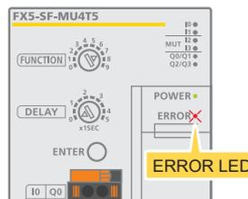
\*: An error will occur if the wiring of the terminals X0, X1, and X2 is changed after the settings are applied.
