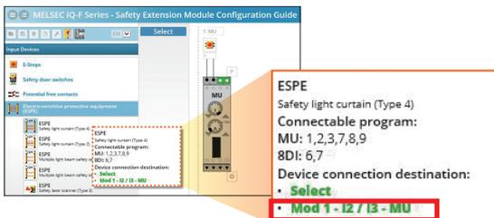
4 The connection configuration of the emergency stop pushbutton and safety light curtain to the safety main module is displayed.
