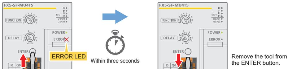
\*: Remove the tool from the ENTER button within three seconds after the ERROR LED starts flashing. Holding down the ENTER button for longer than three seconds causes an error of the entire safety main module.
