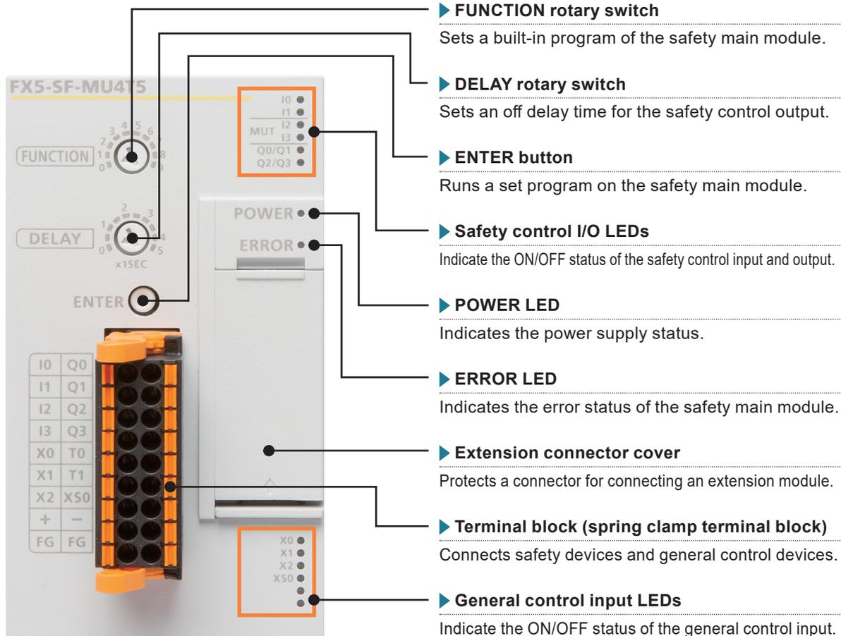
5 SAFETY MAIN MODULE WIRING
