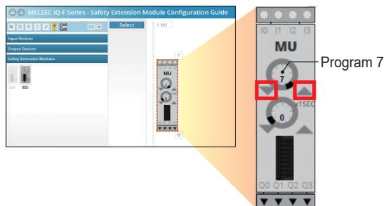
To display a logic circuit of the program 7, click
