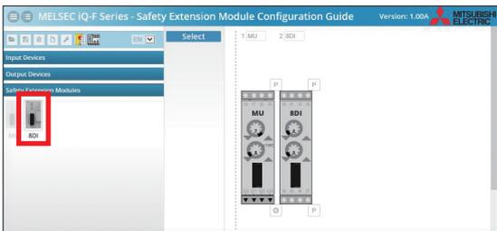
**3** Two safety input expansion modules (8DI) are added to the safety main module (MU).
