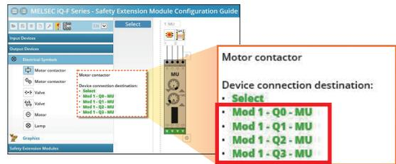
5 The connection configuration of the emergency stop pushbutton, safety light curtain, and safety contactors to the safety main module is displayed.
