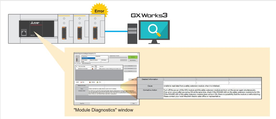
Information such as safety device settings and input/output status can be checked in the buffer memory, reducing the recovery time.
