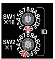
[Station number 1] Turn the rotary switches to set as shown on the left side. (01h)
