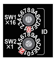
[Station number 2] Turn the rotary switches to set as shown on the left side. (02h)
