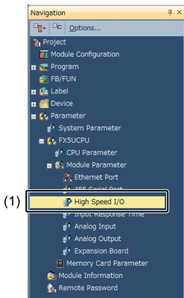
(1) Double-click [Parameter] → [FX5UCPU] → [Module Parameter] → [High Speed I/O] on the navigation window.
