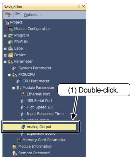
(1) Double-click [Parameter] → [FX5UCPU] → [Module Parameters] → [Analog output] on the navigation window.
