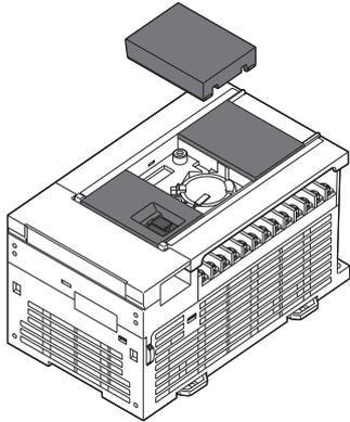
The PLC does not contain any consumable parts that could cause a short-term life. When using the optional battery, it is recommended to replace it periodically with the procedures given in the instruction manual. For the output relay, caution must be paid to the life when the relay operates at an abnormally high frequency or when switching a large capacity load.
