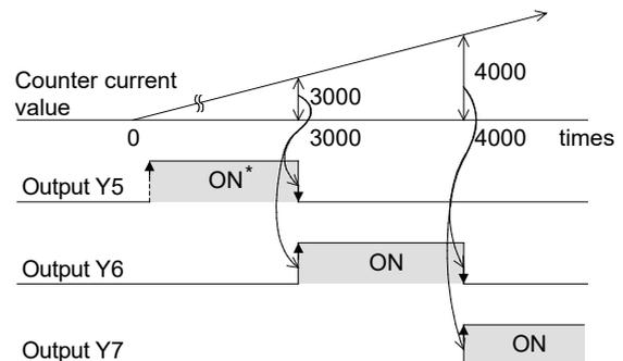
\* Y5 turns on when the counter counts up from 0 to 1.
