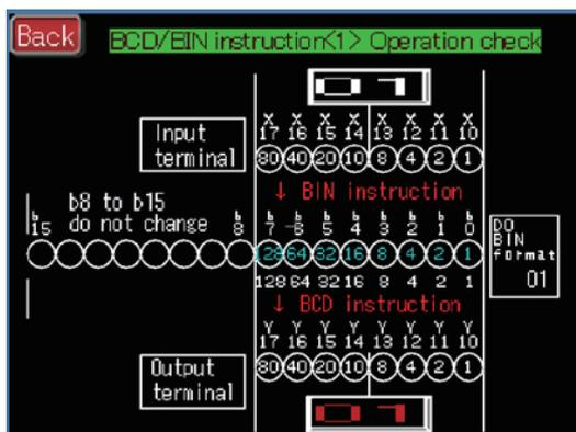
It is possible to check the bit operations of the input relays (X), output relays (Y), and data registers in the GOT screen monitor.
