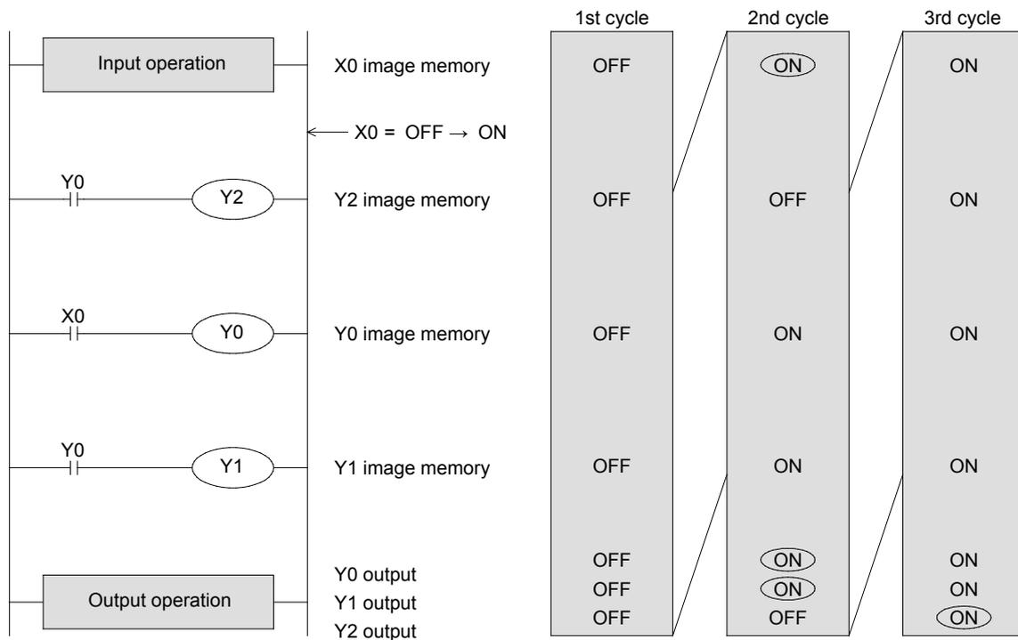
As shown above, Y0 and Y1 may have up to a 2-cycle response delay. (The output contact will be ON approximately 10 ms later.)
