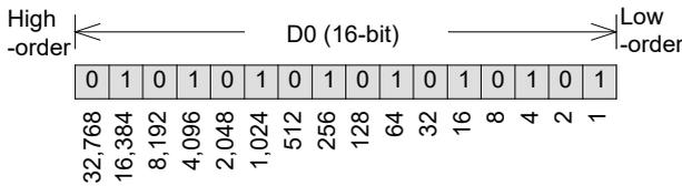
An unsigned 16-bit data register can represent numeric values from 0 to +65,535.
