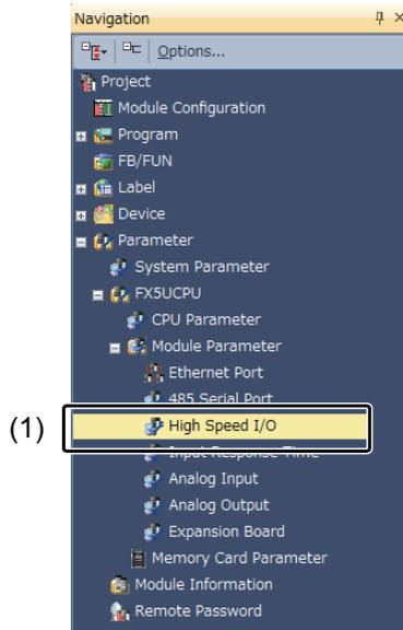
(1) Double-click [Parameter] → [FX5UCPU] → [Module Parameter] → [High speed I/O] on the navigation window.
