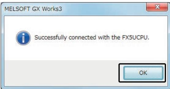
(9) Check that the CPU module is successfully connected, and click [OK].
