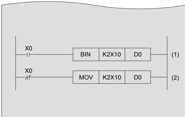
Transfer BIN-converted X10 to X17 ON/OFF (BCD value) to D0.
