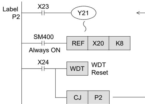
[Delay jump by one operation cycle]
