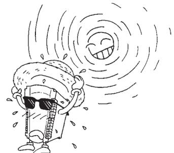
Do not install near a heating element, where the module could be subject to direct sunlight, dew condensation, rain or wind.
