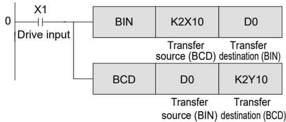
**BIN instruction.....** When the drive input is ON, the BCD value of the transfer source is converted to BIN and transferred.
