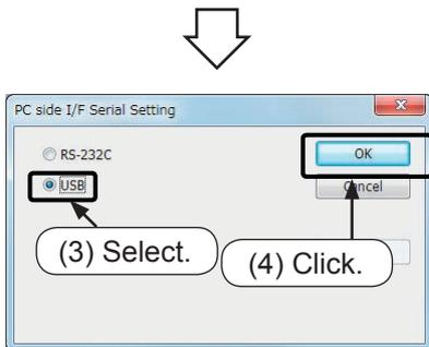
(3) Select the communication port on the PC side. (Select [USB] for the demonstration machine.)
