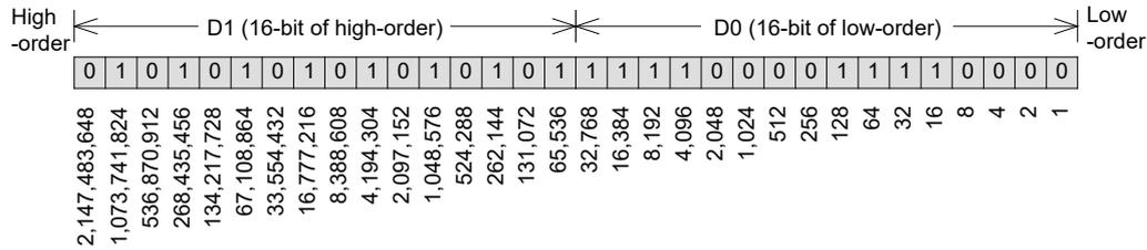
32-bit data is represented by a group of data registers with adjacent numbers. (The high-order bits are larger numbers and the low-order bits are small numbers.)
