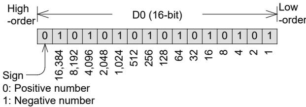
A signed 16-bit data register can represent numeric values from -32,768 to +32,767.
