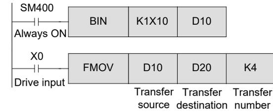
The data set by DSW1 is converted to BIN and then transferred to D10.
