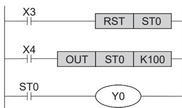
The timer ST0 starts timing at the moment X4 changes to ON. The timer keeps its current value if X4 is set to OFF or if the power is turned off during timing.
