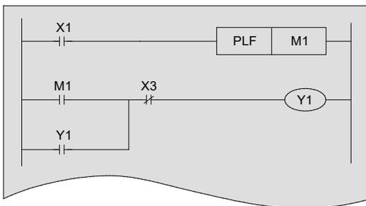
[When the falling edge pulse contact instruction is used]
