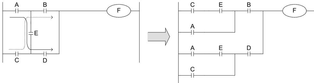
A circuit in which current flows in both directions must be rewritten as shown above. (The circuit when having no D, and the circuit when having no B, in parallel. It was connected.)
