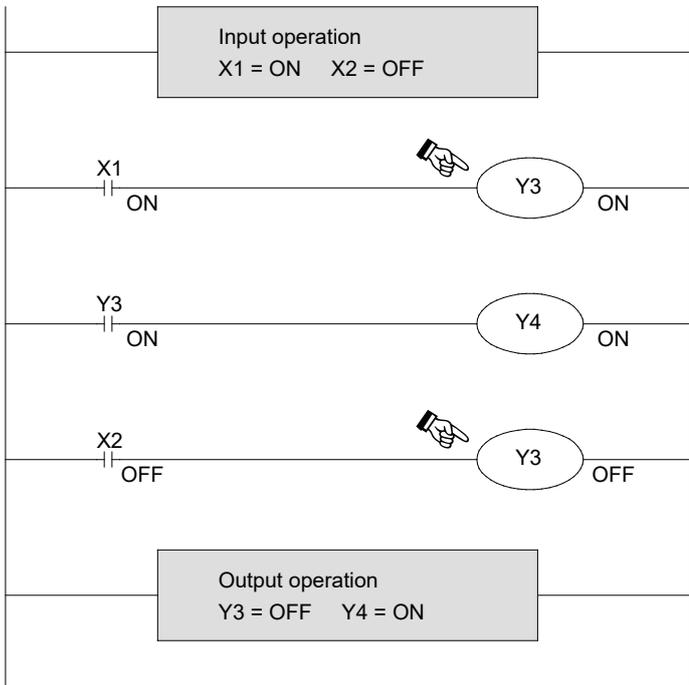
In this example, assume that coil Y3 is used in multiple locations.
