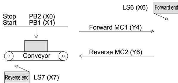
The following sequence circuit expresses the movement of a conveyor as shown on the left. The limit switch LS6 N.C. contact and the LS7 N.C. contact are de-energized at the conveyor's forward end and reverse end.
