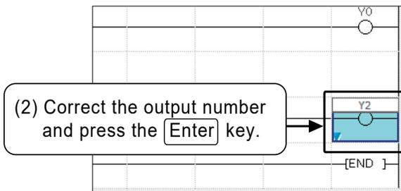
(2) The device can be modified. Modify the device to "Y2", and press the **[Enter]** key.
