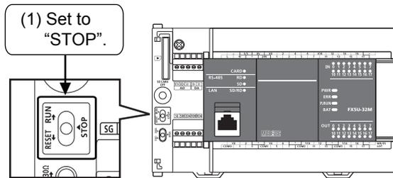
(1) Set the "RUN/STOP/RESET" switch of the CPU module to "STOP".
