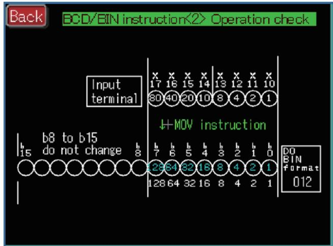
It is possible to check the bit operations of the input relays (X) and data registers (D0) in the GOT screen monitor.
