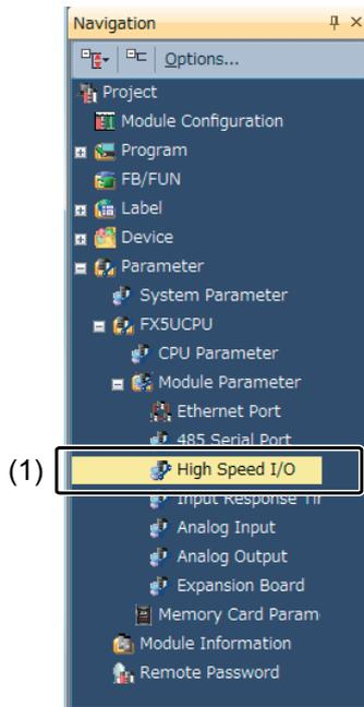
(1) Double-click [Parameter] → [FX5UCPU] → [Module Parameters] → [High Speed I/O] on the navigation window.
