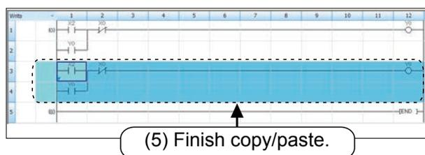
Continue to edit the circuit with the "cut" operation performed in the previous steps.
