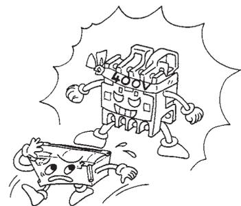
Separate the module as far away as possible from high-voltage wires, high-voltage devices and power devices.
