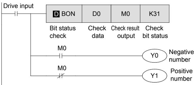
When the 31st bit (highest bit) of the 32-bit data D1 and D0 is ON, M0 is turned on.
