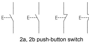
When a pushbutton switch has 2a, 2b contacts as shown on the left, the PLC needs one input for the 1a or 1b contact.
