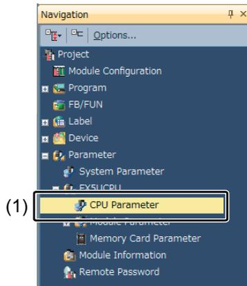
(1) Double-click [Parameter] → [FX5UCPU] → [CPU Parameter] on the navigation window.
