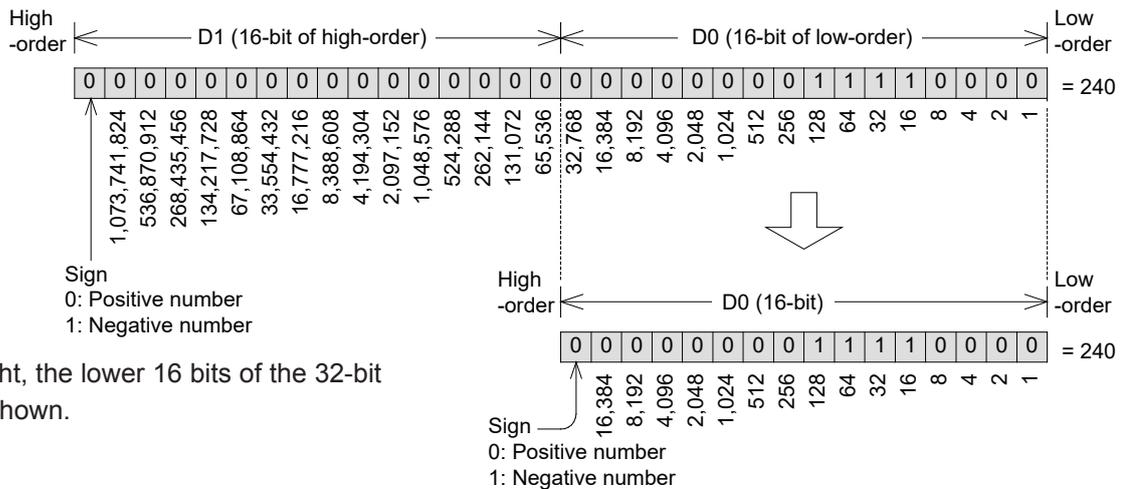
On the right, the lower 16 bits of the 32-bit data are shown.
