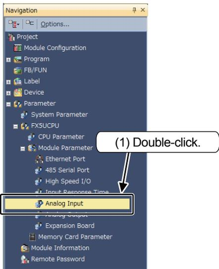
(1) Double-click [Parameter] → [FX5UCPU] → [Module Parameter] → [Analog Input] on the navigation window.
