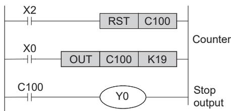
This counter counts the activation of the left limit switch shown above, and stops the table after counting 19 times.
