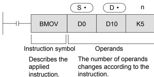
**S.** : The so-called source is the operand which does not change according to the execution of the instructions.
