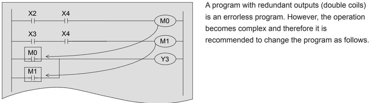
A program with redundant outputs (double coils) is an errorless program. However, the operation becomes complex and therefore it is recommended to change the program as follows.
