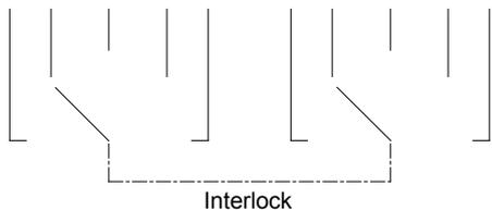
If there is one 2-step 5-notch select switch (rotary switch) as shown on the left, the PLC input will be 5 points.
