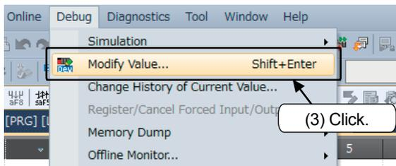
(3) The ON/OFF state will be highlighted when [Debug] → [Modify Value] are selected from the menu bar.
