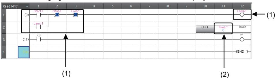
(1) The on/off states of contacts and coils are displayed.
