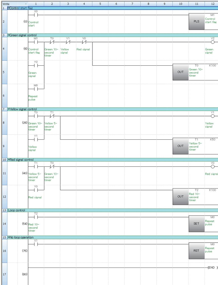
If X0 turns ON, M1 will turn ON for one scan cycle.
