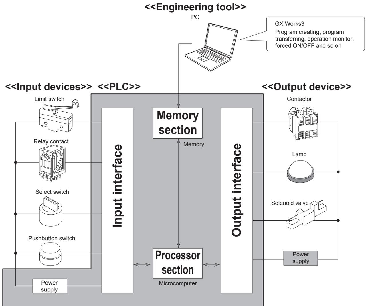
A PLC incorporates an electrical circuit mainly comprised of a microcomputer and memory. Input/output interfaces exist between input/output devices and the electronic circuit to connect them. The engineering tool is used to write a program to the memory in the PLC.
