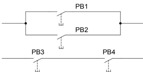
An input switch always connected in parallel or an input switch used as a serial connection can each be handled as one input.
