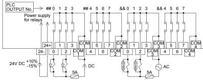
Terminal blocks are not equipped with built-in fuses. In order to prevent breakdown of circuits caused by load short-circuit, provide a fuse of 5 to 10 A for every four points.
