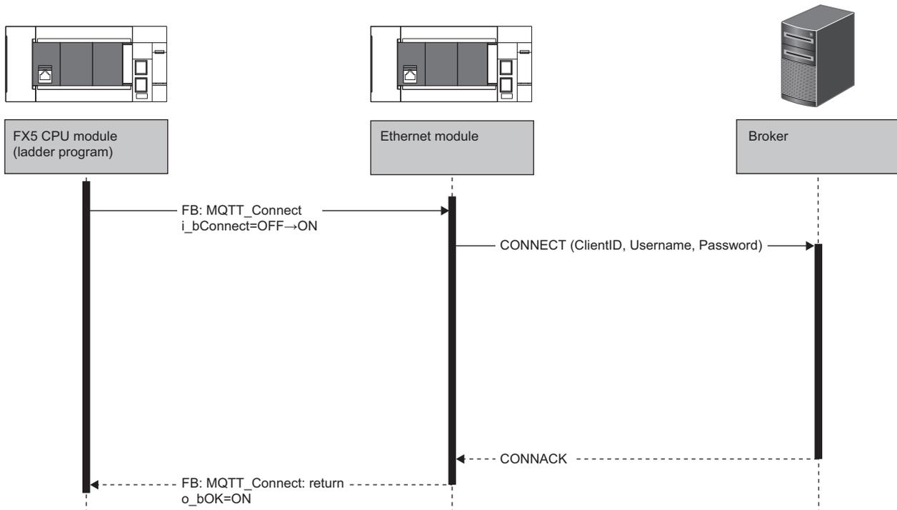
To connect to a broker, the MQTT client (Ethernet module) sends the CONNECT command to a broker.
