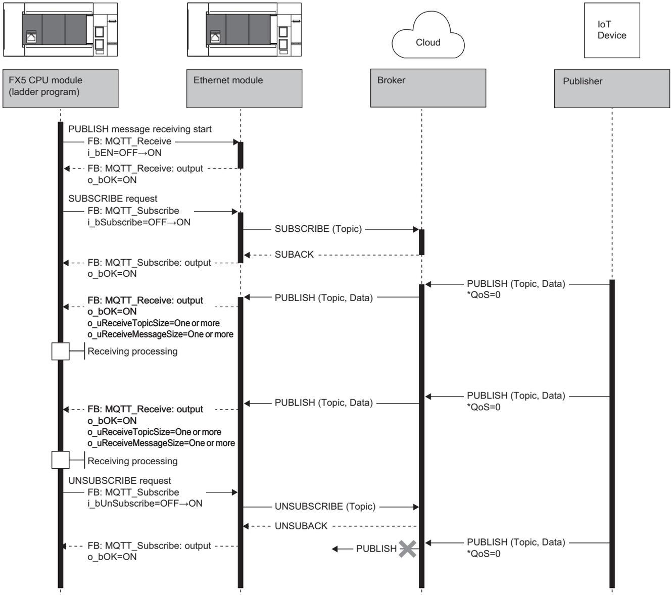
As a subscriber, the MQTT client uses `FB: MQTT_Subscribe` to send a broker the `SUBSCRIBE` command to request a topic to subscribe. The broker returns the `SUBACK` command to the subscriber. When the requested topic matches a topic in the `PUBLISH` command received from publishers, the broker uses the `PUBLISH` command to send the topic name and data to the subscriber.
