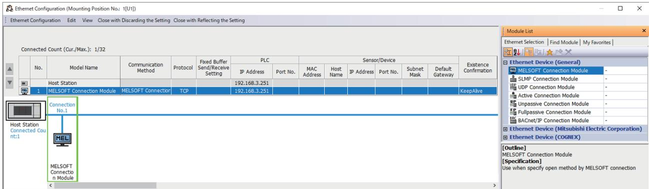
Drag and drop an "Ethernet Device" in the "Module List" to the left side of the screen, and set the following items. The setting items vary depending on the "Ethernet Device" and "Communication Method".
