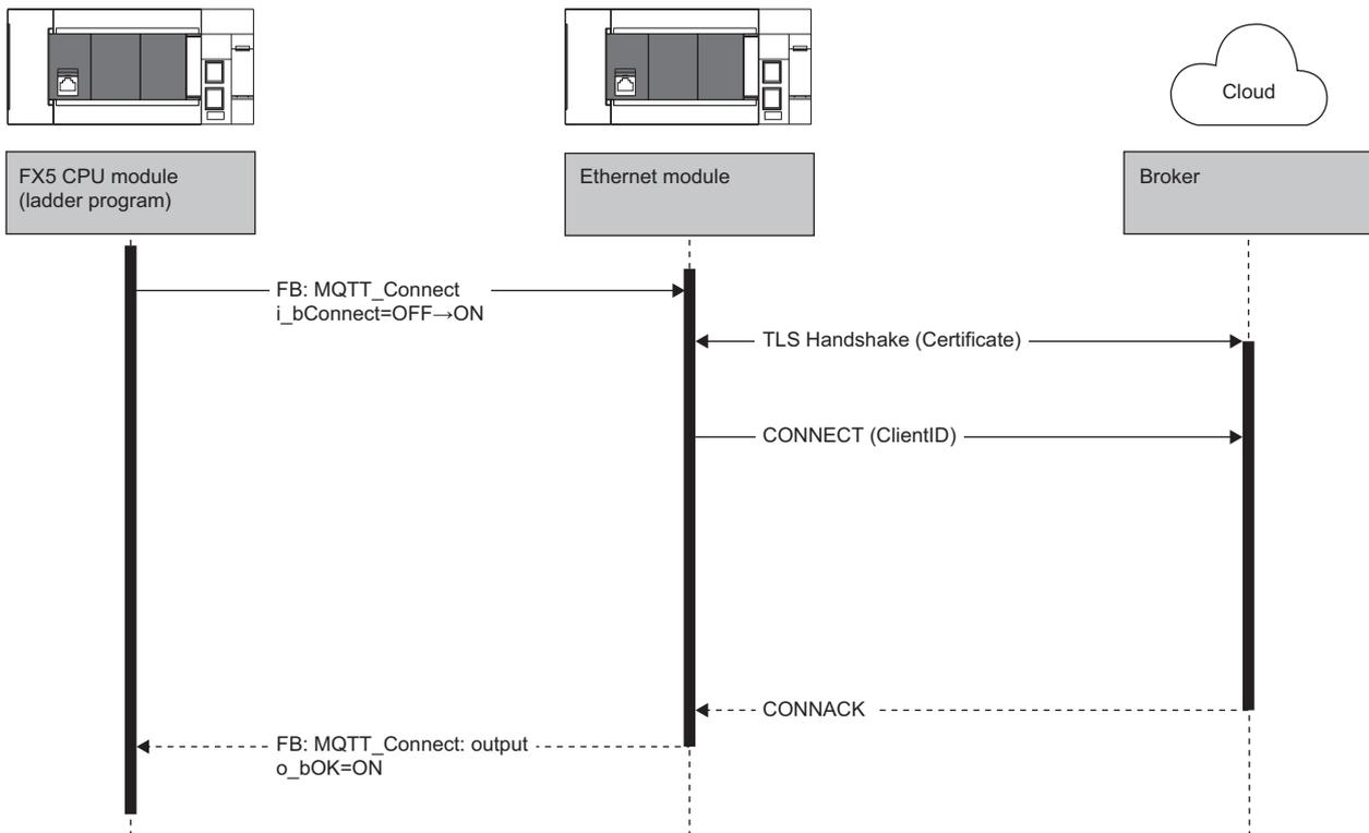
To use TLS connection, the MQTT client performs a TLS handshake before sending the CONNECT command. During the handshake, the client and broker exchange their certificates with each other. The client and broker must be configured in advance to trust each other's certificates.
