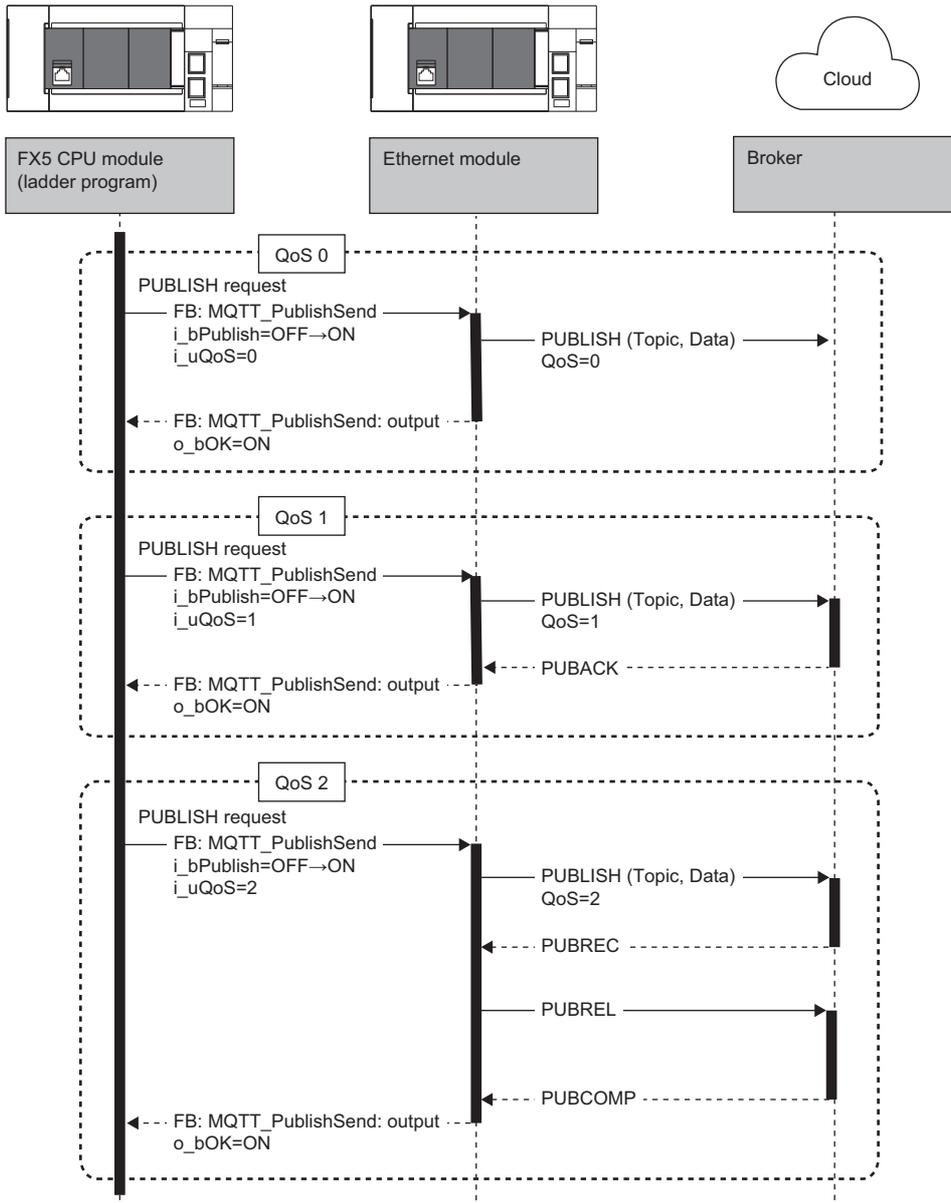
To send a message to a broker, the MQTT client (Ethernet module) sends the PUBLISH command to a broker.
