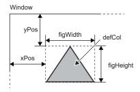
When a negative value is set for the figure height (figHeight), the downward triangle is displayed.
