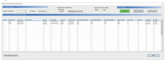
The module to be diagnosed can be switched with "Target Module Specification".
