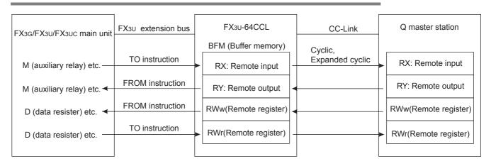
Data is transferred using FROM/TO instructions via the buffer memory (or direct specification of buffer memory) between the FX3G/FX3U/FX3UC PLC and the 64CCL. Data is replaced with internal devices (such as M, R and D), and used in sequence programs.
