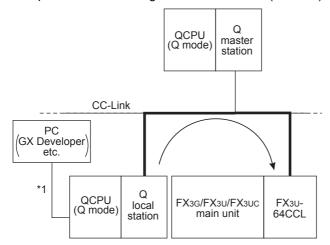
\*1. Direct connection or connection using the GOT transparent mode.
