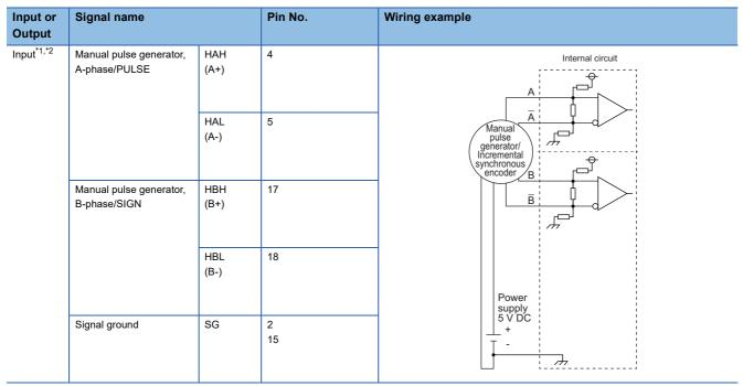
\*1 Set "0: Differential-output type" in "[Pr.89] Manual pulse generator/Incremental synchronous encoder input type selection" if the manual pulse generator/Incremental synchronous encoder of differential-output type is used. The default value is "1: Voltage-output/open-collector type".
