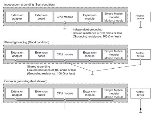
• Keep the distance between the grounding point and the programmable controller as close as possible to shorten the length of ground cable.
