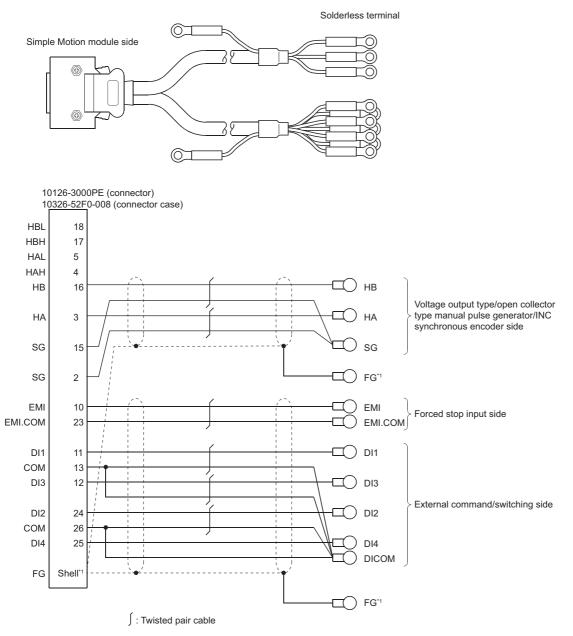
\*1 Make sure to perform shield treatment on the used equipment side. Also, connect it to the shell of connector side.
