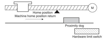
• When the zero signal is detected again during deceleration (4.) in the following figure) with detection of zero signal, the operation stops at the zero signal detected lastly to complete the home position return.
