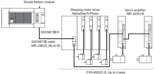
FX5-40SSC-S: Up to 4 axes FX5-80SSC-S: Up to 8 axes
