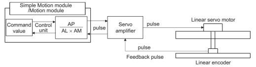
Calculate the number of pulses (AP) and movement amount (AL × AM) for the linear encoder in the following conditions.
