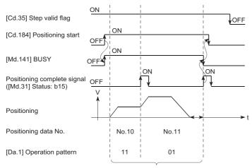
No positioning data No. unit, so operation pattern becomes one step of unit for carrying out automatic deceleration.
