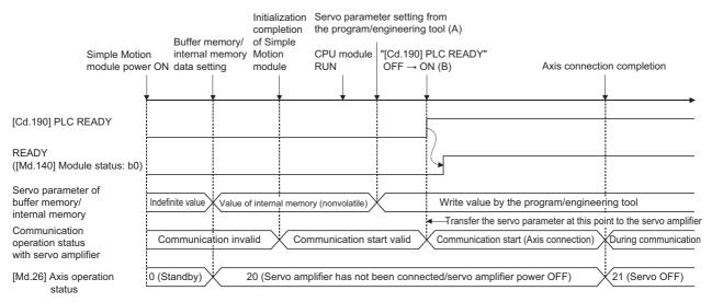
When the servo amplifier's power supply is turned ON after the "[Cd.190] PLC READY" is turned OFF to ON ((C) in the following figure)
