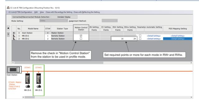
**2.** Set the PDO mapping pattern selection for the station to be used in other than the cyclic synchronous mode in Detail Setting of "PDO Mapping Setting".
