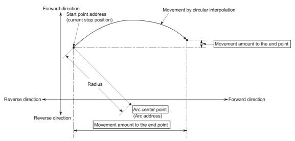
Positioning of a complete round with a radius of the distance from the start point address to the arc center point can be carried out by setting the movement amount to "0".
