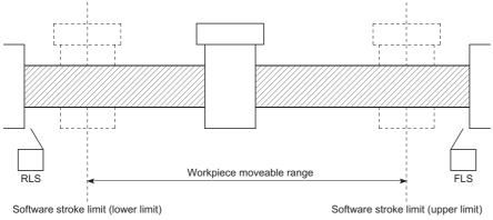
The following drawing shows the differences in the operation when "[Md.20] Command position value" and "[Md.21] Machine feed value" are used in the moveable range limit check.
