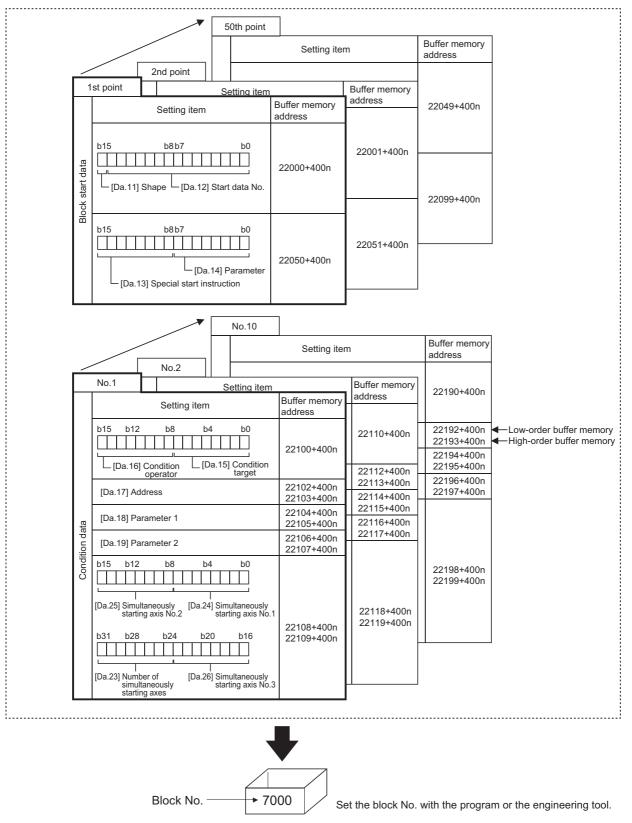
Set the "block start data" and "condition data" corresponding to the following "block No.7001" using the program or the engineering tool to Simple Motion module.
