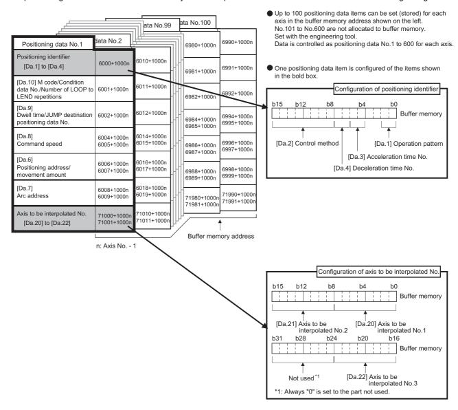
The following explains the positioning data setting items [Da.1] to [Da.10] and [Da.20] to [Da.22]. (The buffer memory addresses shown are those of the "positioning data No.1".)
