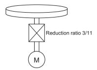
First, find how many degrees the load (machine) will travel ( $\Delta$ S) when the motor turns one revolution (AP).
