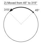
To designate the positioning direction (not carrying out the shortcut control), the shortcut control is invalidated and positioning in a designated direction is carried out by the "[Cd.40] ABS direction in degrees".
