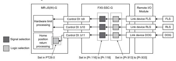
Set the following values for the signal logic selection of the servo amplifier.
