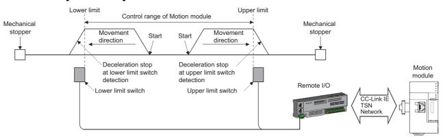
Set the servo parameters and the link device external signal assignment parameters appropriately. For details, refer to the following.
