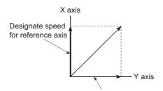
Calculated by Simple Motion module
