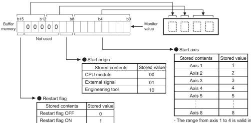
• The range from axis 1 to 4 is valid in the 4-axis module and from axis 1 to 8 is valid in the 8-axis module.
