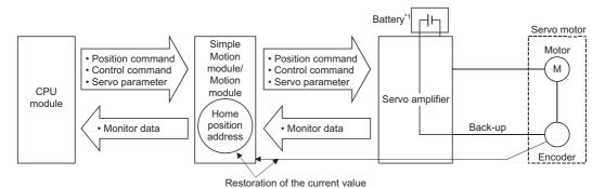
\*1 Depending on the servo amplifier used, it may be necessary to install a battery for retaining the location of the home position return in the servo amplifier.
