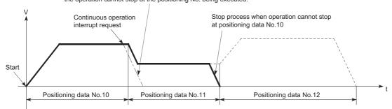
• When operation is not performed (BUSY signal is OFF), the interrupt request during continuous operation is not accepted. It is cleared to 0 at a start or restart.
