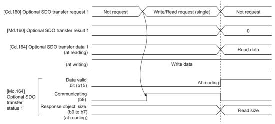
· Send/receive timing for individual read/write (when an error occurs)
