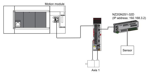
In this example, the signal used as the upper limit signal (FLS) is assigned to RX0 and the signal used as the lower limit signal (RLS) is assigned to RX1.
