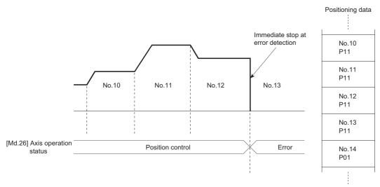
• During simultaneous start, a stroke limit check is carried out for the current values of every axis to be started. Every axis will not start if an error occurs, even if it only occurs in one axis.
