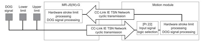
· When not using the external input signal of the servo amplifier
