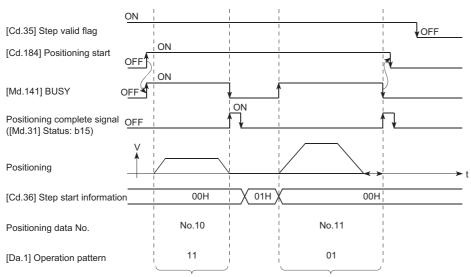
Operation pattern becomes one step of positioning data No. unit, regardless of continuous path control (11).
