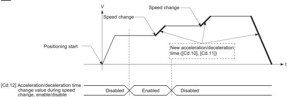
• If the "new acceleration/deceleration time" is set to "0" and the speed is changed after the "new acceleration/deceleration time" is validated, the operation will be controlled with the previous "new acceleration/deceleration time".
