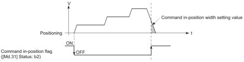
· A command in-position width check is carried out every operation cycle.
