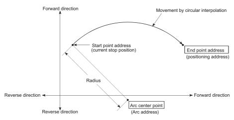
Positioning of a complete round with a radius from the start point address to the arc center point can be carried out by setting the end point address (positioning address) to the same address as the start point address.
