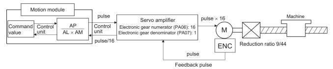
First, find how many millimeters the load (machine) will travel ( $\Delta S$ ) when the motor turns one revolution (AP).
