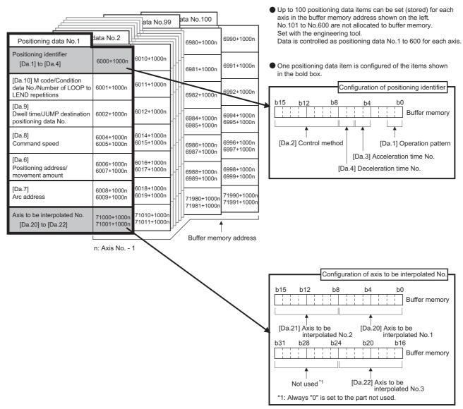
When setting positioning data using a program, determine buffer memory addresses using the following calculation formula and set the addresses.
