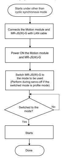
Change MR-J5(W)-G to the mode to be used by modifying link device that is assigned Modes of operation from program or watch.
