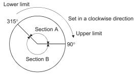
Set as follows to set the movement range of section A or B in the above figure.
