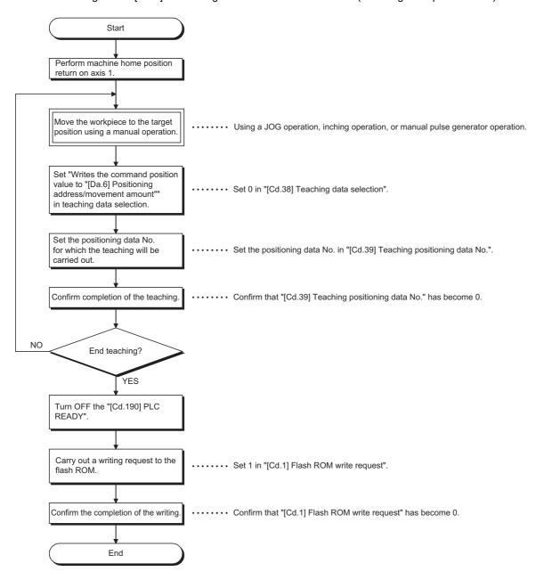
• When teaching to the "[Da.7] Arc address", then teaching to the "[Da.6] Positioning address/movement amount" (Teaching example for 2-axis circular interpolation control with sub point designation on axis 1 and axis 2)
