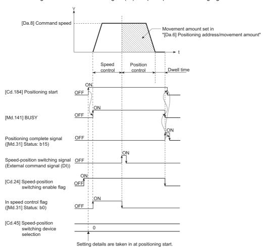
The following operation assumes that the speed-position switching signal is input at the position of the command position value of 90.00000 [degree] during execution of "[Da.2] Control method" "Forward run: speed/position" at "[Pr.1] Unit setting" of "2: degree" and "[Pr.21] Command position value during speed control" setting of "1: Update command position value". (The value set in "[Da.6] Positioning address/movement amount" is 270.00000 [degree])
