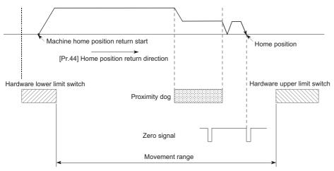
• When the direction from the workpiece to the home position is the opposite direction from the "[Pr.44] Home position return direction", the operation carries out a deceleration stop when the proximity dog turns OFF, and then carries out a machine home position return in the direction set in "[Pr.44] Home position return direction". The example shown below is for when "0: Positive direction" is set in "[Pr.44] Home position return direction".
