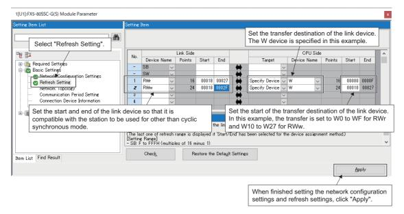
**4.** When performing control with other than the cyclic synchronous mode, perform operation with the supported link device for each object.
