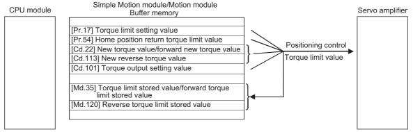
• The following table shows the storage details of "[Md.35] Torque limit stored value/forward torque limit stored value" and "[Md.120] Reverse torque limit stored value".
