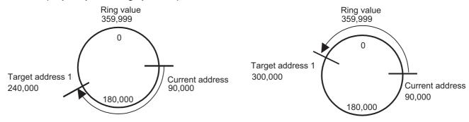
Example of rotation in the direction where the current value increases (BFM #530/#630: 1) (1-speed positioning operation)
