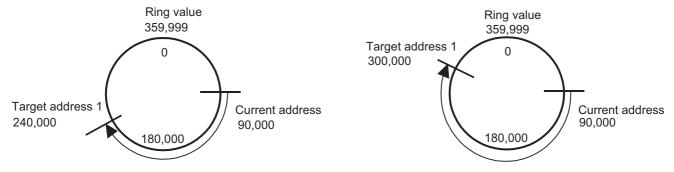
Example of rotation in the direction where the current value decreases (BFM #530/#630: 2) (1-speed positioning operation)
