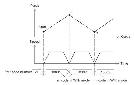
\*1. When setting the m code in With mode in a 20SSC-H earlier than Ver.1.30, the system waits for the m code OFF command, the m code OFF command is needed for the system operation to transition to the next table.
