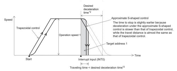
\*2. For the relation between the time for the actual deceleration and the specified time for desired deceleration, refer to the following.
