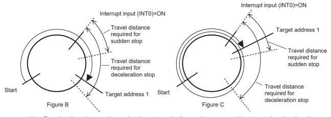
Deceleration time setting value is automatically set between sudden stop deceleration time and deceleration time.
