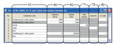
\*3. In 2-speed positioning operation and interrupt 2-speed constant quantity feed operation, two setting rows are required.
