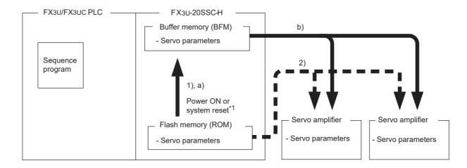
· How to transfer the servo parameters stored in the flash memory to the servo amplifier
