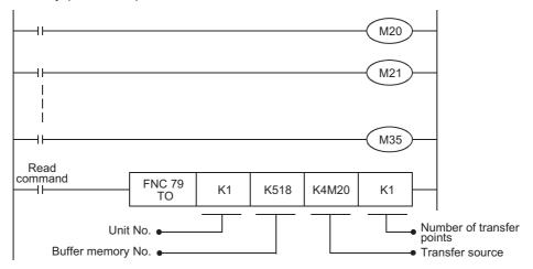
d) Writing bit information stored in data registers to the buffer memory In the program below, the ON/OFF status of each bit of a data register (D201) is written to the buffer memory (BFM #518) in unit No. 1. Each bit of the data register (D201) should be set to ON or OFF in advance by bit specification of word devices.
