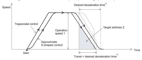
For the relation between the time for the actual deceleration and the specified time for desired deceleration, refer to the following.
