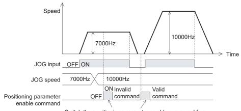
Switch the positioning parameter enable command from OFF to ON when the target axis is not performing positioning operation. If it is switched from OFF to ON while the target axis is performing positioning operation, the changed positioning parameter is invalid.
