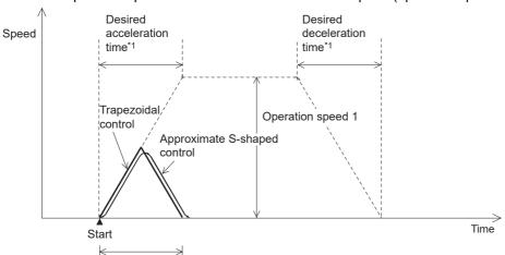
Traveling time < desired acceleration time\*1+ desired deceleration time\*1
