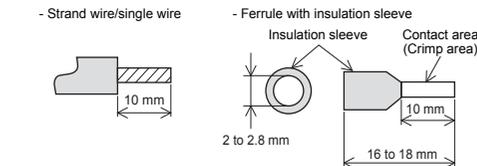
The following table shows wire ferrules and tools for wire ferrules compatible with the terminal block. Use of items other than these may result in not being able to remove the wire ferrule, so carefully check that the wire ferrule can be unplugged.
