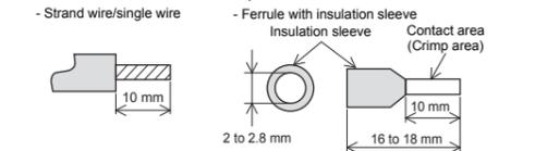
The following table shows wire ferrules and tools for wire ferrules compatible with the terminal block. Use of items other than these may result in not being able to remove the wire ferrule, so carefully check that the wire ferrule can be unplugged.
