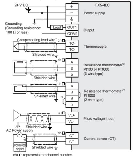
\*1 When using a thermocouple, use specified compensating lead wires.
