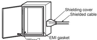
\*1 These wires are used to improve the conductivity between the door and control cabinet.
