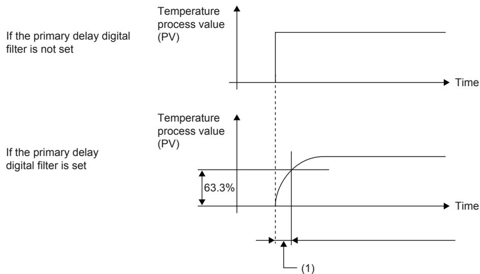
(1) 'CH1 Primary delay digital filter setting' (Un\G563)
