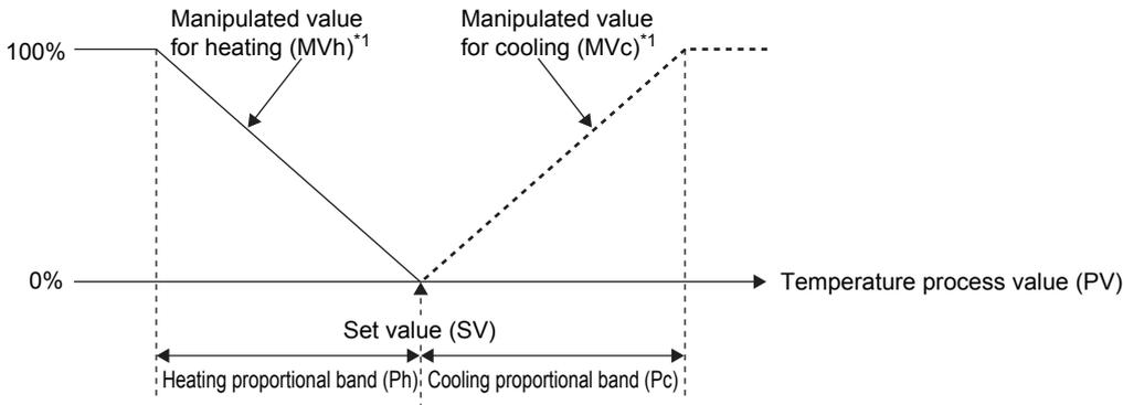
\*1 A value to be actually output is within the output limiter range set in "Upper limit output limiter" and "Lower limit output limiter" of "Limiter setting" in "Application Setting". (Page 78 Application Setting)
