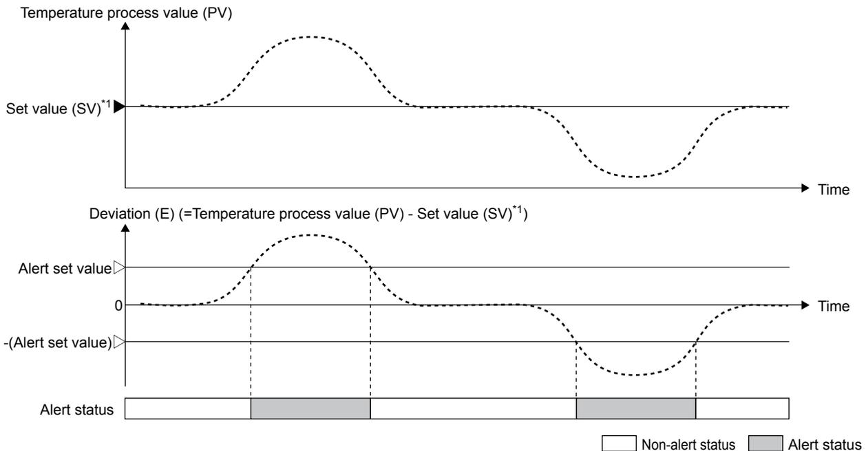
\*1 Depending on the alert mode setting, this value becomes the set value or the monitored value. The setting range of the alert set value is (-Full scale of the input range) to the full scale of the input range. (Page 54 Setting the set value (SV) and the setting change rate limiter)
