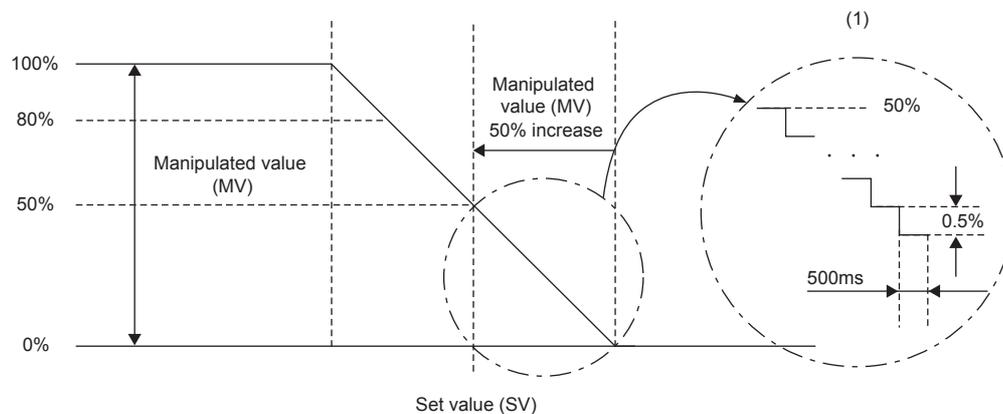
(1) When 'CH1 Output change ratio limiter' (Un\G510) has been set to 10 (1.0%/s)
