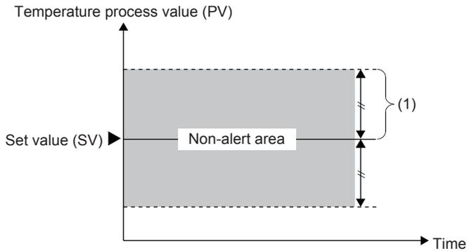
(1) 'CH1 Loop disconnection detection dead band' (Un\G538) (this band has the set value (SV) at the center)<sup>\*1</sup>
