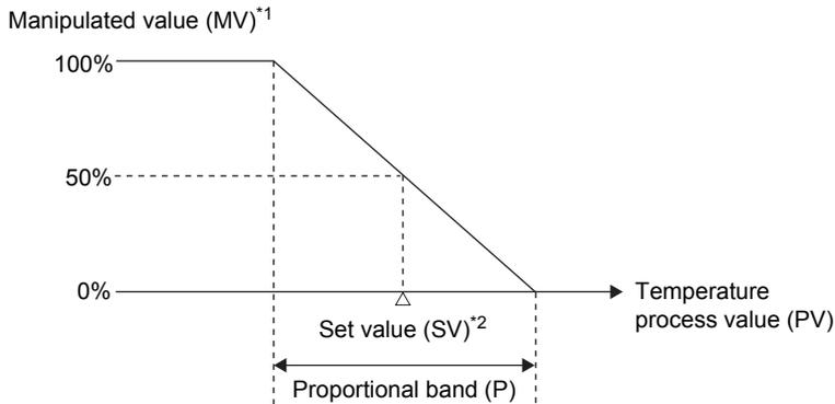
\*1 A value to be actually output is within the output limiter range set in "Upper limit output limiter" and "Lower limit output limiter" of "Limiter setting" in "Application Setting".
