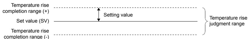
When the value set in 'CH1 Temperature process value (PV)' (UnG402) is within the temperature rise judgment range, 'CH1 Temperature rise judgment flag' (UnG404) is set to Within temperature rise completion range (ON). (For the time taken for 'CH1 Temperature rise judgment flag' (UnG404) to set to Within temperature rise completion range (ON) after the temperature rise completion, set the time in 'CH1 Temperature rise completion soak time setting' (UnG507).)
