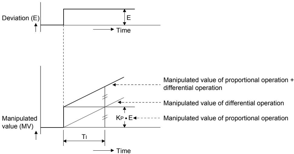
An integral action is used as a PI action in combination with a proportional action, or a PID action in combination with a proportional action and a derivative action. An integral action cannot be used by itself.
