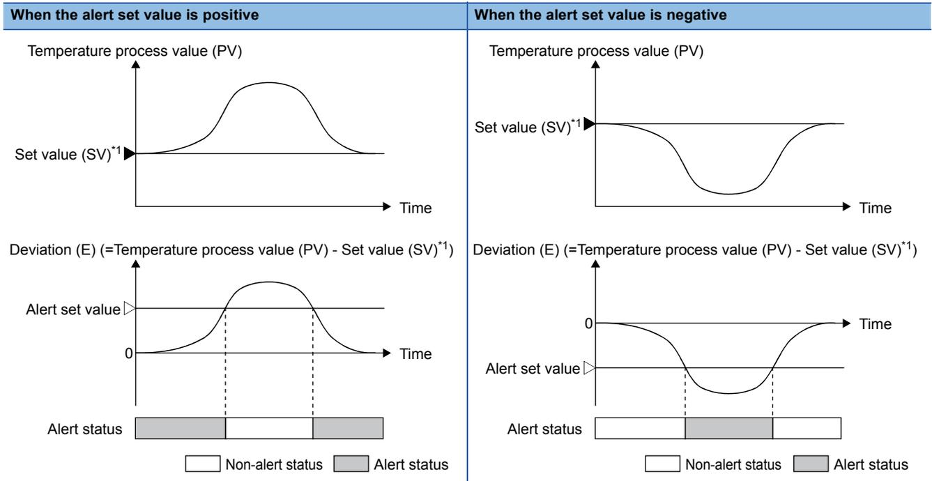
\*1 Depending on the set alert mode, this value becomes the set value or the monitored value. The setting range of the alert set value is (-Full scale of the input range) to the full scale of the input range. (Page 54 Setting the set value (SV) and the setting change rate limiter)
