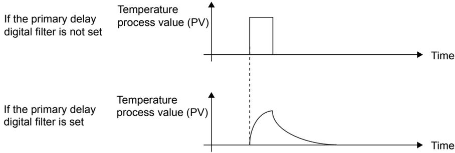
Set the time for the temperature process value (PV) to change by 63.3% in the primary delay digital filter.
