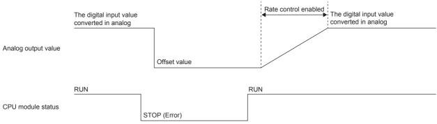
• When D/A conversion is enabled, D/A output is enabled, or the analog output HOLD setting is the previous value or set value if rate control is enabled, the analog output restarts from the offset value when the CPU module changes from STOP (error) to RUN.
