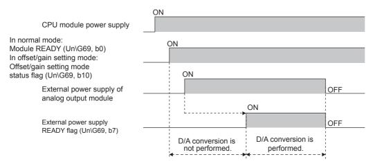
· When the external power supply is turned on and off
