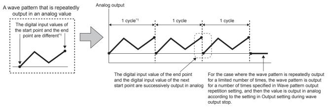
\*1 The wave pattern output cycle is calculated using the following formula.
