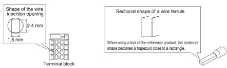
The following table shows wire ferrules and its associated tools compatible with the terminal block. The shape of the wire ferrule differs depending on the crimp tool to be used, use the reference product. If the product other than referenced products is used, the wire ferrule cannot be removed. Sufficiently confirm that the wire ferrule can be removed before use. <Reference product>
