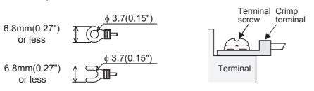
· When 2 wires are connected to 1 terminal: Use a crimp terminal of the size shown below, and install it as shown in the lower right figure.
