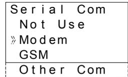
In the Top Menu, scroll down to the “Others/Serial Com/Modem” option and Press “OK”.
